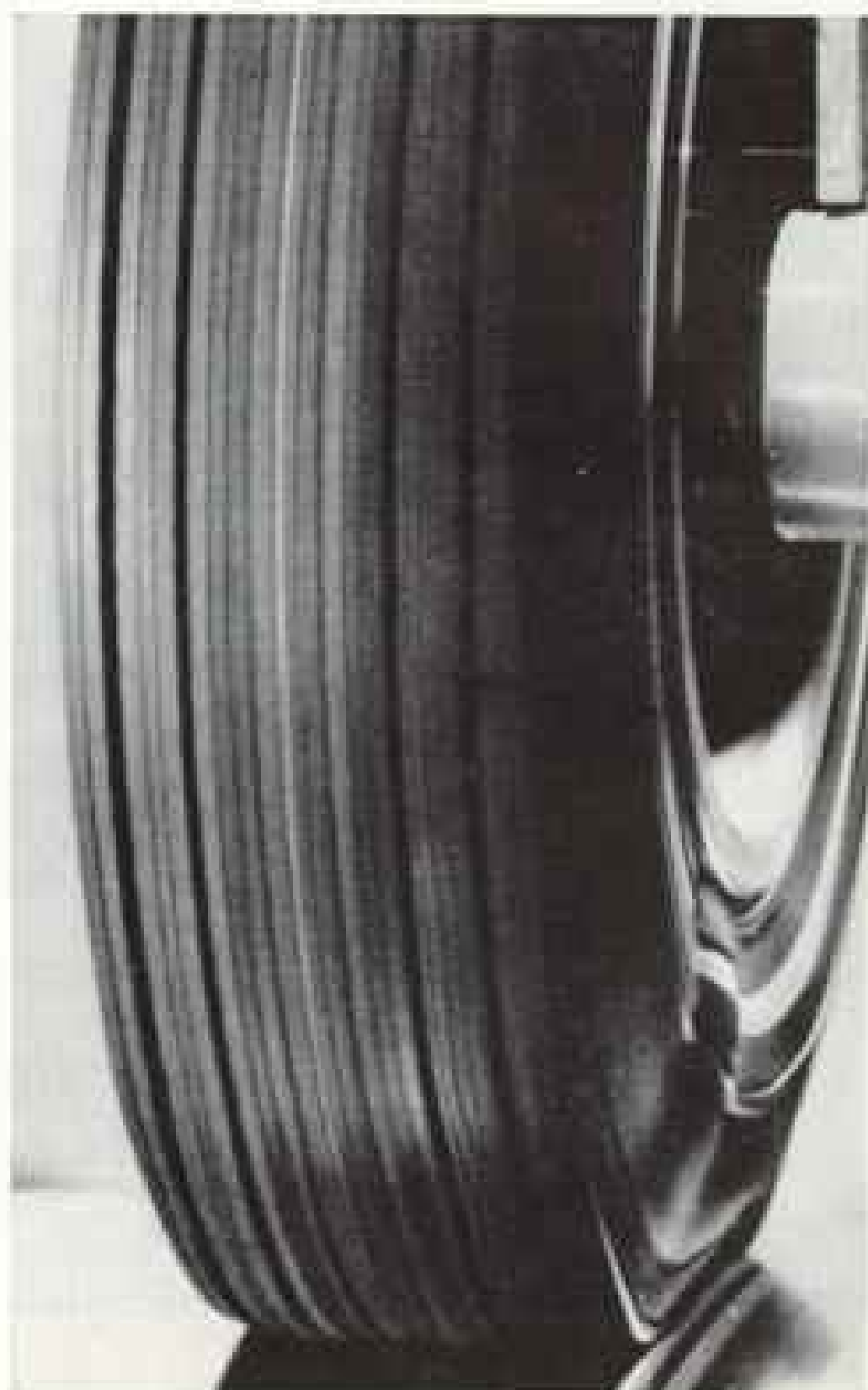
The Polyglas tire fights squirm. Look how this Polyglas tire stands up under the exact same speed and conditions as the two-ply tire. That's how much difference the fiberglass belts on the Polyglas tires can make in increasing mileage and improving traction.
