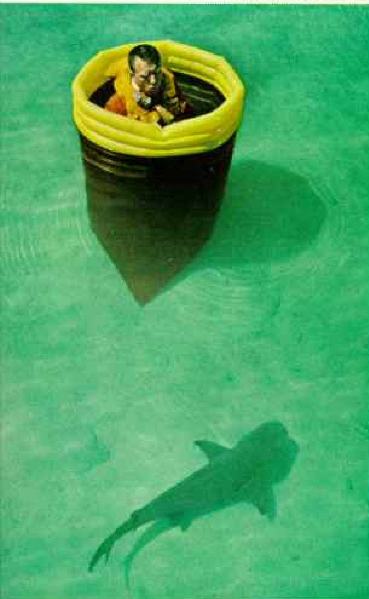
Cruising lemon shark at the Lerner Marine Laboratory on North Bimini Island circles Dr. C. Scott Johnson, testing a "survival sack" of his own design. Attached to a life jacket, the plastic bag can be quickly inflated.
