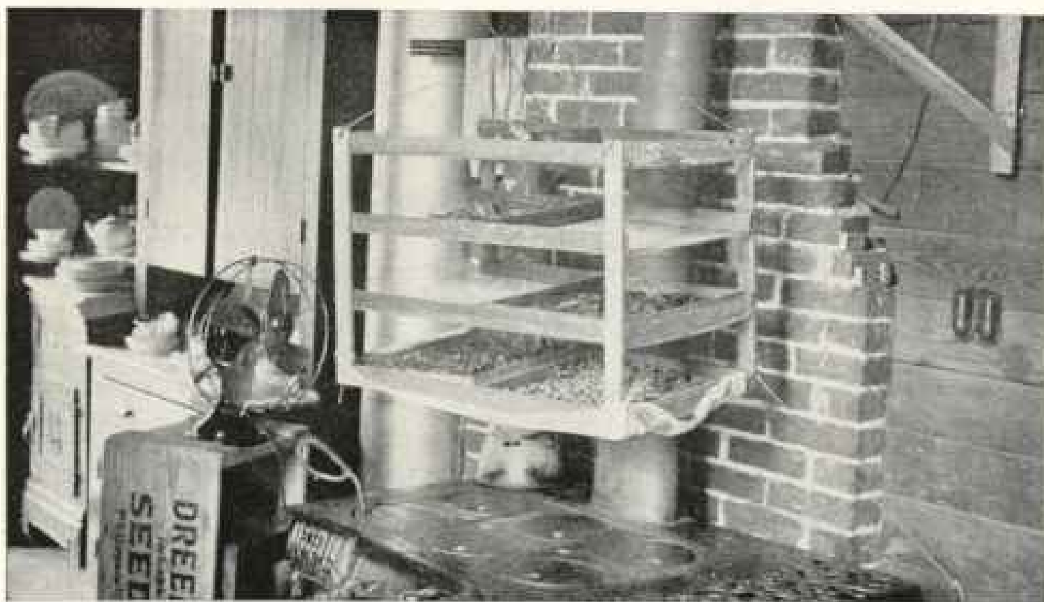
THE HANGING STOVE DRIER SWUNG OVER THE KITCHEN STOVE AFTER THE MEAL HAS BEEN PREPARED
