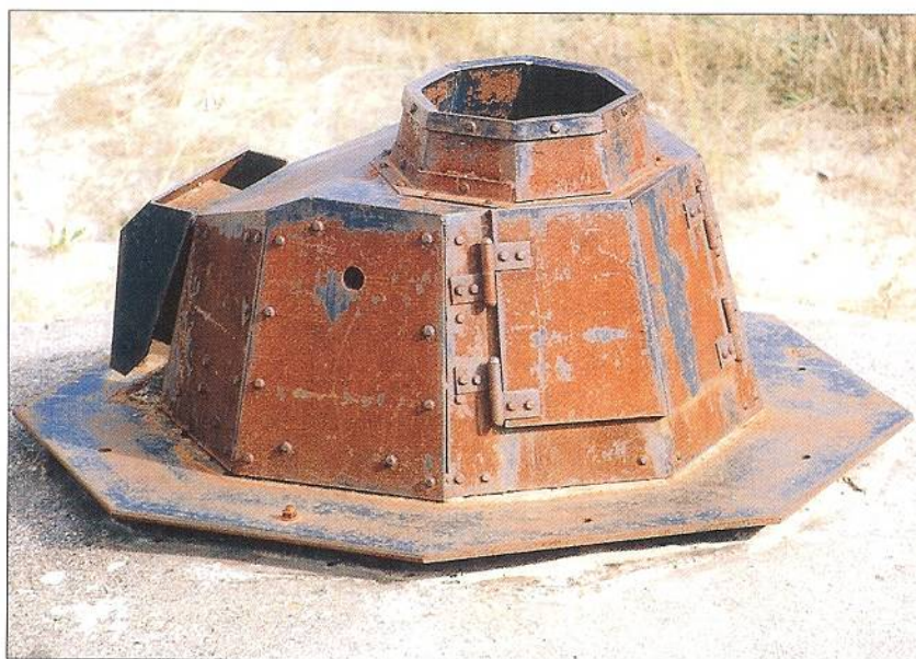
A rusted and incomplete World War I Renault FT tank turret from a tobruk Panzerstellung was one of the surviving remnants of strongpoint W5 on Utah Beach. In recent years it was removed from the beach and placed in the nearby museum due to vandalism. (Neil Short)
