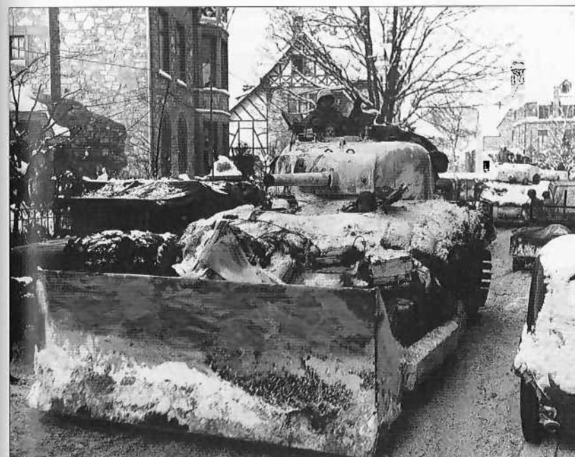
Only the US and British Commonwealth armies employed tank-dozer like this M4 Sherman with an M1 dozer blade; they were extremely useful for breaching (or simply burying) several kinds of obstacle. (NARA, courtesy Steven Zaloga)
