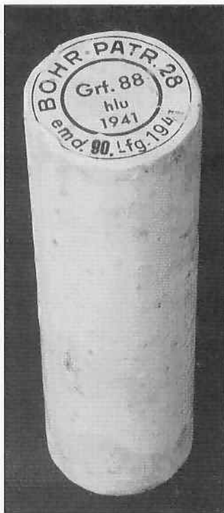
German 100g Bohrpatrone 28 charge ('1928 boring cartridge') – here dated 1941 – packed in tan compressed paper between Bakelite ends. The detonator well is sealed with a pink disc to identify TNT filler. (Private collection)
