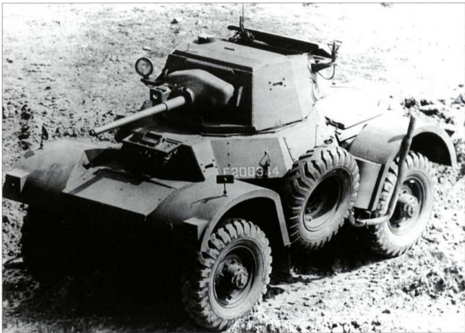
As the landing of a liberation army in North-West Europe drew closer, reconce regiments in Britain were re-equipping with a variety of AFVs. The Daimler armoured car, with a 2pdr main gun, proved highly successful – and this photo reminds us that what looks right usually performs well. The Daimler had a combat weight of just under 7½ tons, a top speed of 50mph and a range of 205 miles; it was highly nimble, and popular with its crews. (Tank Museum 2803/F6)
