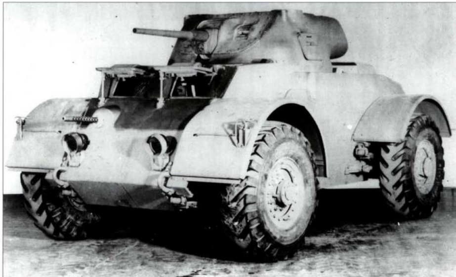
During the Italian campaign, 4 Recce re-equipped its armoured car sections with the American T17E1 Staghound. With a top speed of 56mph and a road range of 450 miles, the Staghound mounted a 37mm main gun and co-axial and bow .30cal machine guns. However, its 13.7 ton loaded weight made it too heavy and cumbersome for the primitive roads of the Italian countryside, and it was more successful in NW Europe. (IWM KID 1268)
