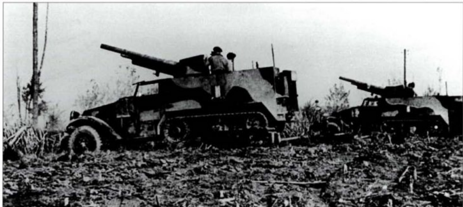
Self-propelled 75mm guns of a Recce unit – possibly those of 4 Recce – in action during the Operation 'Olive' battles, to break through the eastern or Adriatic sector of the Gothic Line, in August/September 1944. These are old US 75mm GMC M3 tank-destroyers – outdated in that role, but still providing useful all-purpose mobile supporting fire for a number of Allied motorized and infantry units. (Tank Museum 2986/E6)
