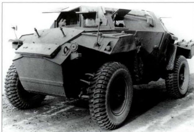
Humber also produced a scout car that was used by Recce units. Heavier and larger than the Dingo, it nevertheless had a slightly higher top road speed of 60mph, and the same range of about 200 miles. (Tank Museum 2085/D4)
