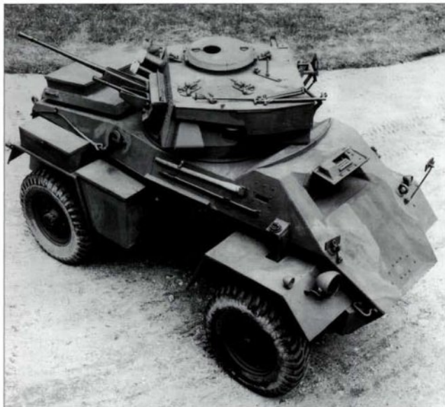
Tunisian experience taught the Corps that something heavier than the LRC was needed. The first 'heavy' armoured car adopted was the Humber, which was used in Tunisia, Sicily, Italy and NW Europe. This car weighed about 7 tons, and was armed with a 15mm and a 7.92mm Besa MG; it had a top speed of 45mph and a range of 250 miles. The Mk II had a three-man crew, which was increased to four in the Mk III but reduced again to three in the Mk IV, which introduced an American 37mm gun as the main armament. (IWM KID 1634)
