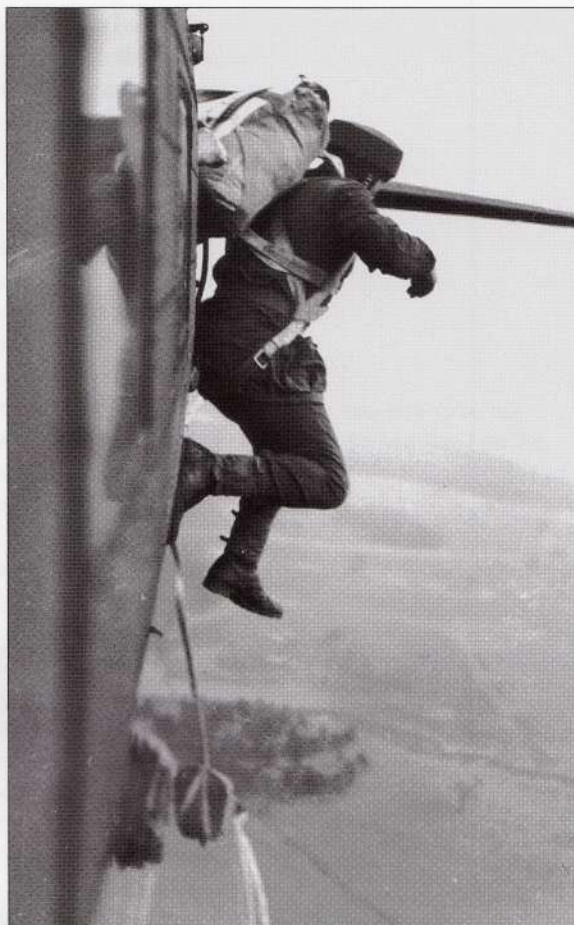
Wearing the canvas-and-rubber training helmet and the X-Type parachute, a soldier of 1 Cdn Para Bn jumps from a C-47 Dakota. The British parachute used a 'canopy last' system which gave less of an opening shock, but the 'canopy first' American rigs could be jumped with greater safety from lower altitudes. Note that the British did not use a reserve pack on the chest. (Photographer Sgt E.R.Bonter, LAC, PA-115865)
