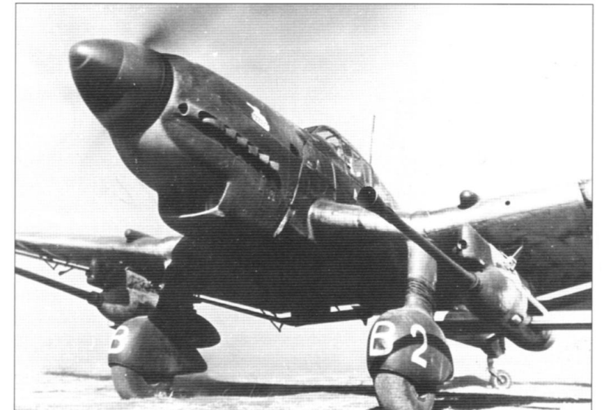
The type of aircraft in which Rudel achieved his extraordinary successes against Soviet tanks: the Junkers Ju 87G, a D-model with two long-barrelled 3.7cm cannon in pods attached under the wings, with horizontal automatic-feed magazines. Although obsolete as an anti-tank gun in ground combat, the 3.7cm was highly effective against the thinner top armour of Soviet tanks. (Private collection)
