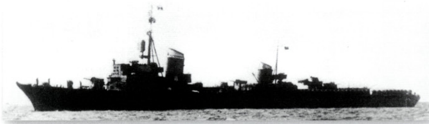
The more rakish appearance of the M39 Elbing class Flottentorpedoboot was not deceptive; this class were a great improvement on their predecessors, being excellent sea-boats and heavily armed. However, only 16 were ever built, and the last five delivered were limited to operations in the Baltic through the earlier loss of Western ports in 1944. (Deutsches U-Boot-Museum)
