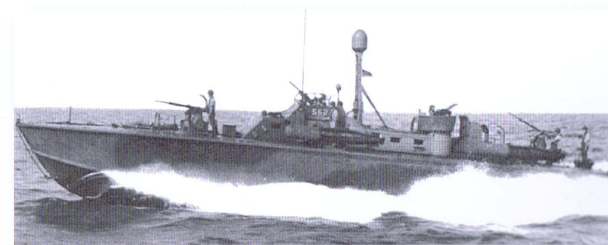
PT 552, a Higgins of the PT 486-563-class, has a second 20mm Mk 4 cannon mounted on the forecastle. The forward 20mm would have a lighter mount than its aft brother.
