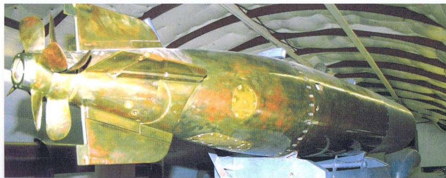
This 22.5-in. Mk 13 torpedo on a Mk 1 Mod 1 roll-off rack displays the bronze body, fins, and two counter-rotating props. The warhead was light gray. Many model kits and other illustrations often depict red warheads. This was never so. PT boat painting instructions stressed that no red would be displayed in any form. Friendly aircraft seeing even a hint of red immediately assumed it was a Japanese flag.
