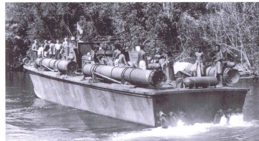
This stern view of an Elco boat displays its Mk 18 Mod 1 torpedo tubes, the Mk 3 smoke generator canister over the stern transom, and its weathered camouflage. Native guides can be seen on the fantail.
