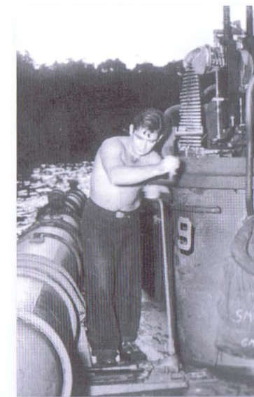
21-in. Mk 1 Mod 1 torpedo tubes had to be hand-cranked outboard before launching. The "fish" were launched at an angle from the boat's course, but the gyros were individually set to turn them on to the correct course with a one-degree spread between each of the four torps.
