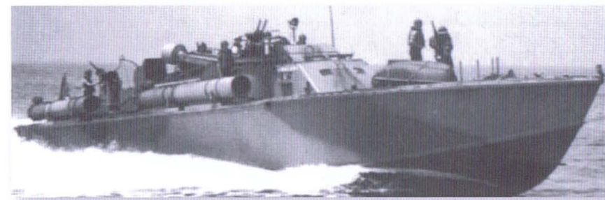
An 80ft Elco at moderate speed. A 6ft wooden dinghy, obtained by many boats for boat to shore movement, is on the forecabin. The SO radar mast is folded down to reduce the boat's profile.
