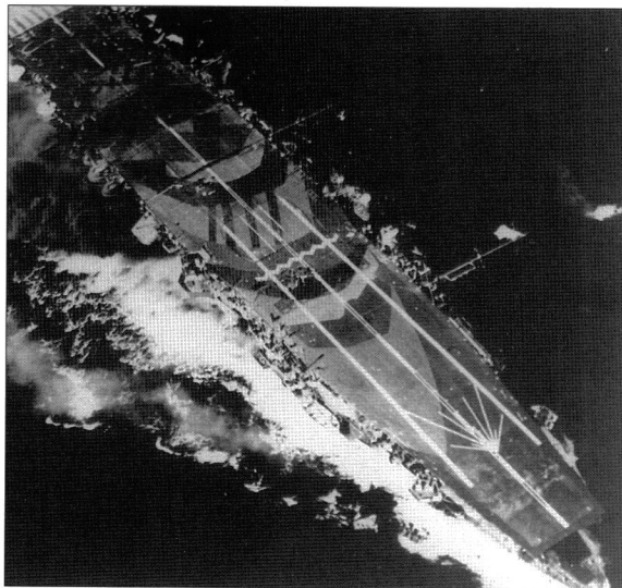
A well-known shot of Zuiho under attack during the battle of Leyte Gulf. Note the flight-deck camouflage; though dramatic it was ineffective. A Type 13 radar can be seen on the lowered mast on the port side. Also note the buckled flight deck aft, the result of a bomb explosion on the hangar deck. (US Naval Historical Center)
