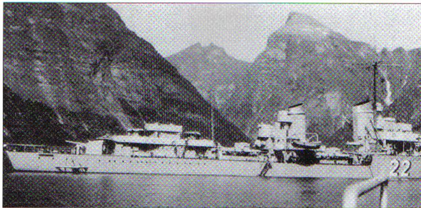
In this view of the after part of Z6, Theodor Riedel , the second and third turrets have been trained to port, exposing the open rear. The structure at the hull side near the stern is a fender, which prevented the side of the vessel swinging hard against a pier or quay and damaging the propellers, which were sited immediately below this area.
