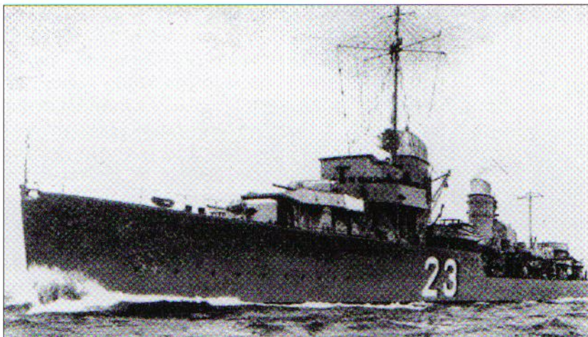
This view of Z7, Hermann Schoemann, shows the distinct lack of rake to the bows of these early Type 34A destroyers. She would be scuttled by her crew after being severely damaged by the cruiser HMS Edinburgh in May 1942 in the Barents Sea.
