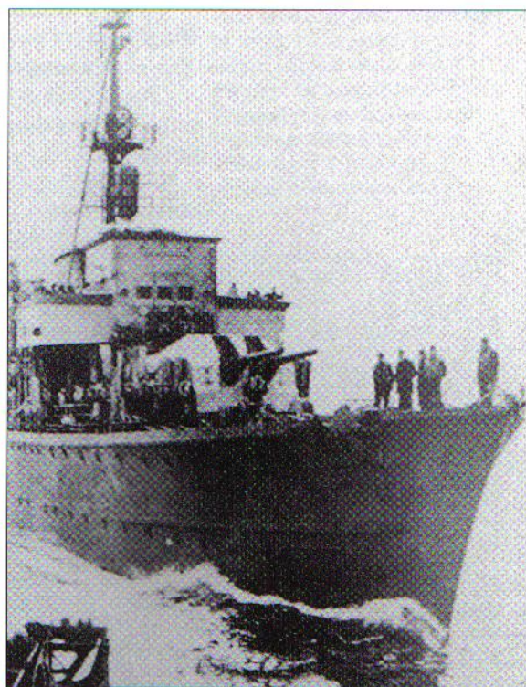
A bow view of one of the Type 36A destroyers. A quadruple 2cm Flakvierling anti-aircraft gun is mounted to the rear of the large 15cm twin turret. This class also featured a searchlight platform on the foremast.
