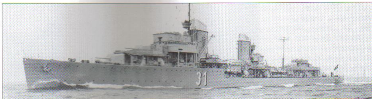
Z15, Erich Steinbrinck , in pre-war livery. Note that her bows lack the extreme clipper-style rake common to all destroyers from Z20 onwards.
