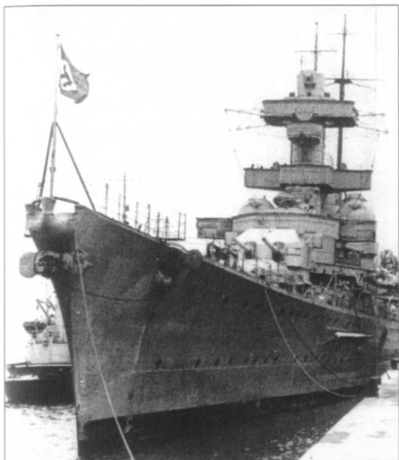
The final bow configuration for Blücher is shown here. Note the change in anchor positions from that shown in the photograph of her launch. There are now one to either side of the bow, in an anchor cluse on the forecastle, and one on the stem itself.
