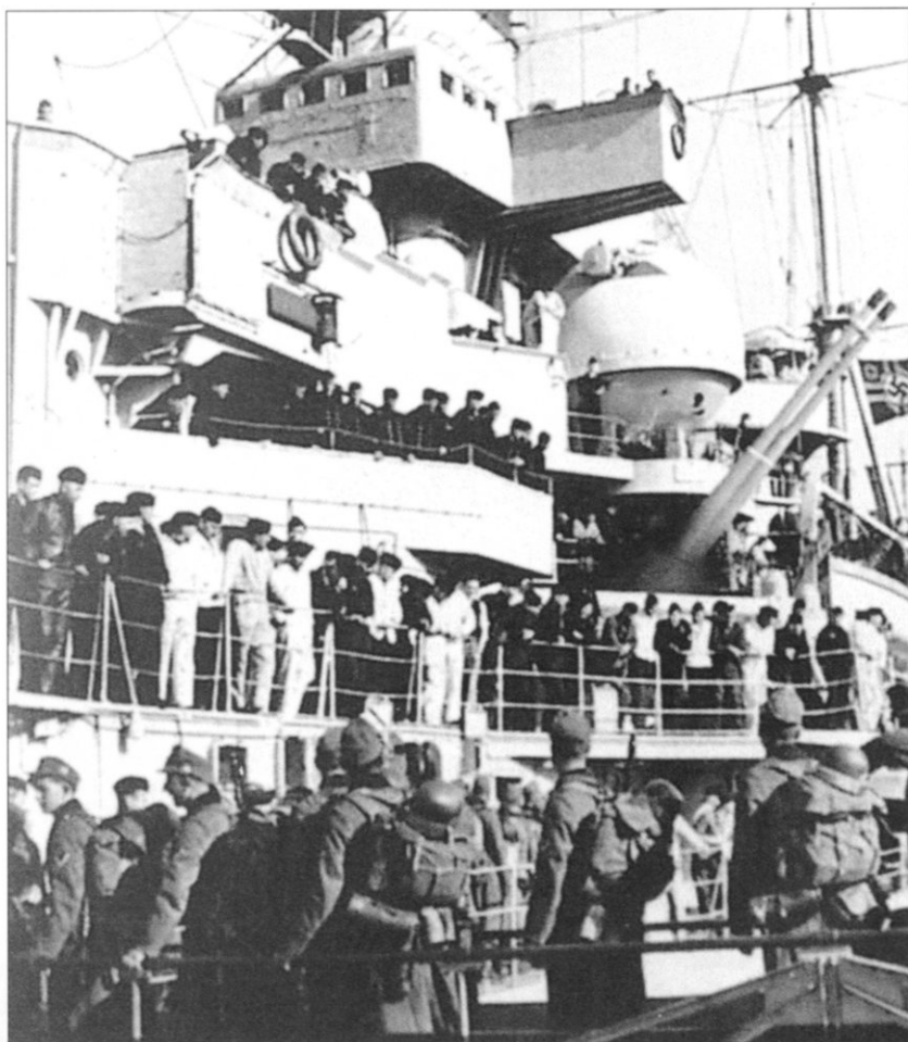
A further view of Admiral Hipper 's forward superstructure, during the embarkation of her passengers. Clearly shown here is the searchlight platform just above the enclosed bridge and the heavy flak guns pointing skywards with their spherical fire control housing just above.
