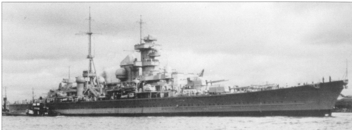
Admiral Hipper in modified guise. Note the bridge is now enclosed, the straight stem is replaced by the clipper-style bow, the raked funnel cap is fitted, and the foretop rangefinder now has a FuMO 'mattress' radar antenna fitted to its face (concealed by a canvas cover in this shot).
