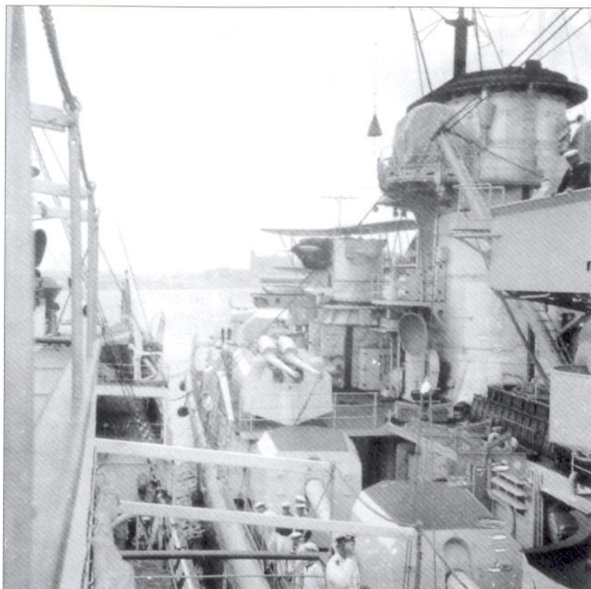
A fine midships view of Admiral Scheer . Clearly visible are the secondary armament turrets and heavy flak guns. Note the searchlights, covered in canvas here, on the funnel platform. Just below and to the left of the searchlight can be seen the fire control rangefinder for the flak armament.
