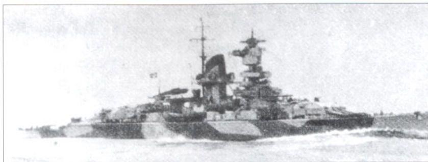
In her late-war guise, Admiral Scheer featured a raked clipper bow and, as seen here, often sported a disruptive 'splinter' camouflage scheme of dark grey bands over a light grey base coat. Note also the high, raked funnel cap.
