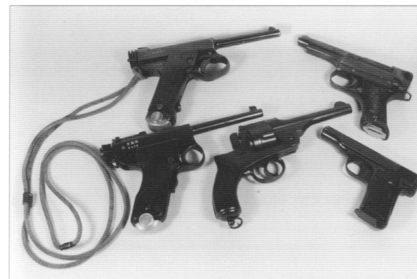
Five models of handguns used by the IJN. (Top left) 8mm ("Papa") Nambu Type 14 with lanyard, and large modified trigger guard; (bottom left) improved 1904 Nambu, with Navy anchor marking; (center) 9mm Type 26 revolver; (top right) 8mm Type 94; (bottom right) imported 7.65mm Fabrique Nationale/ Browning M1910. (Steve Hayama)
