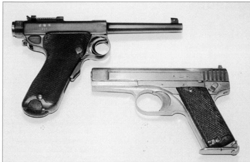
(Left) 1904 ("Grandpa") Nambu, recognizable by the adjustable tangent rear sight and the grip safety catch; (right) a 7.65mm Type Hamada. (John Ziobro)
