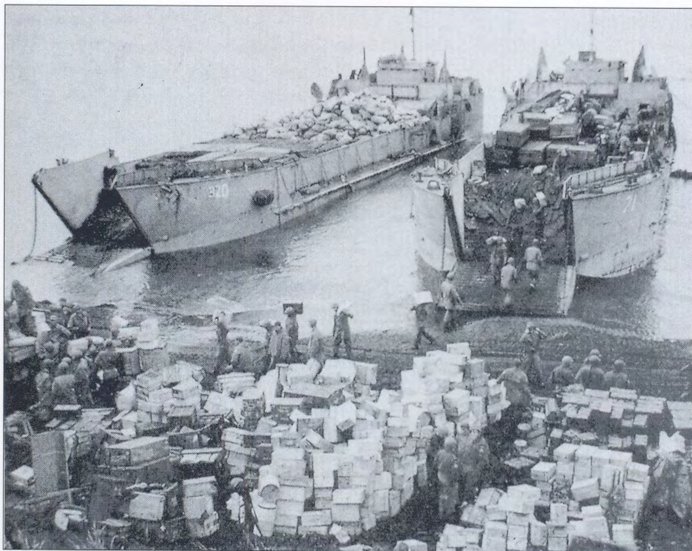
Two LCT(5)s offload cargo; besides three medium tanks, an LCT could carry a huge amount of general supplies. The beach space dilemma is vividly demonstrated here – the beachmaster is probably trying to decide where to dump the arriving cargo.
