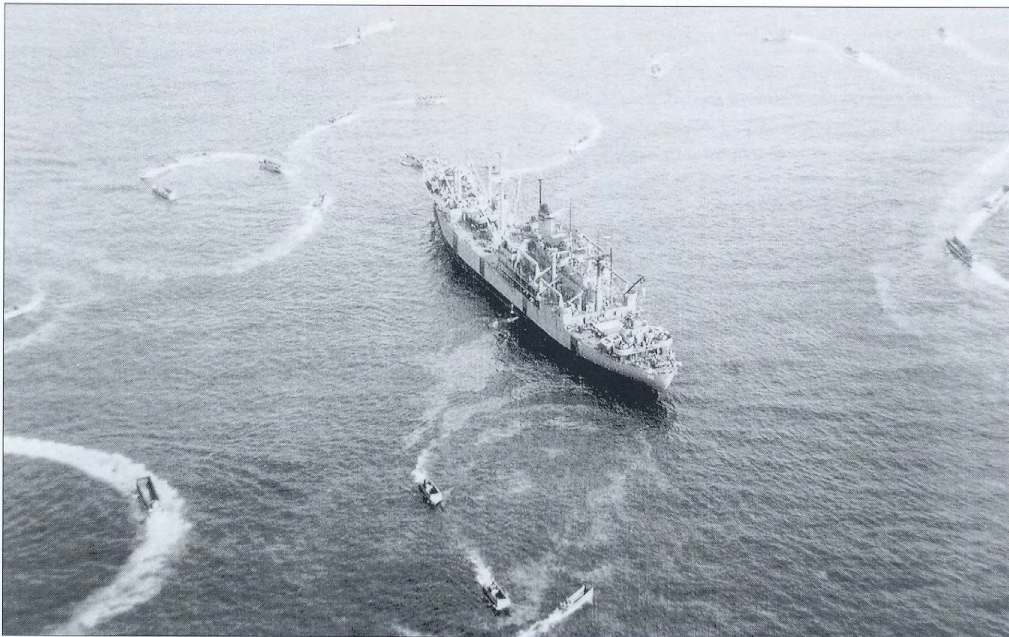
LCVPs from the USS Chinton (APA-38), a Bayfield Class attack transport, circle prior to forming up into assault waves. The dark panels along the hull sides mark the boat stations. Note that the groups of landing craft are circling clockwise and counter-clockwise: the theory was that if they collided they were going in the same direction and would glance off, causing less damage than if heading into one another.
