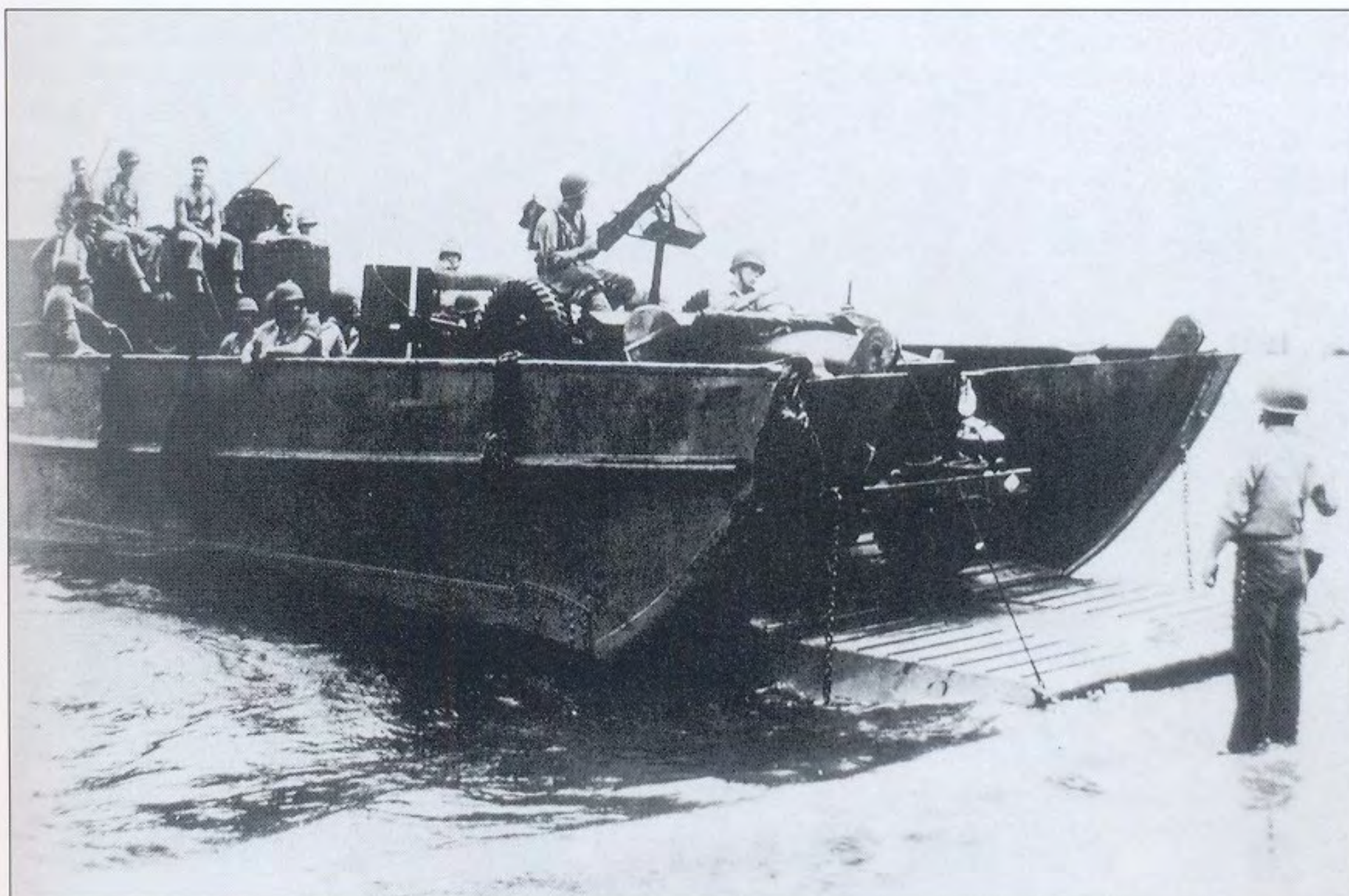
In the early Solomon Islands campaign large beaching craft, such as the LST and LCI, were not yet available. This Landing Craft, Medium Mk II, seen disembarking a Marine 1-ton truck on Guadalcanal in November 1942, was one of the largest beaching craft available for this early operation.
