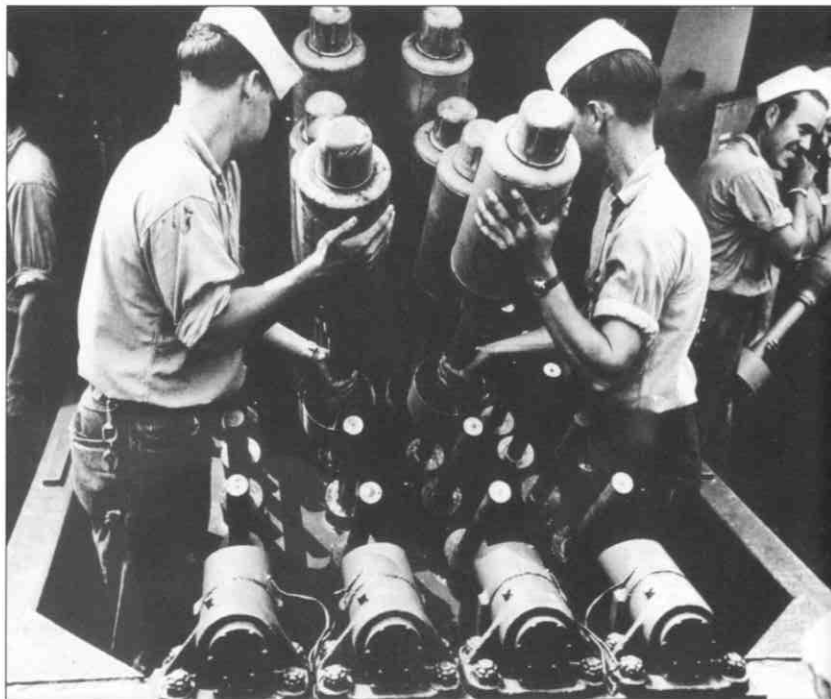
Sailors in standard shipboard fatigue uniform of 'dixie cup' hats, chambray shirts and dungaree trousers loading a 'Hedgehog'. By 1943 these forward-firing projectors were deployed on destroyers to allow quicker engagement of submarines. This device had six rows of spigot mortars with 24x 65lb. projectile warheads which could be fired in a pattern 200 yards in front of a destroyer as it approached a submarine's suspected position, instead of having to wait to drop depth charges as it passed overhead. The sinking warheads detonated if they struck a hull; a miss allowed sonar operators to stay on their phones, tracking the contact. A smaller eight-warhead device called a 'Mousetrap' was installed on some vessels.
