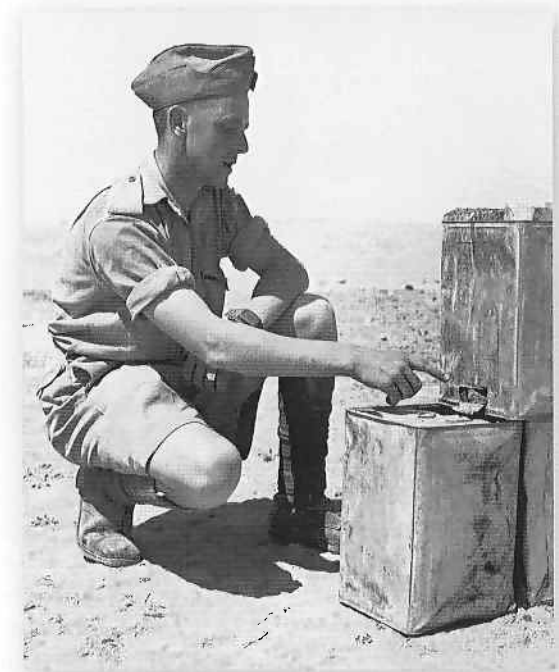
Water was precious in the desert and every drop that could be saved was put to good use. Here a soldier is recycling some dirty water using a primitive filter. Unclean water was poured into the top of the empty cans and then descended through layers of sand and small stones to emerge at the bottom, void of much of its earlier contamination. (IWM, E 12283)
