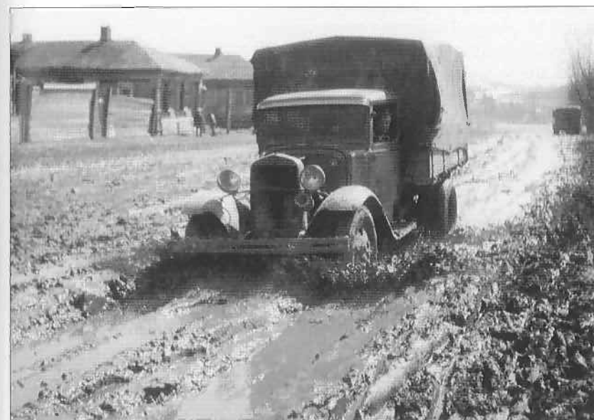
A captured Soviet GAZ-AAA truck in German service on a muddy road in autumn 1941. The Germans had captured thousands of Soviet trucks, and they performed better than most German vehicles under these primitive conditions. (Nik Cornish)
