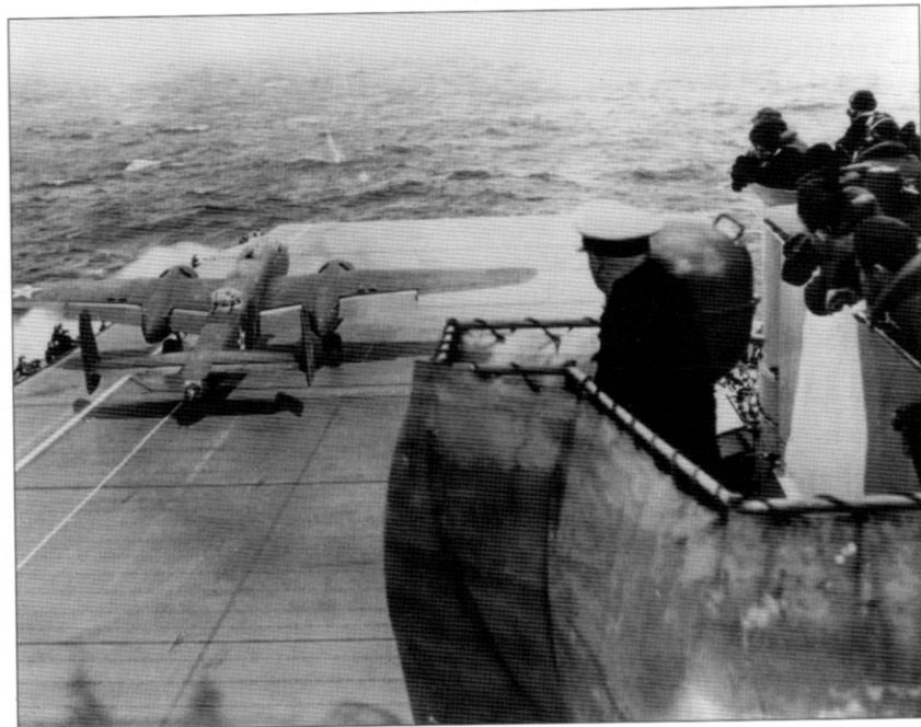
This photograph shows the rough sea conditions and overcast weather at the time of take-off. The tail guns were wooden dummies, intended to frighten any Japanese fighters. (US Navy)
