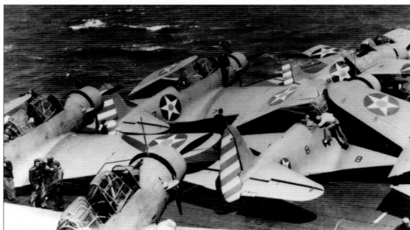
The Enterprise (CV 6) had a mix of aircraft. They included the three-man torpedo bomber, TBD-1 Devastators and the fixed-wing F-4F-3 Wildcat fighters. (US Navy)
