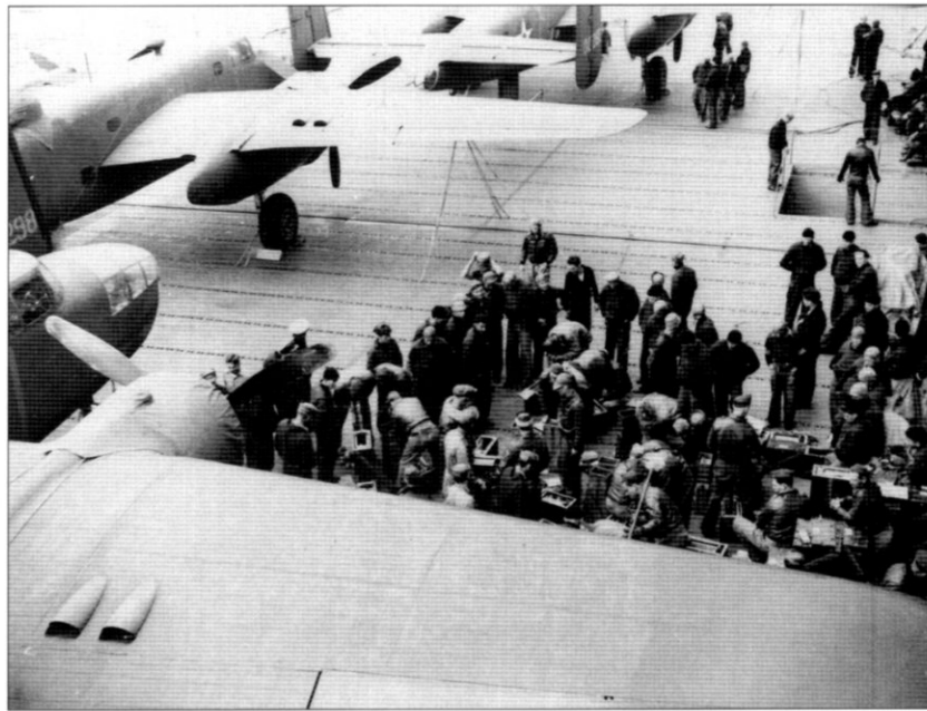
The B-25B crews relied on twin mounted .50-caliber machine guns in a top turret and a .30-caliber gun in the nose. Here, army personnel are loading .50-caliber ammunition into canisters. (US Navy)
