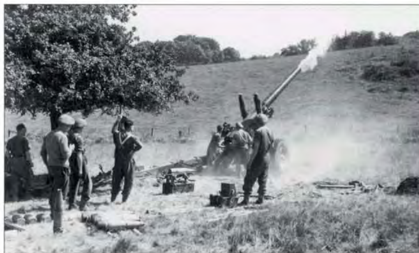
British 5.5in. (140mm) medium gun firing in support of Operation Bluecoat north of the River Orne. This type of gun fired a 45kg shell to a maximum range of 14,800 metres. Each medium regiment had 16 of these guns. (Imperial War Museum, B9174)
