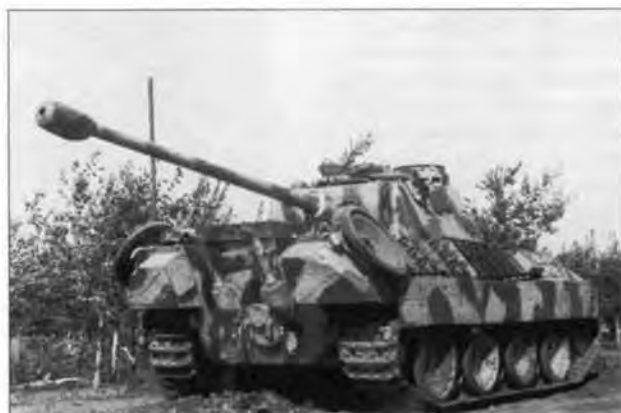
A PzKpfw V Panther tank with its long 75mm gun pointed to the rear. The Panthers were in Normandy in sufficient quantities to take a heavy toll of Allied armour. It was designed in response to the Russian T-34 medium tank and incorporated similarly sloped armour. The Panther was considered as probably the best of Germany's tanks. (Bundesarchiv, 1011-705-0264-01)
