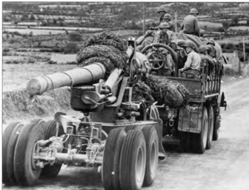
American 155mm gun being towed forward during the American breakout. This large weapon had its origins in the French 155 GPF gun adopted by the Americans in 1917. Its M1 carriage was designed for high speed and manoeuvrability with pneumatic tyres and air brakes. (US National Archives)
