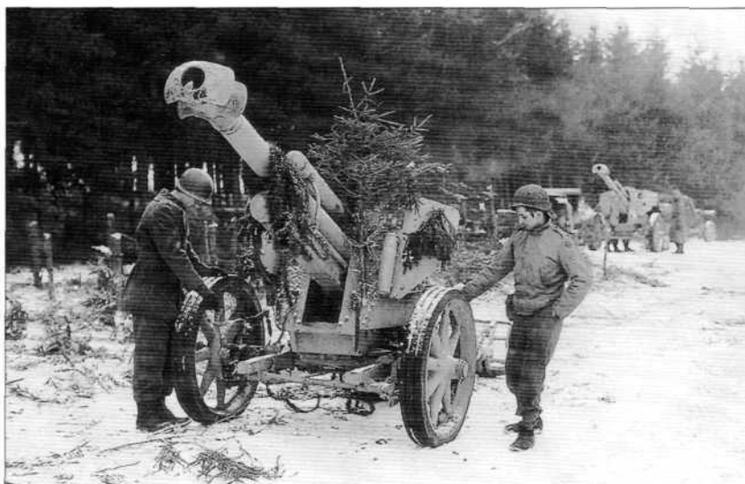
The workhorse of the German field artillery was the 105mm field howitzer like these that were captured by the 35th Division near Luttrebois on 17 January 1945. This is the improved leFH 18/40, which used the lighter carriage of the PaK 40 anti-tank gun. (NARA)
