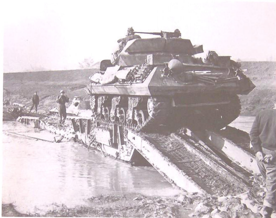
In British service the M10 was known as the Wolverine. This V Corps vehicle is seen being guided across the River Savio on 23 October 1944, using a causeway of Churchill ARKs. A 'dead' Panther lies beyond. The crew are clearly experienced at looking after themselves, as can be seen by the neat, secure stowage, the 'acquired' oversize funnel (an invaluable aid during replenishment), bivouac stakes and bucket. (Imp. War Mus.)
