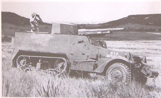
75mm Gun Motor Carriage M3, with front and side-door screens raised. (RAC Tank Museum)
