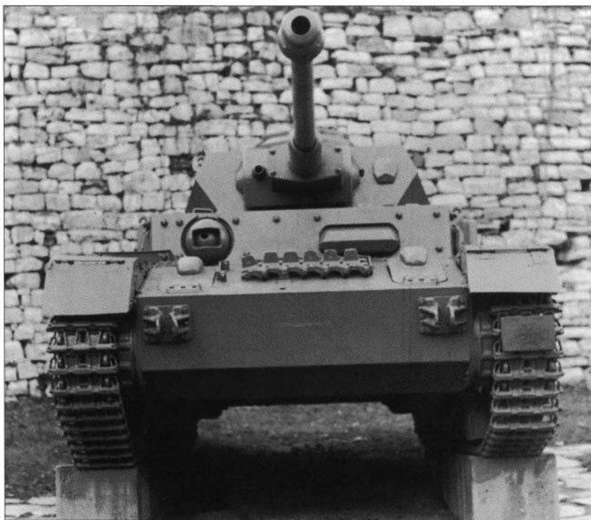
This Pz.Kpfw.IV Ausf.H. was assembled by Vomag in July 1943. The additional 30 mm plates were bolted on the 50 mm frontal armour to speed production. The hull front was made from an 80 mm-thick plate that had become available. This Pz.Kpfw.IV Ausf.H. is now on display in Belgrade, Serbia. (TLJ)
