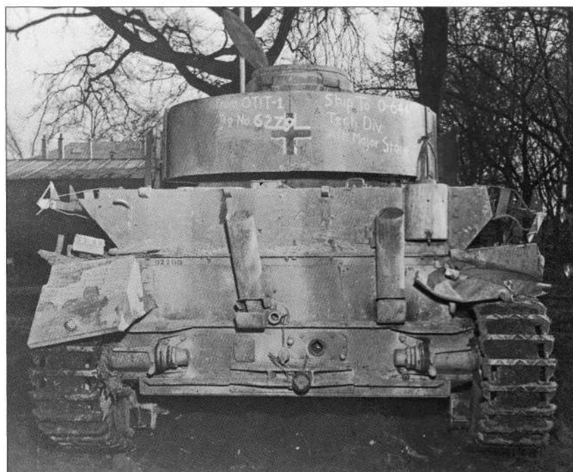
Pz.Bef.Wg.IV. Ausf.J. Fgst.Nr. 92220. The mounting for the 'Sternantenne' was moved to the rear plate. The tripod fitting on the rear antenna base is the bottom section of a unit that raised the height of the antenna by 0.7 m extension pieces. (TTM)
