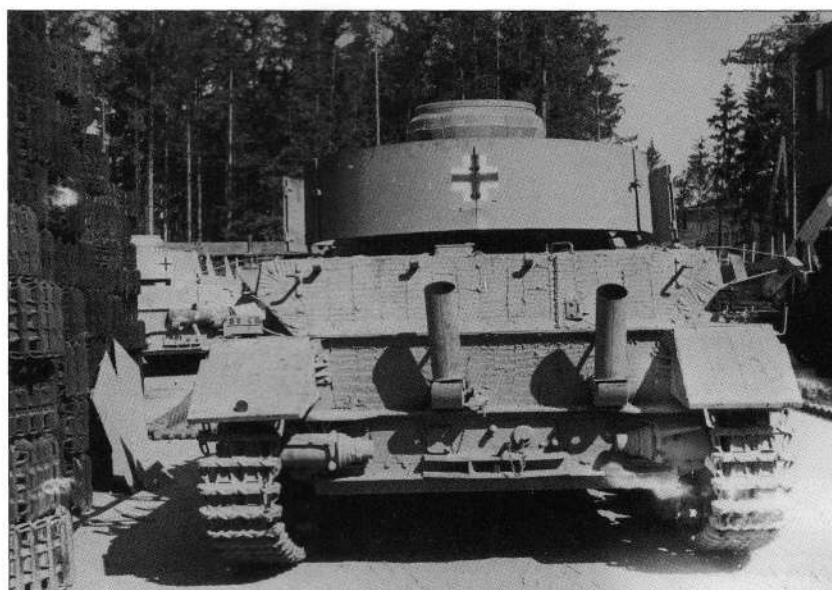
Rear view of a Pz.Kpfw.IV Ausf.J. assembled by Nibelungenwerk in August/September 1944. The Flammentöter exhaust system replaced the cylindrical muffler in August 1944. (WJS)
