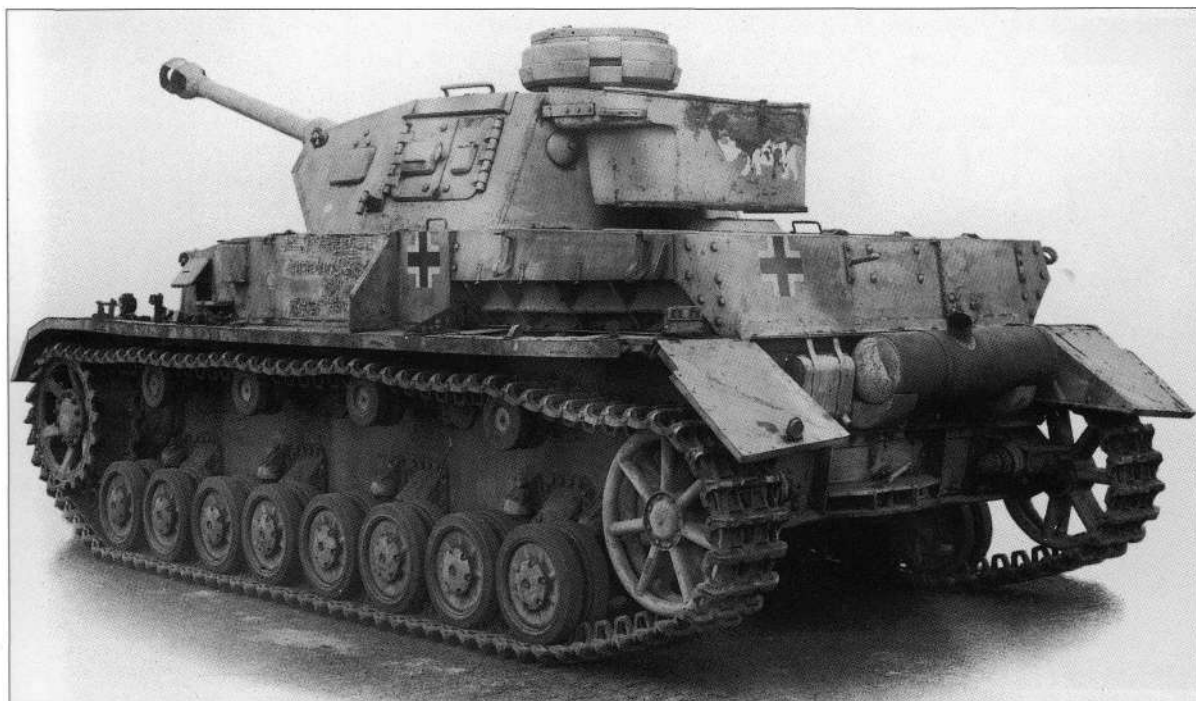
The rear view of Pz.Kpfw.IV Ausf.G. Fgst.Nr. 83072. On the left mudguard are the remains of the rack for mounting two spare wheels. (TTM)
