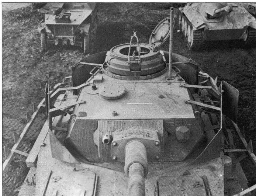
Pz.Bef.Wg.IV. Ausf.J. Fgst. Nr. 92220 was assembled by Nibelungenwerk in September 1944. This tank was completed as a new command vehicle. The turret antenna was mounted in the blanked-off opening for the Nahverteidigungswaffe. The periscopic observation TSR1 is raised to its full extent in this photo. (TTM)
