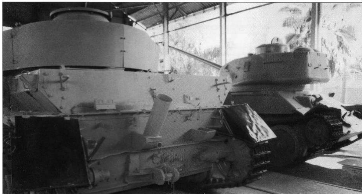
BELOW Rear view of Pz.Kpfw.IV Ausf.J. Fgst.Nr. 110021 shows the extended hull sides forming tow brackets and final form of tow bracket for use with towbars. (Hilary Louis Doyle)
