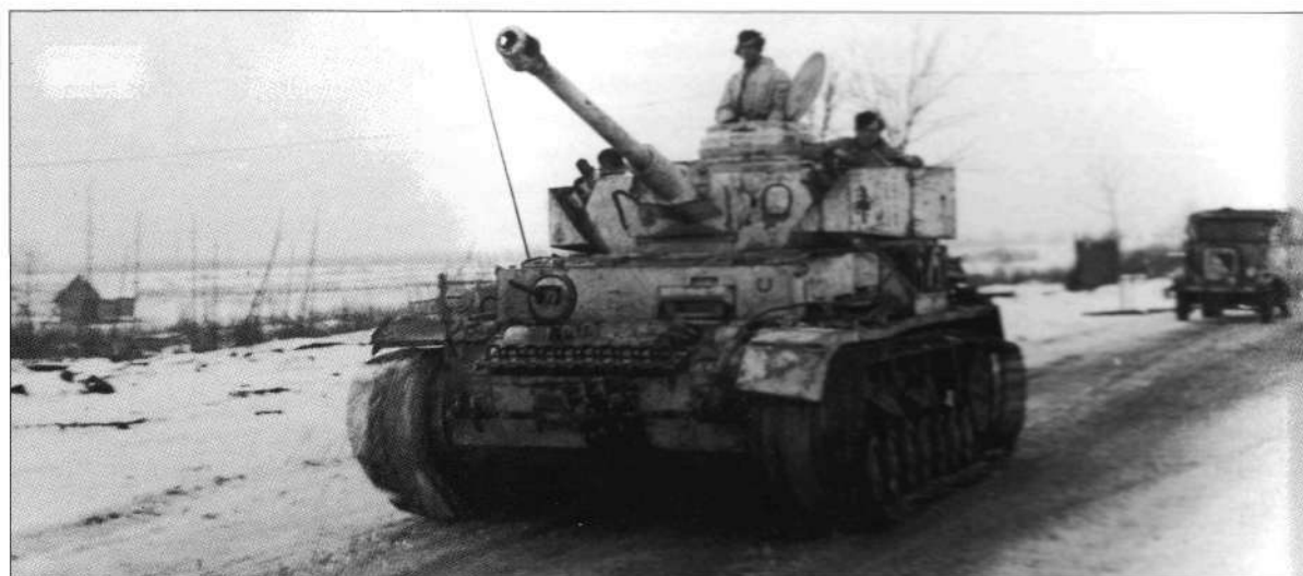
Pz.Kpfw.IV. Ausf.G 7.5cm Kw.K 40 L/48, welded 30 mm extra armour on the front surfaces, Schürzen, smoke candle dispensers. The wider 'Winterketten' (winter tracks) have been fitted for better flotation on snow. (BA)
