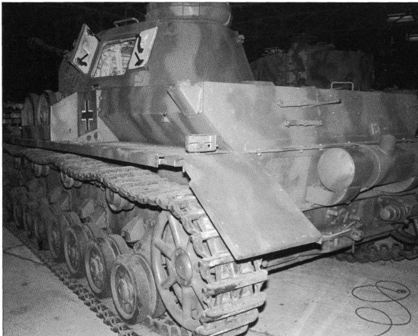
Pz.Kpfw.IV Ausf.J. Fgst.Nr. 86432. With the elimination of the electric turret drive on the Ausf.J the auxiliary generator set was removed along with the associated exhaust muffler.
