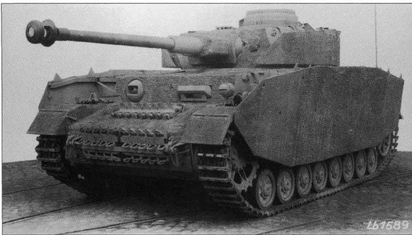
A Pz.Kpfw.IV Ausf.H. Fgst.Nr. 84599 assembled by Krupp-Grusonwerk in September 1943. It is one of the first vehicles coated in Zimmerit anti-magnetic paste, which was introduced to protect vehicles from magnetic grenades. The practice of coating the side Schürzen with Zimmerit was discontinued after a short period. (BA)
