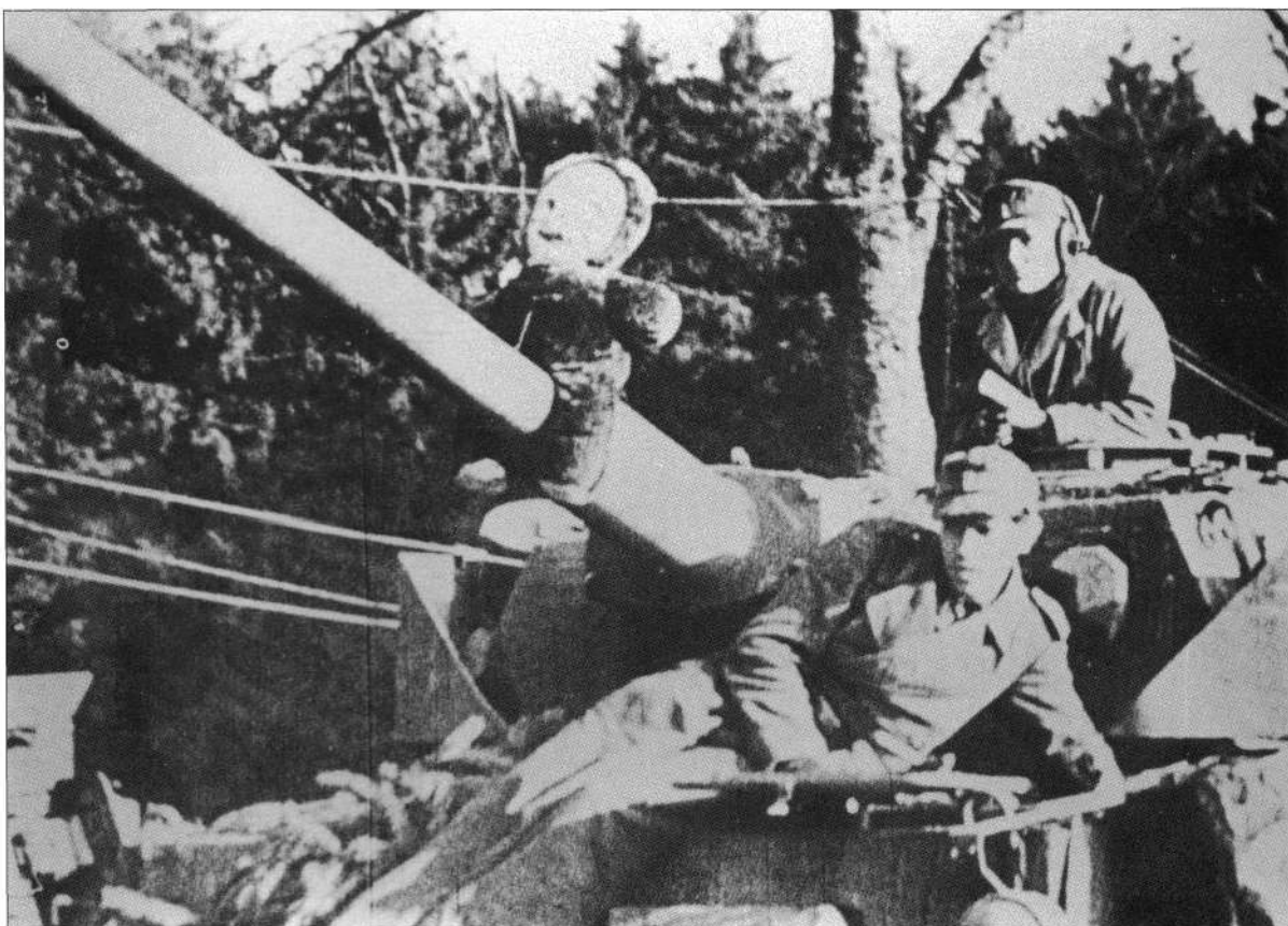
Pz.Kpfw.IV Ausf.J, converted to a Panzer Beobachtungswagen IV with the Sturmgeschütz commander's cupola, in service during the Ardennes Offensive.
