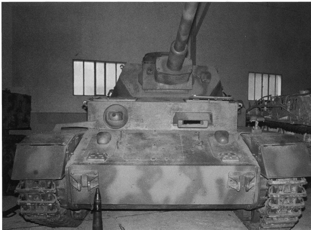
Pz.Kpfw.IV Ausf.J. Fgst.Nr. 86432 assembled by Vomag in February 1944 and on display in Musée des Blindés, Saumur. The interlocking side and front hull plates were characteristic of the Ausf.J but were introduced with some of the final Ausf.H.
