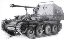
Late-model Marder IIIs were armed with the German 75mm Pak 40/3, with the engine relocated 'amidships' and the fighting compartment at the rear. Note the small rectangular hole cut in the armour right of the gun, for the gunner's telescope; and the travelling crutch for the gun. To free the armament the gunner simply elevated the barrel, and the crutch fell away. (RAC Tank Museum)
