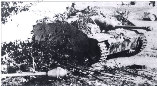
Two concepts of anti-tank defence; a StuG III Ausf. G, with 'Saukopf' mantlet and skirt armour, for distant targets, and the infantryman's hand-held Panzerfaust for close-quarter fighting. (Bundesarchiv)
