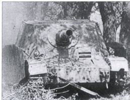
An abandoned Brummbar with skirt armour: note the late driver's vision block, identical to that used on the Tiger Ausf. E, and details of the ball-mounted 150mm howitzer. (RAC Tank Museum)
