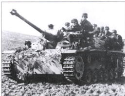
A small number of assault guns were sent to Tunisia shortly before the collapse, and this photo shows an Ausf. F, with L48 gun, in that theatre. The paint scheme seems to be overall light desert yellow, with applied scrub foliage. This may be a gun of the incomplete 'Hermann Göring' Division. (Bundesarchiv)
