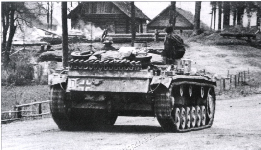
A StuG III Ausf. E moving past a blazing Russian farm: the loader sits on the right-hand radio pannier, which became standard with this model. Note the Gothic 'D' at the left end of the rear hull plate. (Bundesarchiv)
