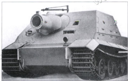
A Sturmgeschütz, showing missile derrick, and prominent muzzle counter-weight on the rocket launcher. (RAC Tank Museum)
