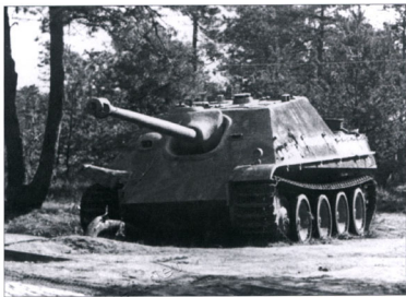
For all that it was a formidable opponent, the Jagdpanzer could be a mechanical mine of trouble after 900km running, and after 1,000km it required a complete overhaul. (The Tank Museum)
