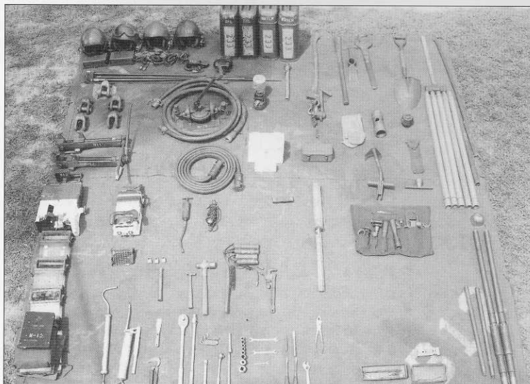
Maintenance gear for an M48A3 tank, laid out for inspection. Most of these items are illustrated in the Plates. The coiled items at upper left are the refueling hoses and hand pump, and the slave cable used to start a tank with dead batteries. (NARA)
