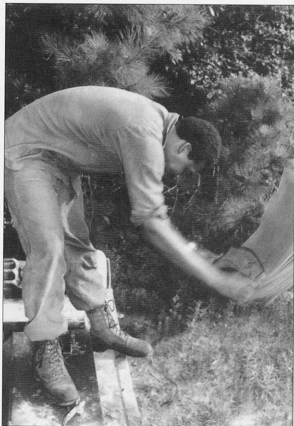
A tanker cleans the air filter baffles by beating them against the fender of the tank. Constant cleaning of the air filters was but one of the many daily maintenance tasks required to keep tanks in good operating condition. (NARA)
