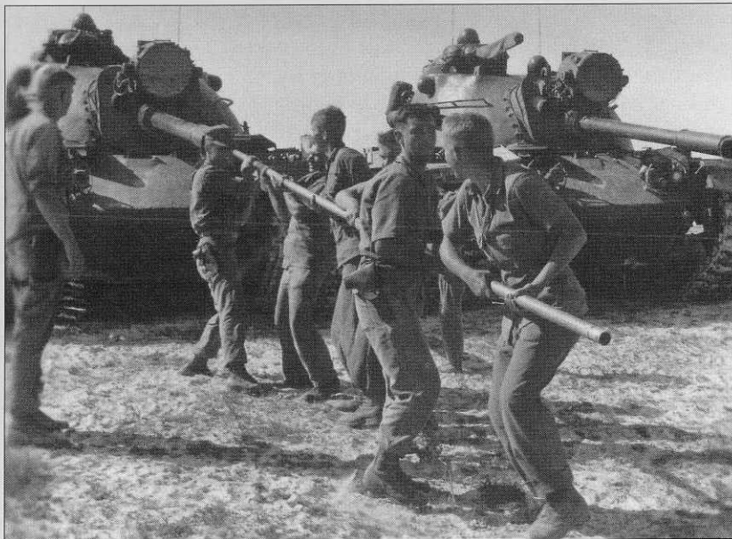
Regardless of combat operations, daily life involved the endless routine of daily maintenance. These crewmen are “punching out” the gun tubes – cleaning them after firing – with several crews working together. (USMCRC)
