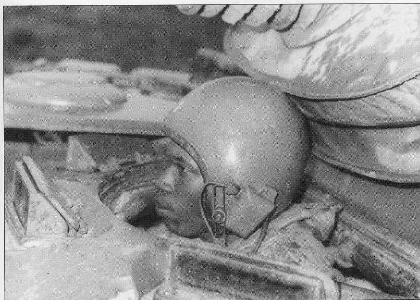
This photo of a typical tank driver illustrates the mud-encrusted driver's vision periscopes that often forced the driver to operate the tank either with his head exposed, or blind under the verbal directions of the tank commander. (NARA)
