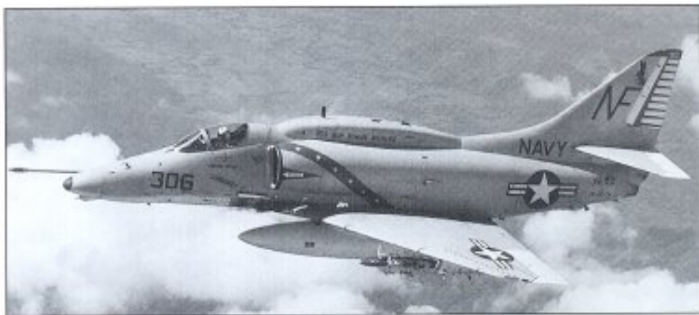
A-4F BuNo 154217 from VA-22 shows the distinctive dorsal hump that housed avionics and made room for restored ammunition in the fuselage. This photo was taken during the unit's 1969 war cruise. BuNo 154217 is presently on display in the National Museum of Naval Aviation at NAS Pensacola, Florida (Lt W E Bradford)
