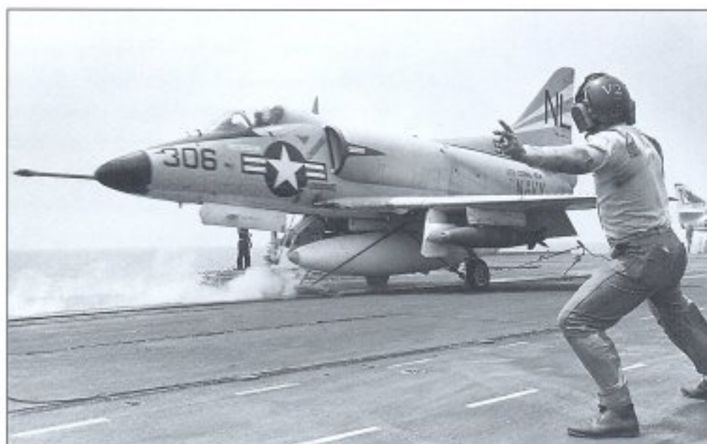
A-4C BuNo 149574 from the 'Blue Tail Flies' of VA-153 launches from USS Coral Sea on 24 March 1965. The aircraft carries Mk 84 2000-lb bombs as well as the normal 300-gallon fuel tank. This aircraft was brought down by AAA northwest of Thanh Hoa three months later on 25 June while being flown by CVW-15 CAG, and ex-VA-153 CO, Cdr Peter Mongilardi. The latter failed to eject from the jet and was killed, thus becoming the first CAG to be lost in action in the Vietnam War (PH1 James F Falk)
