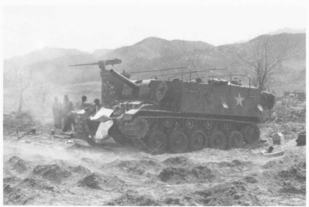
Similar in configuration to the M7 Priest, the M37 Howitzer Motor Carriage was based on the chassis of the M24 Chaffee and entered service in the closing days of the Second World War. Here, M37s of 58th Field Artillery Bn. fire their 105mm howitzers across the Imjin River in support of 3rd Infantry Div. on 12 April 1951. With an air-recognition panel draped across the glacis plate, the nearer vehicle sports a large cartoon on the machine gun pulpit depicting a flaming devil with the name 'Hell Fire' above. (US Army SC363745)
