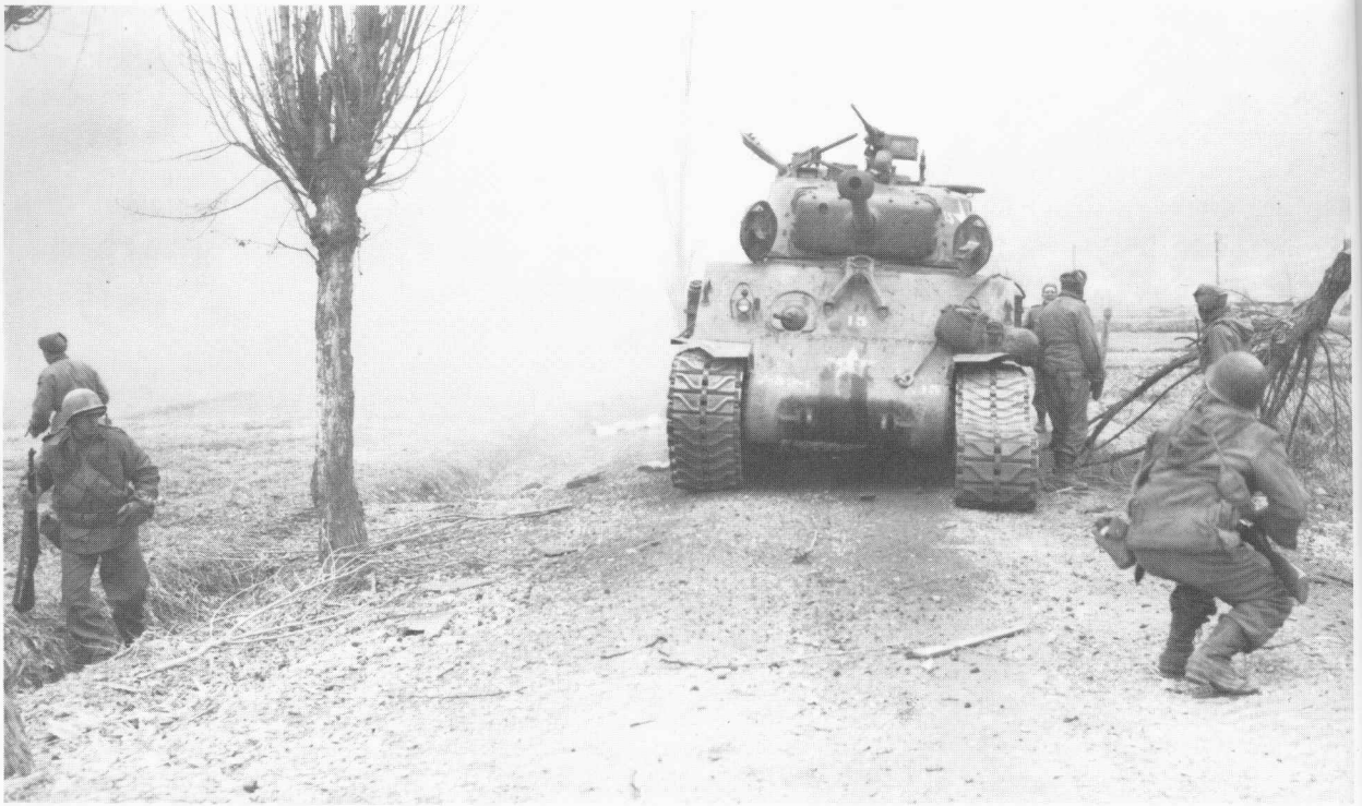
Infantrymen scramble for cover as mortar fire falls near an M4A3(76)W HVSS of 32nd Regimental Combat Team, 7th Infantry Div. which has just run over an anti-tank mine on the outskirts of Hadaewa; 28 February 1951. Almost 70 per cent of UN tank casualties were caused by mines. Often of crude construction, the wooden box-mines were virtually impossible to detect with electromagnetic mine detectors, and no effective counter-measures were found against them. Detection was only guaranteed by laborious probing with bayonets. The .30cal.M1919 Browning machine guns were frequently mounted forward of the commander's cupola to allow him to fire a weapon from within the turret, rather than exposed on the engine decks as was necessary with the .50cal. on its 'sky-mount'. (US Army SC359465)
