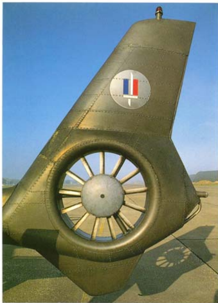
Above An unusual feature of the Gazelle, and several other Aérospatiale designs, is the shrouded tail rotor, known as a 'fenestron'
