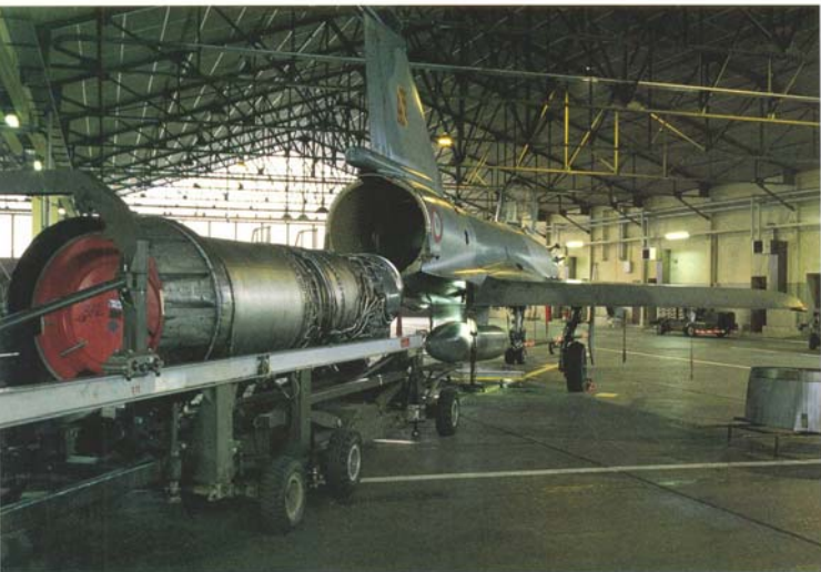
In the EC 3/2 'Alsace' hangar a SNECMA M53-5 is shoehorned back into place after servicing in the GERMAS workshops. At the time of writing it is not expected that EC 2 aircraft will be retrofitted with the M53-P2 engine, although they will have their radar installations updated to the RDI
