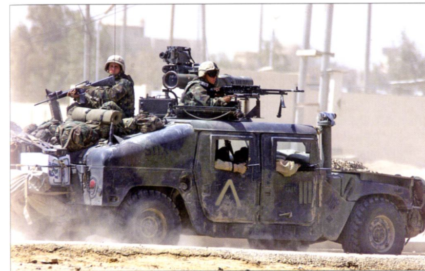
A Marine M1045A1 TOW carrier of Task Force Tarawa during fighting near Nasiriyah, Iraq, in April 2003. The Marine HMMWVs had many small modifications prior to the start of Operation Iraqi Freedom , including the addition of the commercial Gypsy Rack to the rear of the vehicle to provide more stowage for prolonged operations. (Cpl Gordon Rouse, US Marine Corps)
