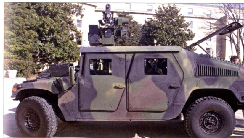
The ultimate package for protecting the HMMWV consists of the Add-On-Armor package as well as the CROWS remote-controlled weapon station, which allows the crew to operate the vehicle weapon from within the vehicle. This vehicle was displayed at the Pentagon in February 2004. (US Army)
