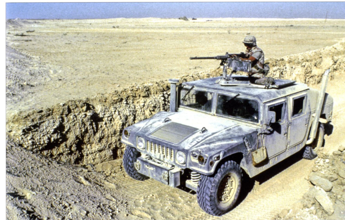
A Marine Corps M1043 armament carrier is seen taking shelter during Operation Desert Storm in February 1991. The Marine HMMWVs can be distinguished by the flat door panels as well as the deep-wading extension to the exhaust seen near the rear wheel. (USMC)
