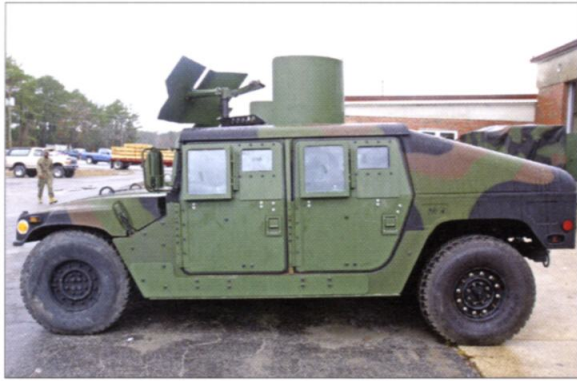
TOP LEFT The Marine Corps developed its own up-armor package for Iraq called the MAK, seen here fitted to an M1043A1 weapons carrier of the 26th Marine Expeditionary Unit in December 2004, shortly before the unit was deployed to Iraq. (Lance Cpl Daniel Lowndes, US Marine Corps)
