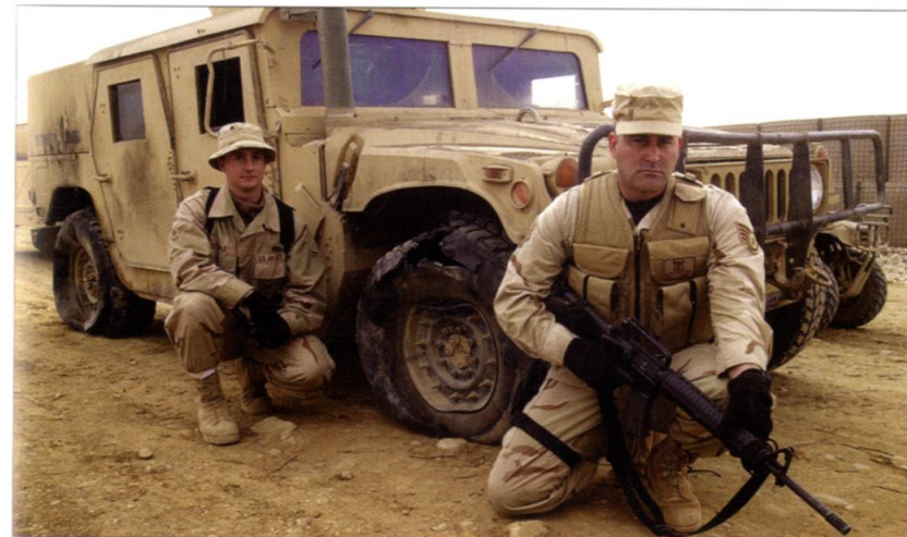
The need for HMMWV protection is evident in this view of an M1116 UAH of the Air Force 455th Expeditionary Operations Group, which ran into an unmarked minefield while patrolling near Bagram air base on January 5, 2005, shredding both tires. Both airmen were uninjured, as seen here. (Tech Sgt Brian Davidson, US Air Force)
