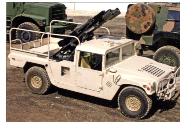
BOTTOM RIGHT The more robust Heavy HMMWV Variant family permits more elaborate armament options, like this Singapore Technologies Super Rapid Advanced Mortar System (SRAMS), which can fire up to 18 120mm mortar rounds per minute. It was first displayed in February 2005 at the IDEX show in the United Arab Emirates. (Author)
