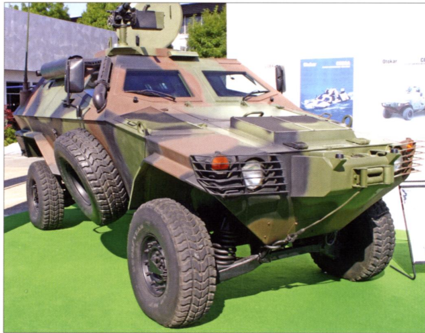
Otokar's Cobra is a light armored car using the HMMWV suspension and powertrain, but with a fully armored body. It has been built for the Turkish Army and at least one other army. (Author)
