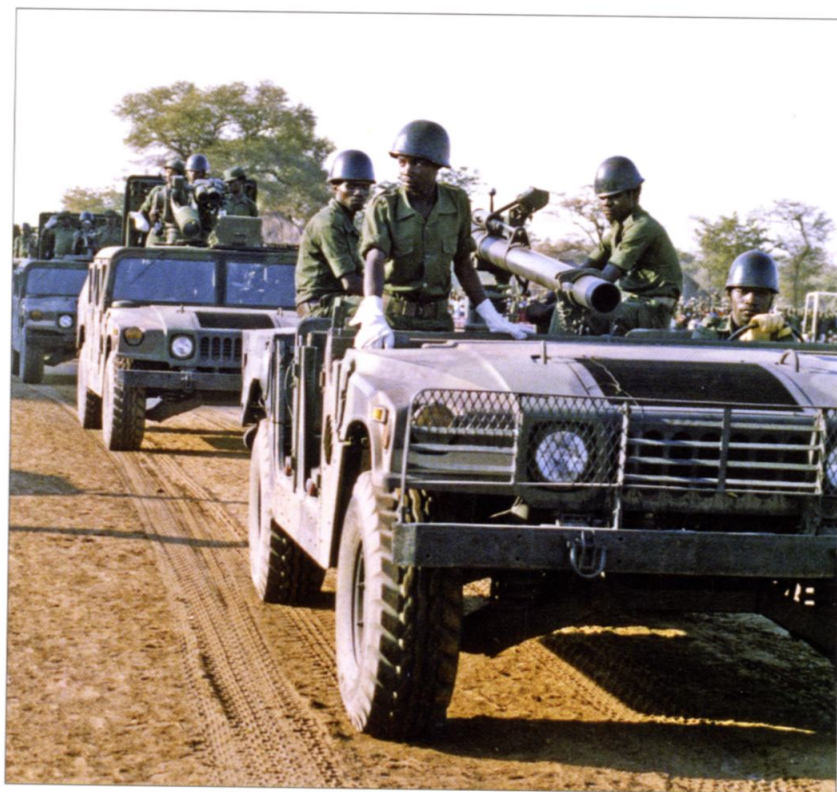
The first combat deployment of HMMWVs by forces other than those of the United States was as "gun buggies" by the UNITA cassador mobile battalions during the fighting with the FAPLA in Angola in 1989-90. The lead HMMWV here is equipped with a US 106mm recoilless rifle. (Free Angola Information Service)
