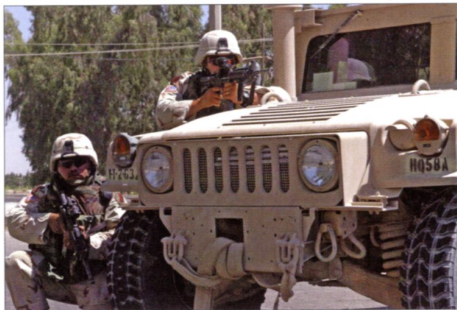
Troops of Task Force 2-63d Armor pull security at a checkpoint near Baqubah, Iraq, in June 2004. This close-up shows the prominent nose of the ECV variants of the HMMWV family like this M1114 UAH. Also noteworthy is the larger winch opening characteristic of the -A2 variants and later models. (Sgt Kimberly Snow, US Army)
