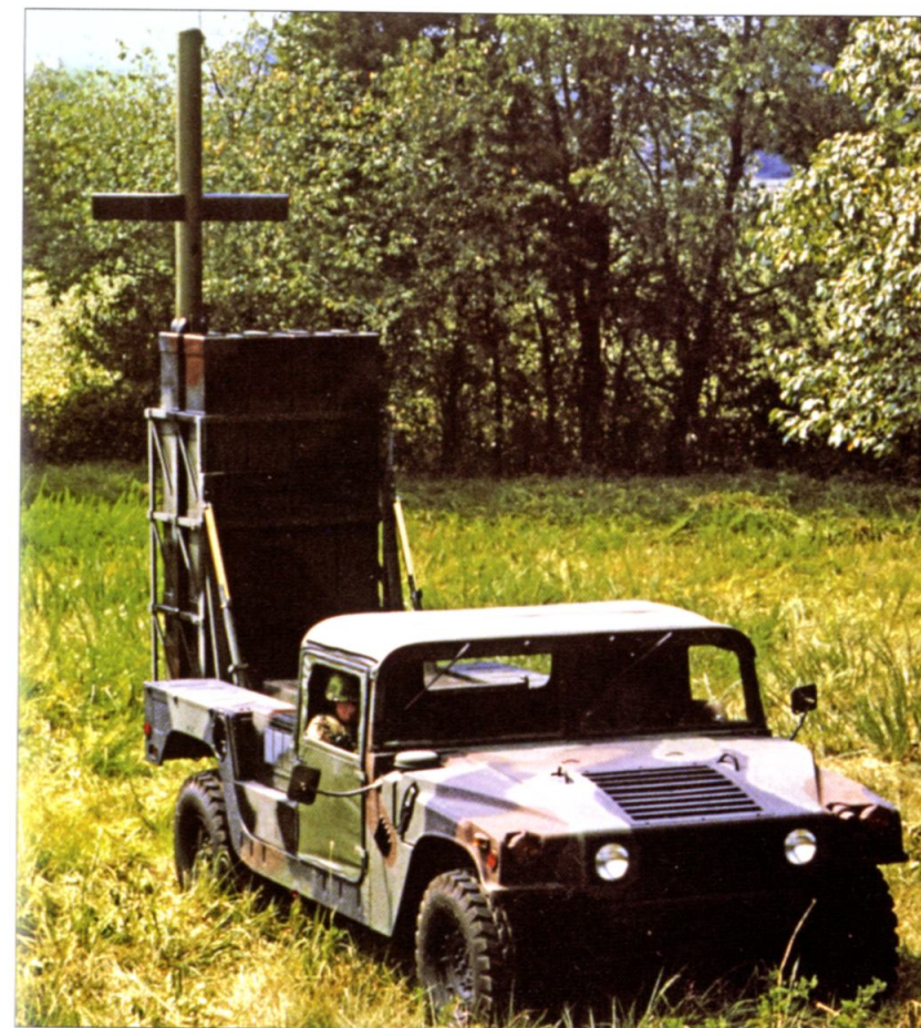
The MGM-157 EFOG-M was an effort to exploit novel fiber-optic guidance for a vertical-launch precision attack missile. It was canceled in 1999, but the concept re-emerged a few years later as Netfires. (Raytheon)
