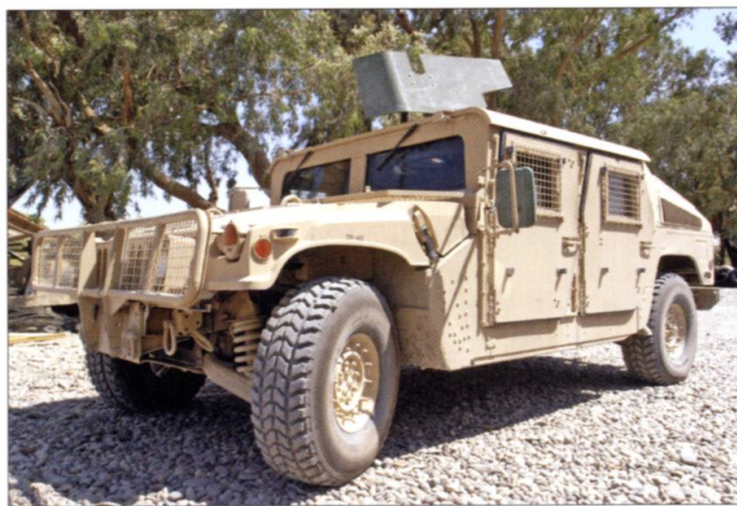
As an interim solution until their own Add-On-Armor kits became available, some Marine units in Iraq received M1114 UAHs from the Army or M1116s from the Air Force, like this M1114 serving with the 2/4th Marines in June 2004.
