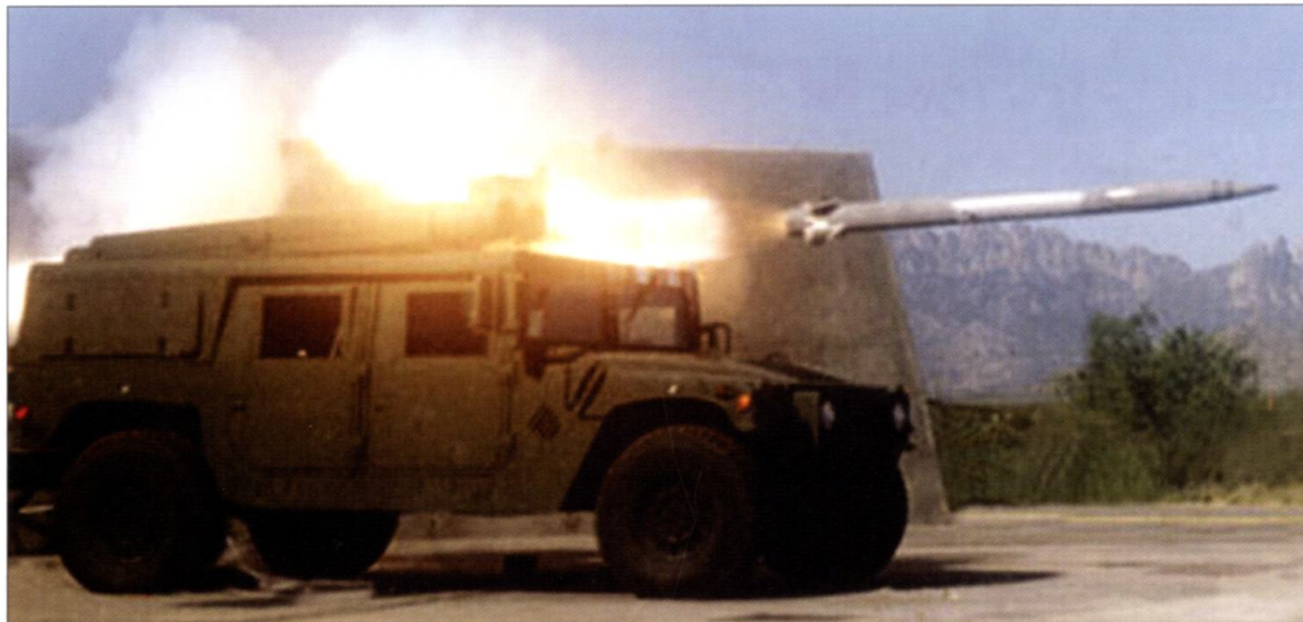
The MGM-166A LOSAT is a hypervelocity antitank missile that penetrates the thickest tank armor by sheer speed rather than high-explosive punch. It was built in small numbers for use by rapid-entry units to provide some highly mobile firepower during contingency operations until heavy forces arrive. (Lockheed Martin)
