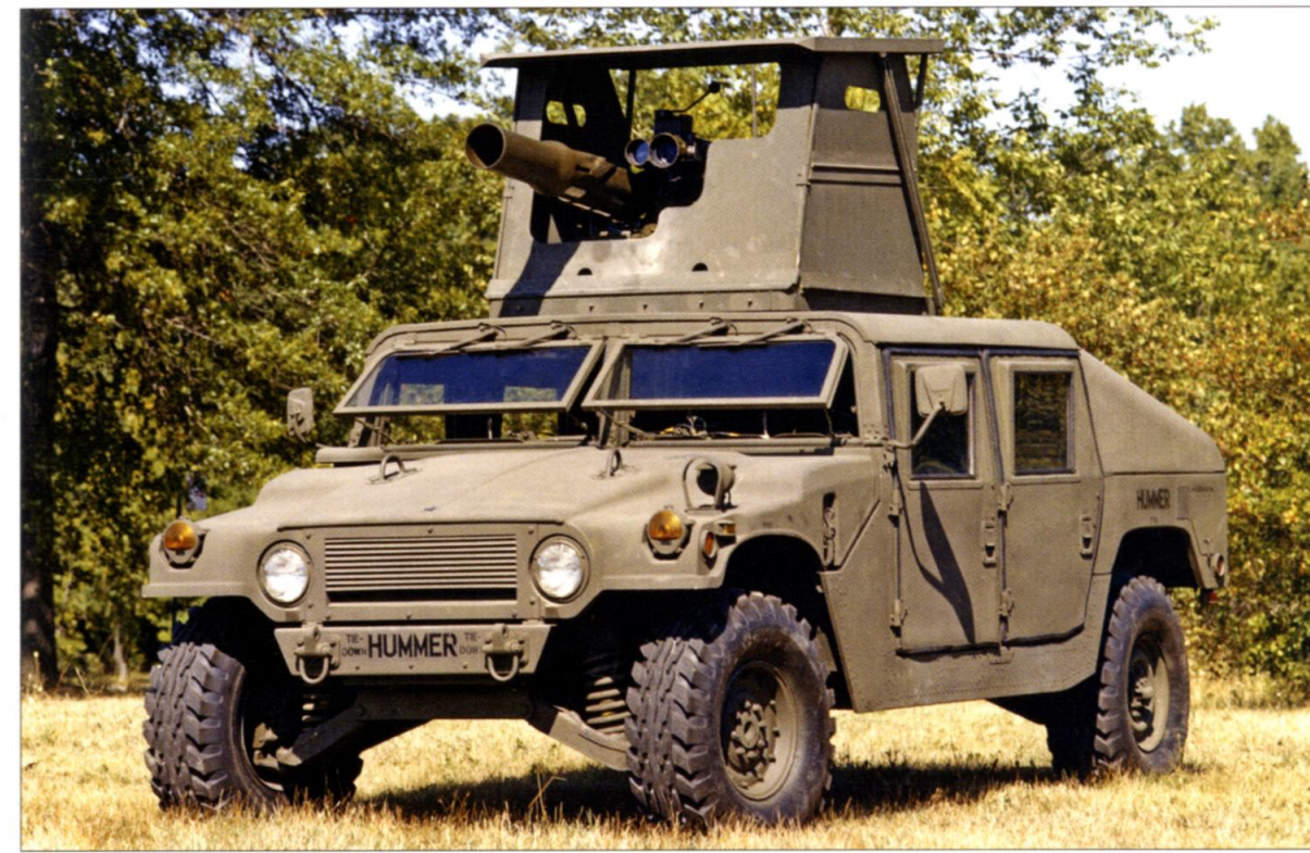
The initial production batch of AM General HMMWVs for the Army tests had a number of differences from the series production versions, such as the slat grille seen here. This TOW carrier also displays the planned Kevlar parapet around the missile launcher, a feature that was subsequently dropped during series production. (AM General)
