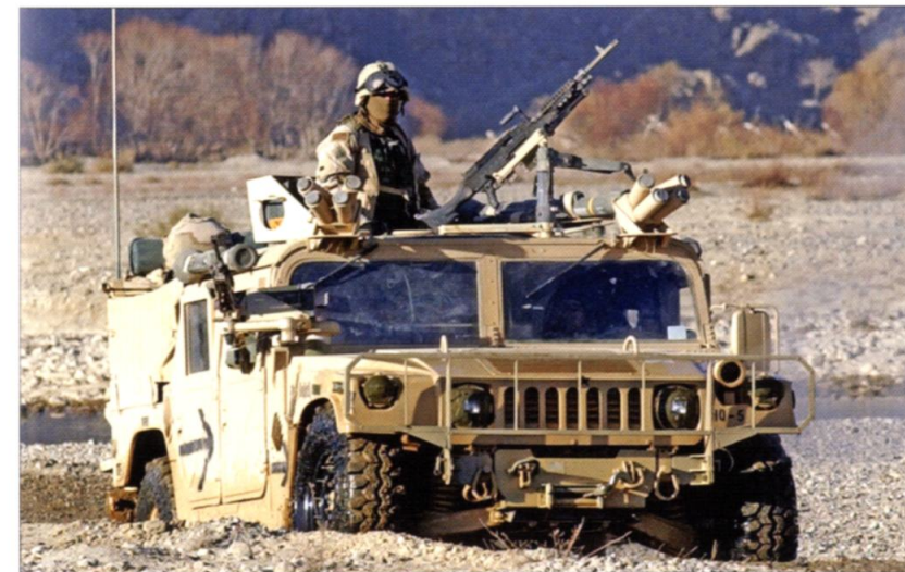
The Dumvee is an M1025 adapted to special operations and can be distinguished by various features such as the passenger-side machine-gun pedestal mount, smoke-grenade launchers, aggressive-pattern tires, and other modifications. This Dumvee is seen in action with the 3d Special Forces Group in the Daychopan region of Afghanistan in January 2004. (Sgt Horace Murray, US Army)
