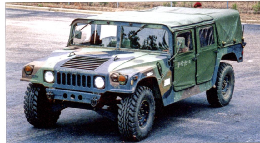
The basic M998 cargo/troop carrier came in several configurations, including this soft-top, four-door version seen here with the 82d Airborne Division in 1992. The related M1038 is essentially the same except for a winch mounted in the front under the radiator. (Author)
