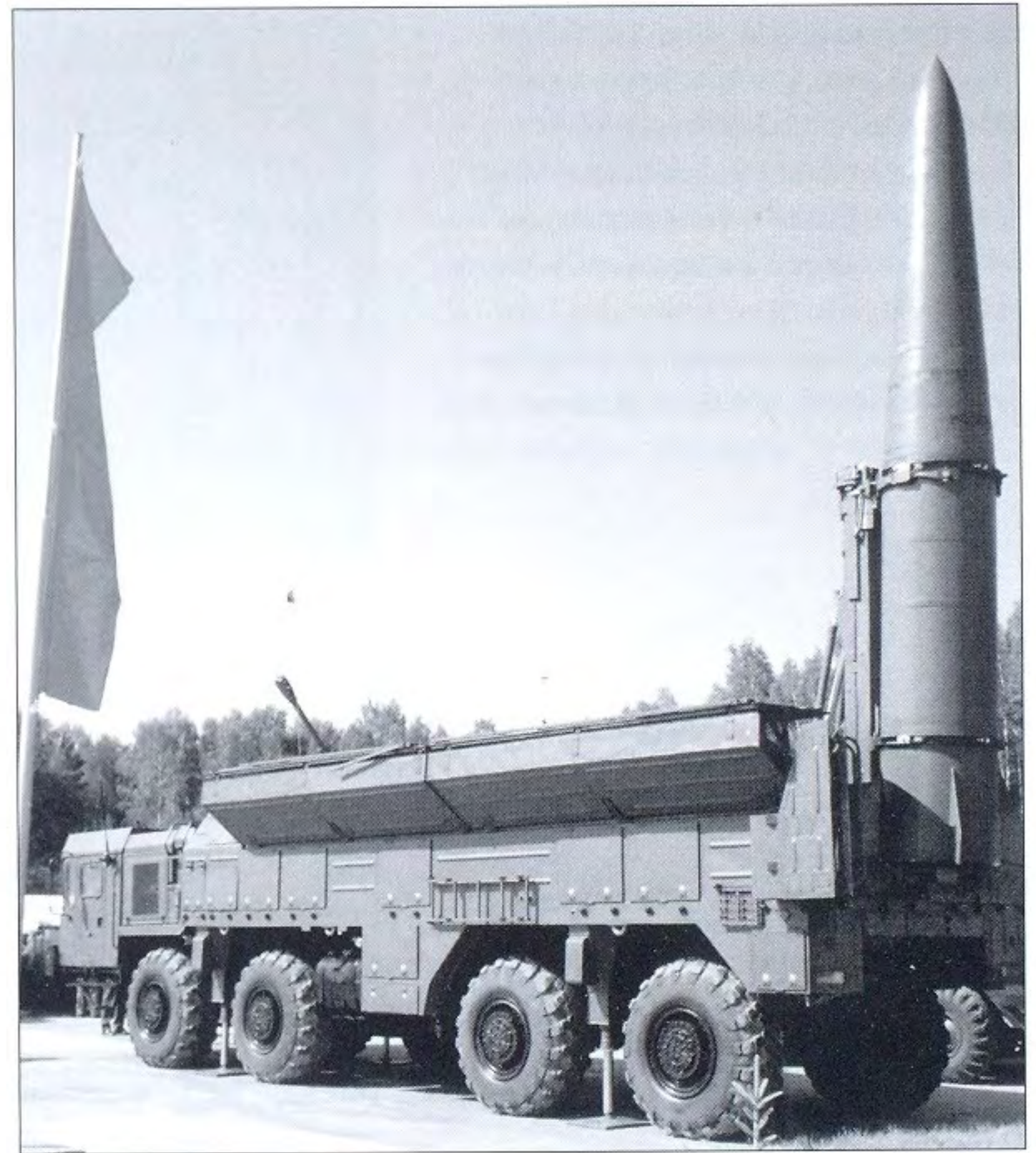
This rear view of the 9P78-1 TEL of the Iskander system shows one of its solid-fuel ballistic missiles in the erected launch position. (Author)
