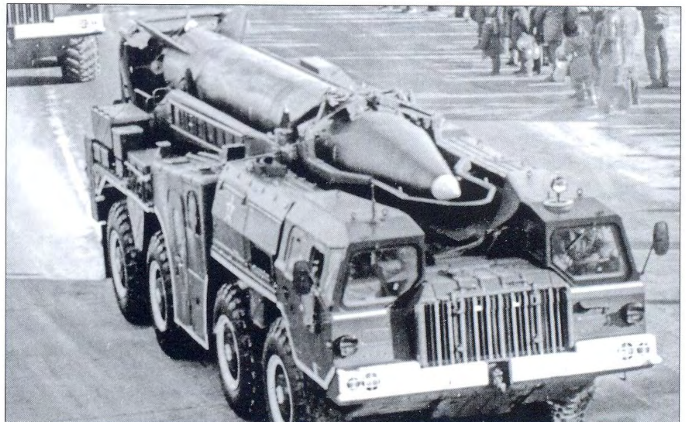
The 8K72 Elbrus tactical ballistic missile system, better known in the West as the SS-1c Scud B, was developed in the 1960s to deliver tactical nuclear warheads. It gained notoriety during its use in regional conflicts in the 1980s and 1990s. (US DOD)
