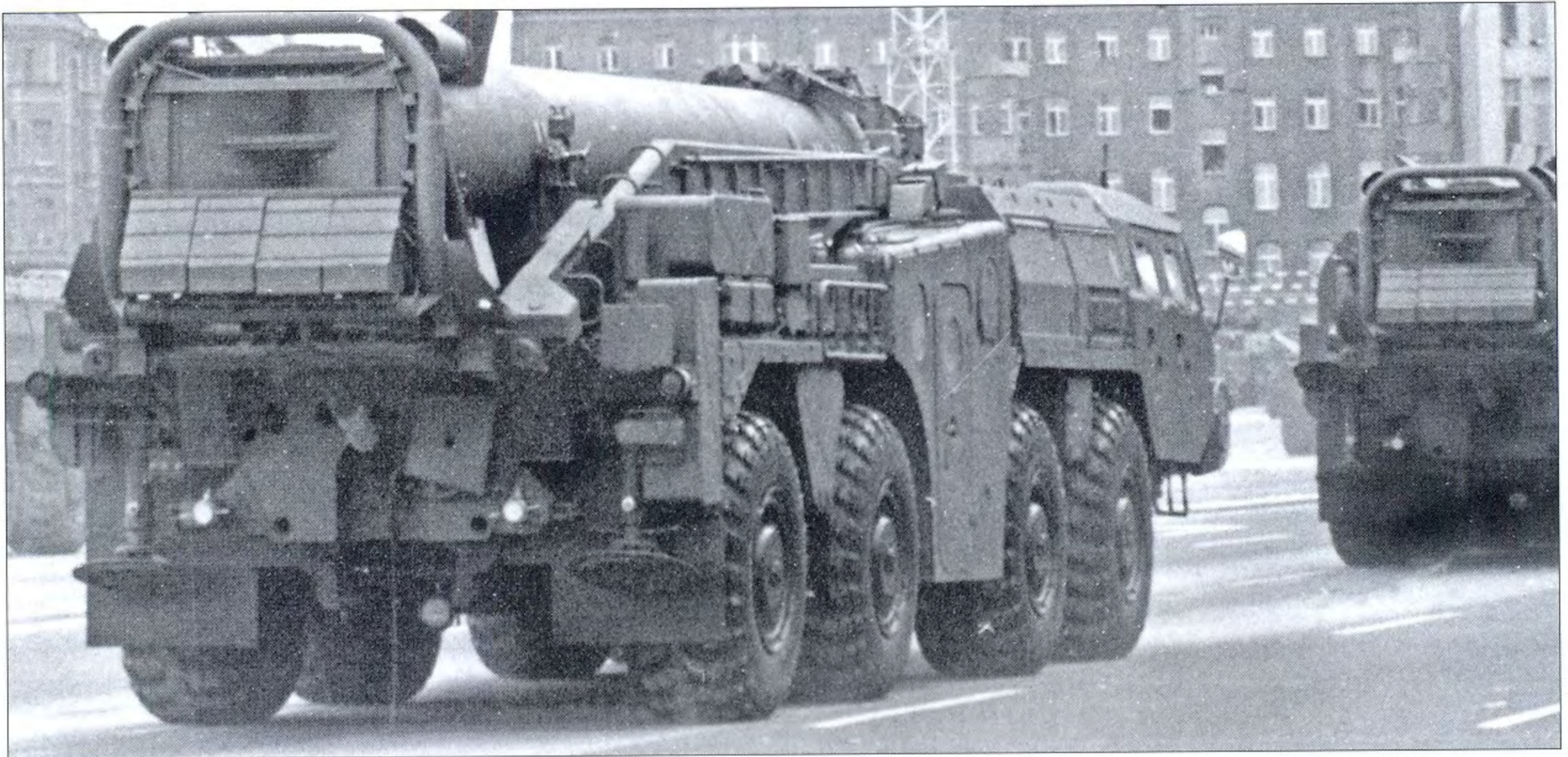
ABOVE Another view of an East German 9P117M TEL from the initial production series with the two portholes on the center-right pumping cabin. (US DOD)
