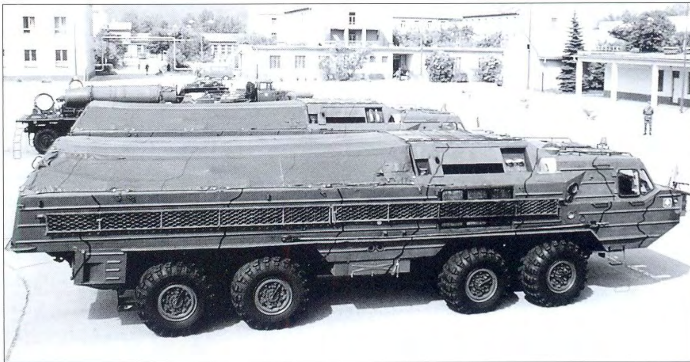
The 9T230 transloader is used to re-supply the 9P71 Oka TEL. It closely resembles the 9P71 TEL, since they are both based on the same BAZ-6950 Osnova heavy-truck chassis. The transloader can be distinguished from the launcher vehicle by the canvas tarp over the rear bed of the vehicle. (Miroslav Gyurosi)
