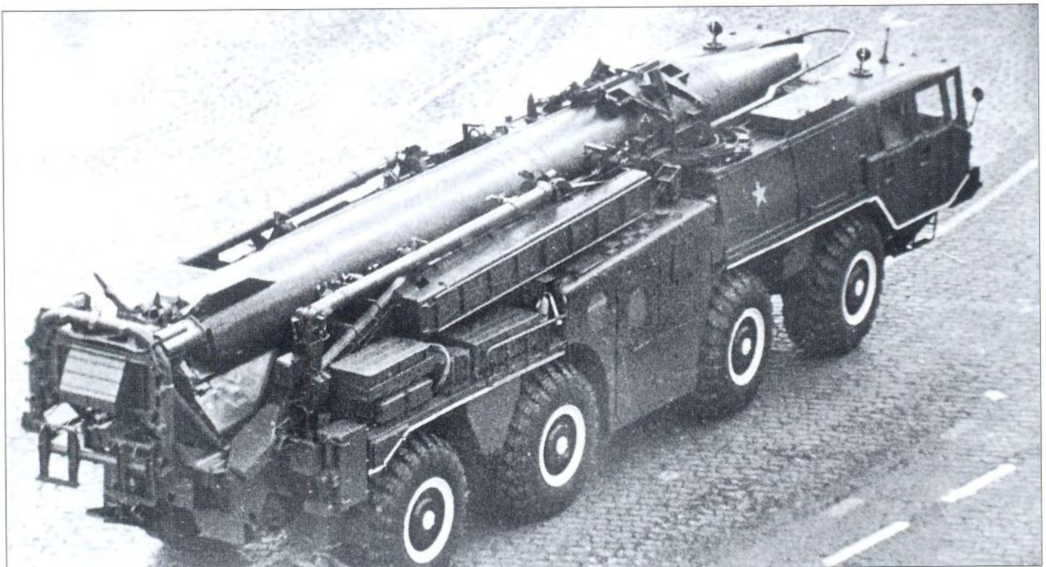
BELOW The initial version of the 9P117 TEL had a heavier erector assembly than the subsequent 9P117M series with self-loading features. This feature is evident in the large hydraulic actuators and box structure on the erector side seen in this overhead view. (US DOD)
