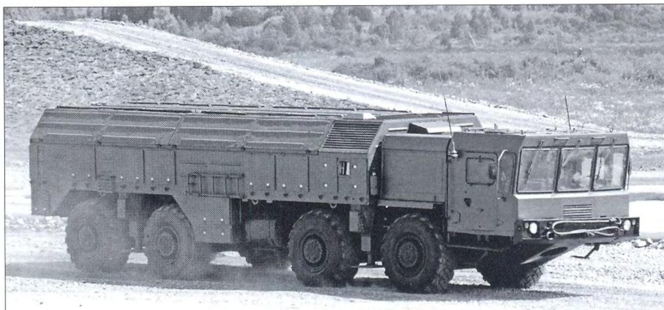
Unlike the 9P117 used with the Scud, the new 9P78-1 TEL used with the Iskander/Tender fully encloses the missile during transit, as seen here on this Russian vehicle at the Staratel artillery proving ground near Nizhni Tagil. (Author)
