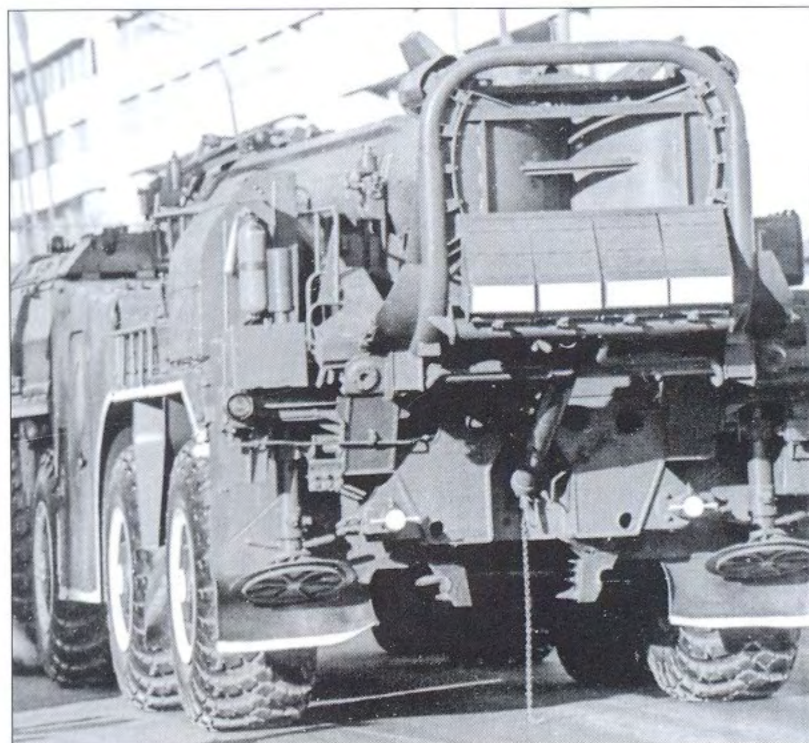
This rear view of a Soviet 9P117M1 TEL clearly shows the large 9N117 launch pad, which folds up behind the missile during transit. (US DOD)
