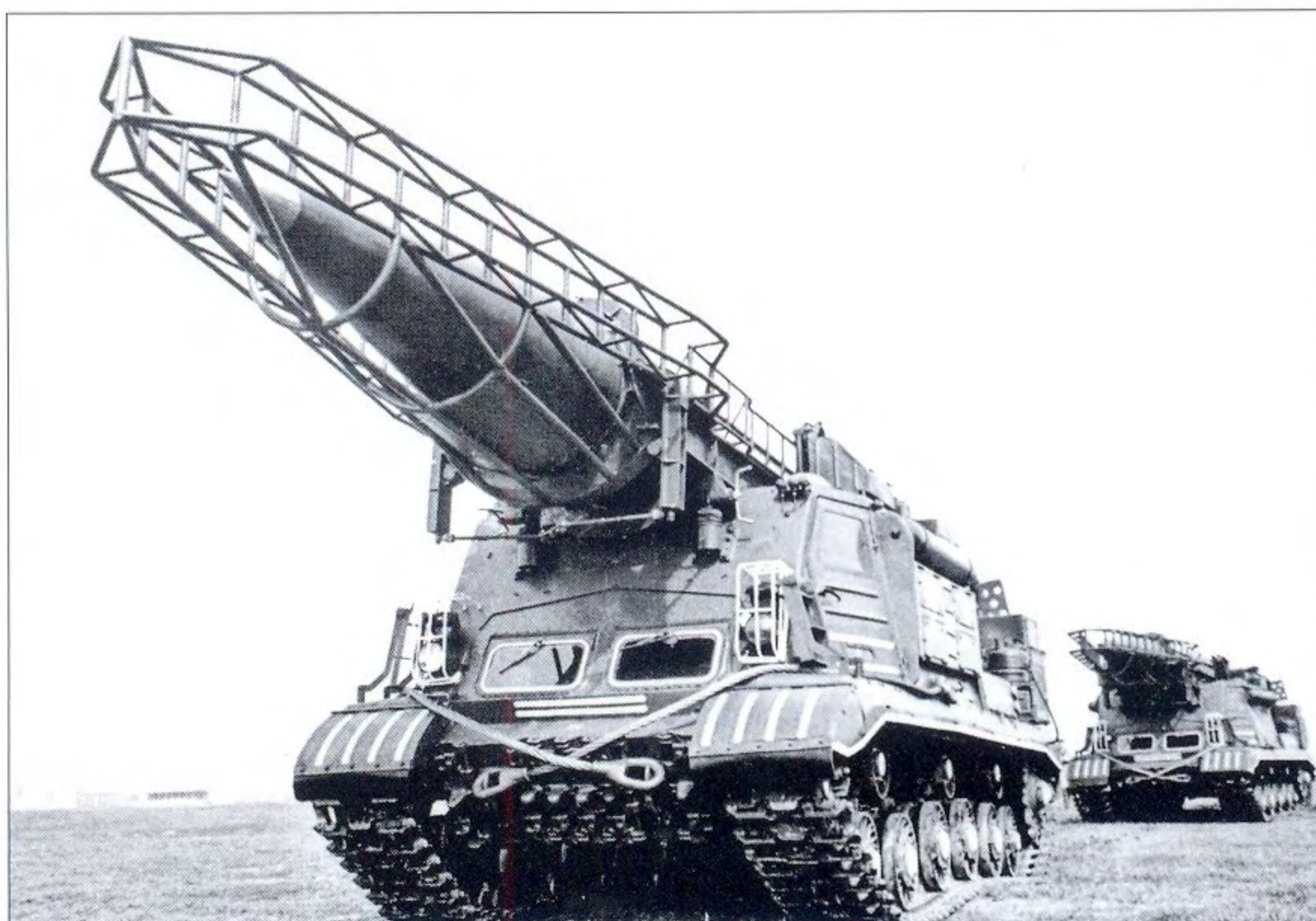
The standard R-11M was launched from the 8U218 TEL, based on the ISU-152K assault gun. The 8K11 (Scud A) can be distinguished from the later 8K14 (Scud B) 2P19 TEL by the presence of a single air pressure cylinder on the side superstructure.
