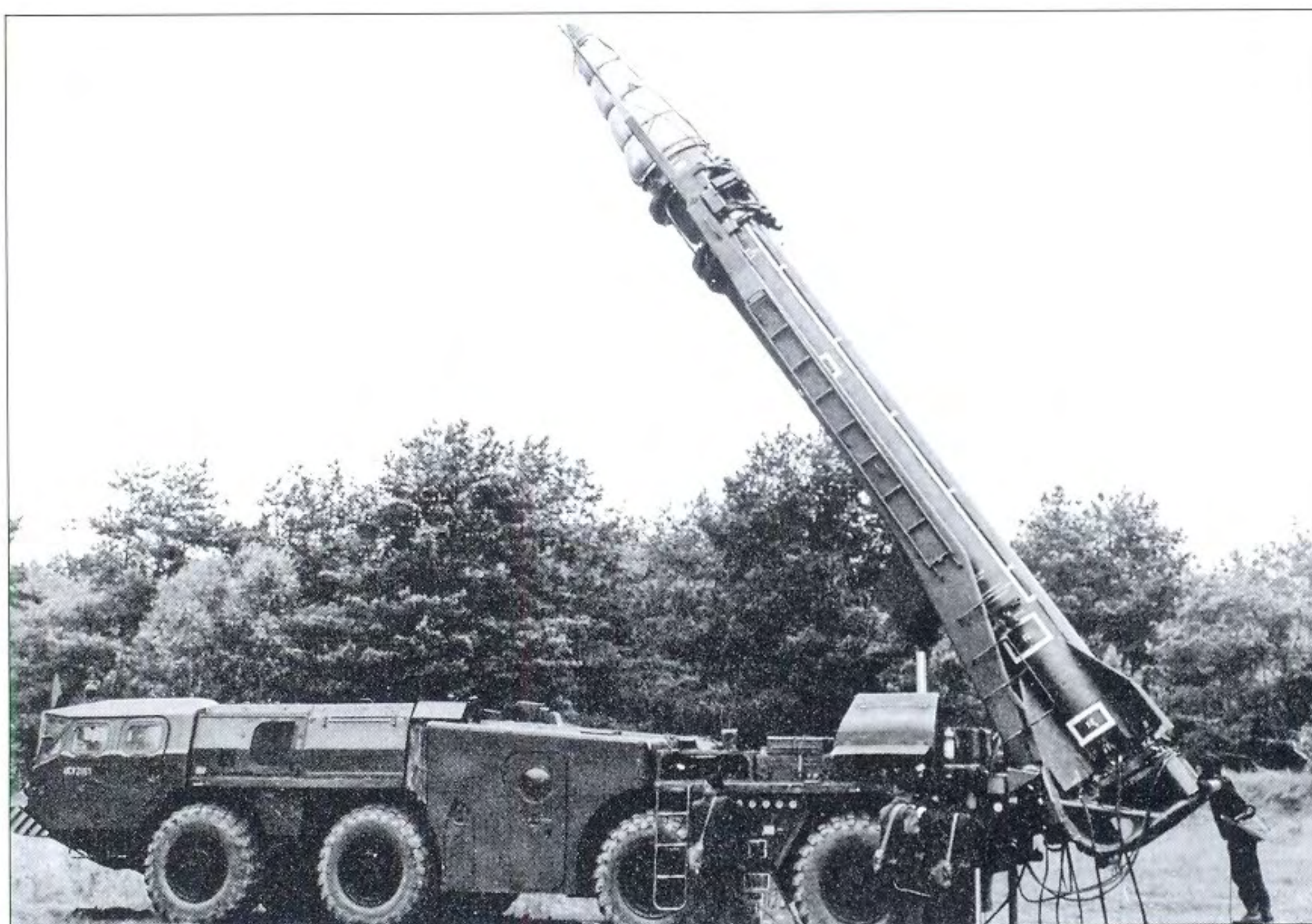
The 9P117M1 TEL used a new power plant and engine with different radiator venting, as seen on this Polish TEL. The 2Sh2 thermal insulating blanket on the warhead is electrically warmed to maintain the nuclear warhead's temperature, and is removed shortly before launch. (W. Luczak)
