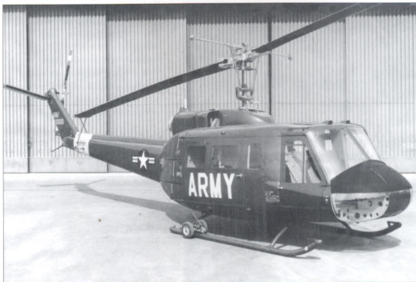
The HU-1D was the first of a new and enlarged series of Bell helicopters, the Model 205. Larger than the preceding Model 204, the new variant first flew in August 1961. By the time it entered service in 1963, the Huey's designation had been changed to UH-1.
