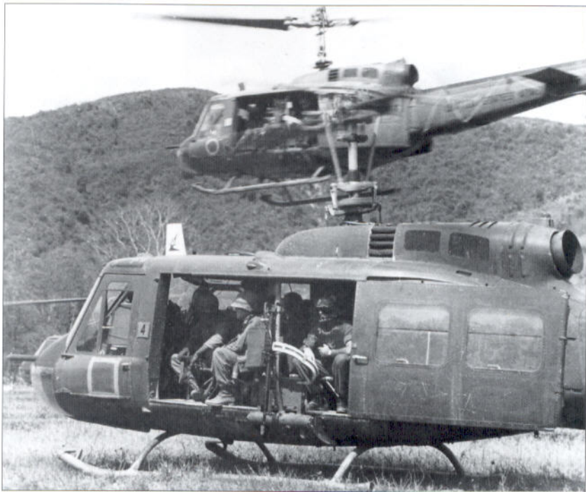
A pair of UH-1Ds lift off from a landing zone after picking up an infantry patrol. The larger D model Huey is easy to distinguish from earlier variants; apart from the longer body, the doors have two windows rather than one.
