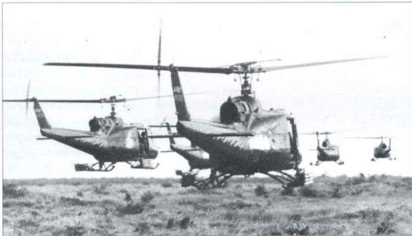
The first non-medical Hueys in Vietnam were assigned to transport companies, but many, like these UH-1As, were fitted with weapons to fly support missions for Piasecki H-21 transport helicopters. However, Hueys quickly took over the transport role as well.
