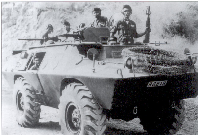
Detail shot of the lead V-100 in a convoy, clearly showing a rear tripod-mounted machine gun, the commander's M79 grenade launcher, and the twin M37 or M1919A4 machine guns. This vehicle like all the others in the convoy carry the barbed wire for crew protection during bivouacs at night. (Copyright Cadillac Gage Textron Inc.)
