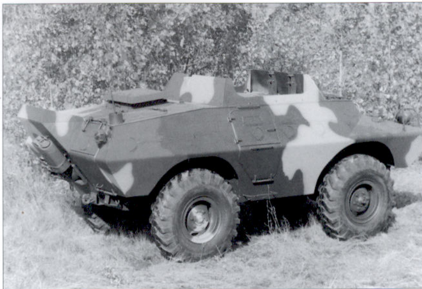
A freshly painted US Air Force V-100 illustrated against a woodland backdrop. USAF V-100s served as a mobile strongpoint and arms carrier for responding to intrusions and enemy attacks on air bases in Vietnam and Thailand. (Copyright Cadillac Gage Textron Inc.)
