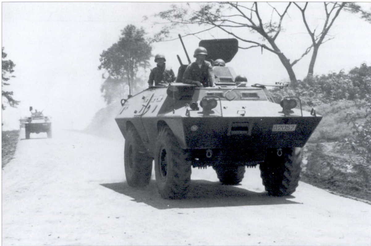
Two V-100s patrolling along a road. The yellow lettered "TC" within a red circle signifies that this is a V-100 belonging to an ARVN cavalry unit. These two V-100s are armed with a combination-mount, consisting of a .30 M37 or M1919A4 machine gun and a .50 M2 machine gun. (Copyright Cadillac Gage Textron Inc.)
