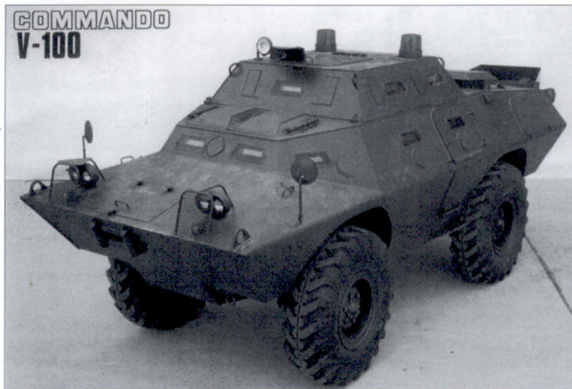
A late-production V-100 Emergency Response Vehicle with a raised center section. The elongated slots in the raised section allowed better elevation for the firing of tear gas guns into riots and crowds. (Copyright Cadillac Gage Textron Inc.)
