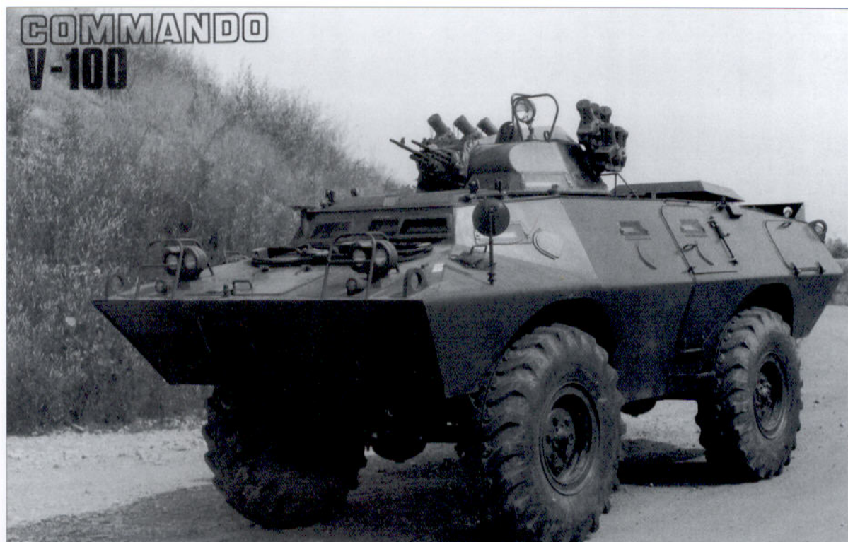
BELOW Final version of the V-100 pictured at the factory in the early 1970s. Lessons learned from Vietnam have been incorporated into the final version, which incorporates twin M60 machine guns. The final model also offered Wegmann grenade launchers, a spotlight, twin vision blocks for additional visibility for the driver, and a towing cable stored on the nose of the vehicle. The revised headlight guards, which were intended to cut down on glare, and the revised covers for the fuel tanks are also all visible on this model. (Copyright Cadillac Gage Textron Inc.)
