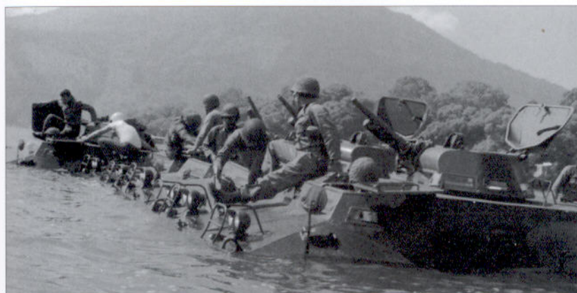
A line of V-100s undergoing fording training in Lake Atmalan, Guatemala. The top-mounted air intake and exhaust, along with seals around the doors, made fording operations possible without any preparations.
