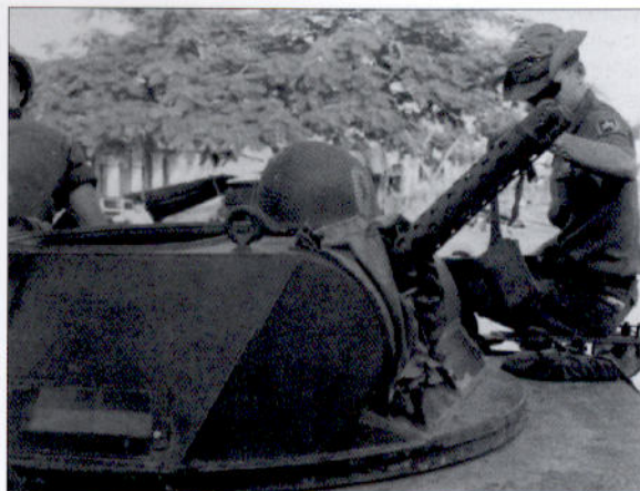
Detail of the twin M37 or M1919A4 .30-caliber machine guns mounted on the T-50 turret. This is a later turret, as the earlier models had a narrower vision block in the front to compensate for the width of the .30 M37/.50 M2 machine gun mount.
