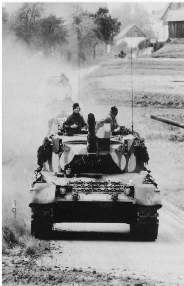
Leopard 1A3 with the protective screens for the TEM 1A stereoscopic/coincidence sights – slid open. Camouflage is enhanced with bands and splotches of mud. (MaK System)
