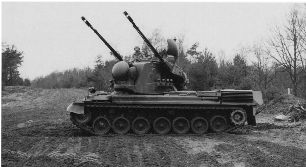
Manned and ready, this Flakpanzer 1 Gepard A1 has the hatch open and the tracking radar swung round in the operating position. The exhaust for the APU runs along the left side of the hull. (Michael Jerchel)
