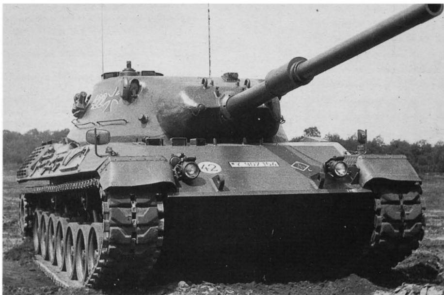
One of the 50 pre-series vehicles seen during trials at Munster. The 'O series' re-introduced the optical rangefinder, but still had only a rectangular hatch at the loader's station and used the old rhomb style of tactical marking on the glacis. The tactical marking assumed the familiar rectangular style on introduction of the series vehicle (1st batch). (Archiv Laber)
