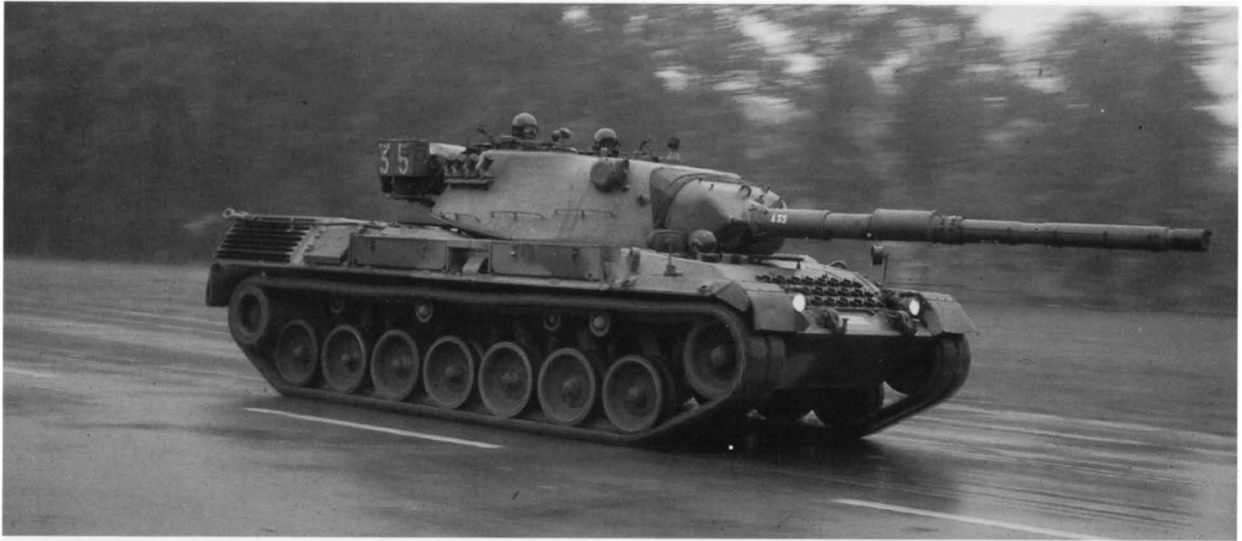
Leopard 1 BE of the 4th BN Lanciers at speed on the ring road near range 9, Bergen, in 1993. Between the two storage boxes at the side of the hull is the exhaust for the diesel driven heating system – most welcome in winter! (Michael Jerchel)
