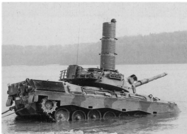
This Leopard 1A2A1 of PzBtl. 184 is fitted with a snorkel (mounted on the commander's cupola) for deep fording up to a depth of 4 m. (Michael Jerchel)
