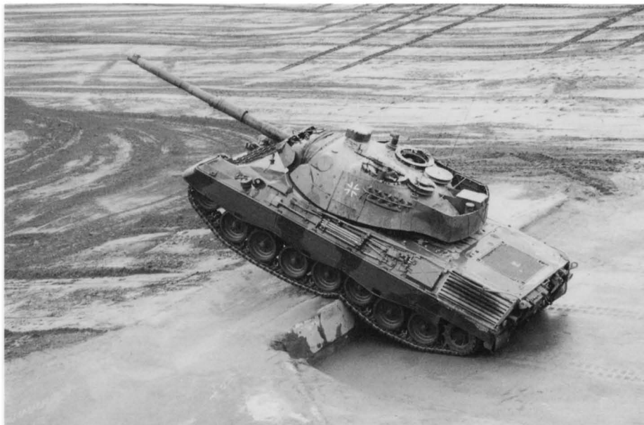
A Leopard 1A5A1 (former 4th batch) negotiates an obstacle. The Leopard can climb over vertical obstacles up to 1.15 m high and cross trenches up to 2.5 m wide. (Michael Jerchel)
