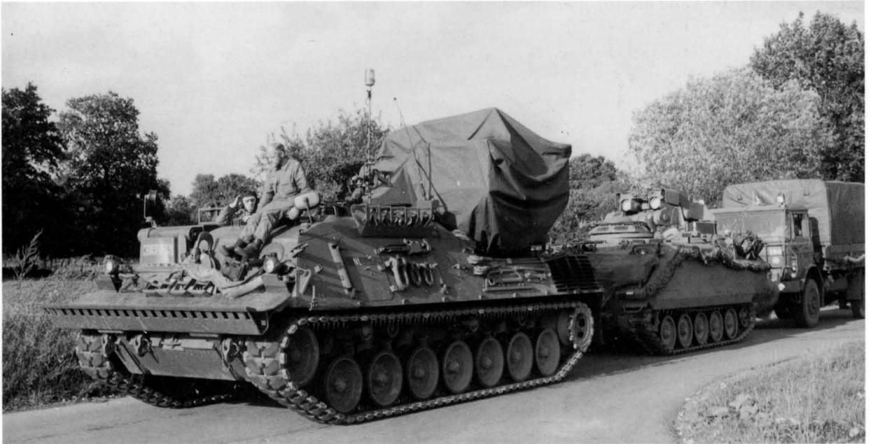
Dutch Bergingstank ARV with a YPR-765 PRAT in tow and a spare engine (protected by a tarpaulin) on the engine deck. The Dutch version of the Leopard ARV, seen
