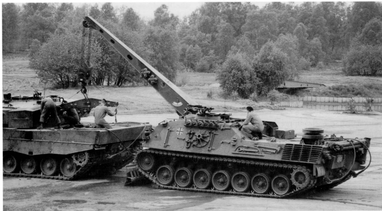
Bergepanzer 2A2 ARV in the process of changing the powerpack of a Leopard 2A4 MBT. The base plate for the support struts at the rear is stored on the left side of the hull,
