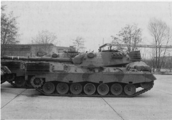
This depot view of a Leopard 1A2A1 shows the camouflage pattern introduced in 1985. The Leopard 1A2A1 has oval outer panels over the optical sight heads, unlike the circular covers fitted to the first to fourth batches. The power socket for the searchlight is located between the optical head and the national emblem. (Thomas Laber)
