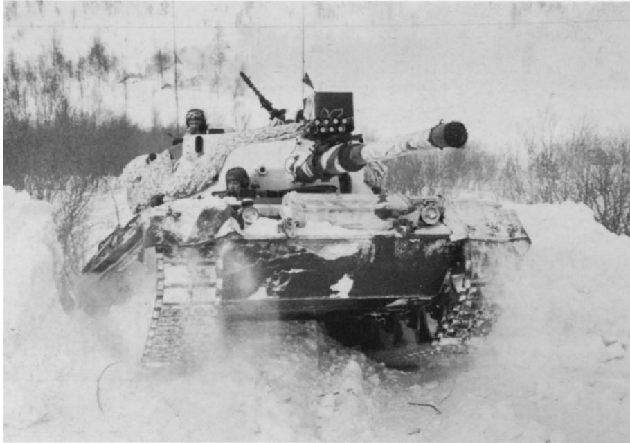
Like most Norwegian Leopards, this snow white example has an extra storage box on the upper glacis plate. A gunfire simulator is mounted on the gun barrel. (Norwegian MoD)
