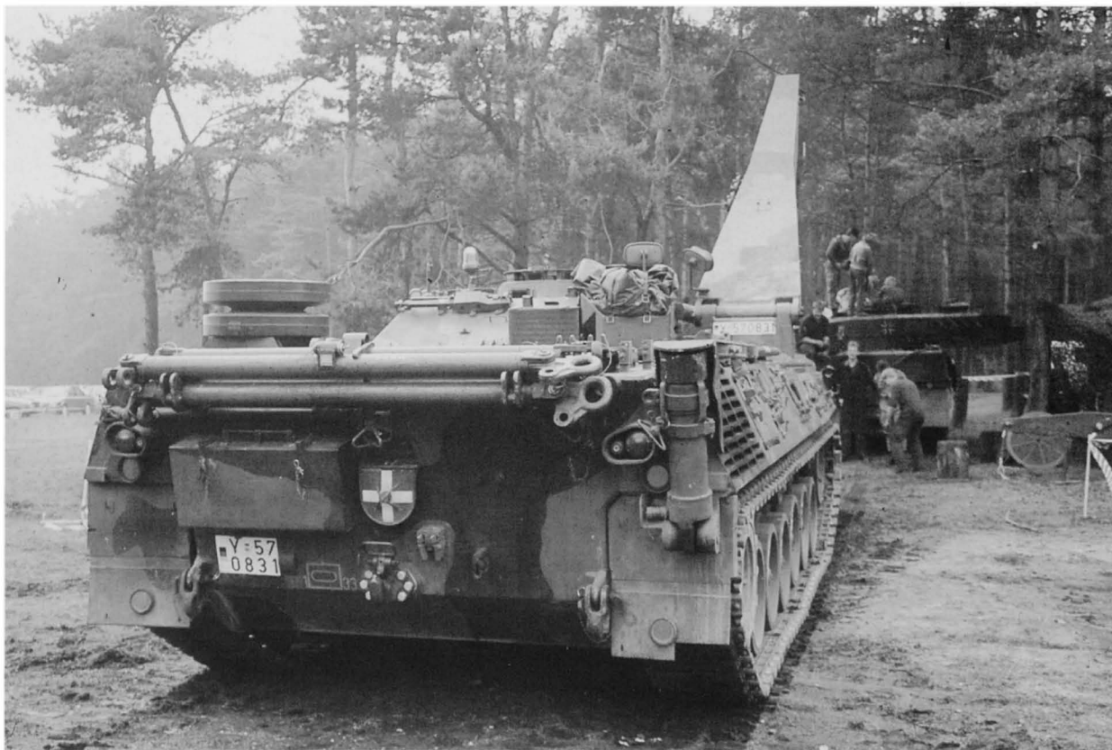
The improved Leopard ARV, Bergepanzer 2A2, incorporates support struts, seen here in the travelling position on this vehicle of Panzerbataillon 33. (Michael Jerchel)
