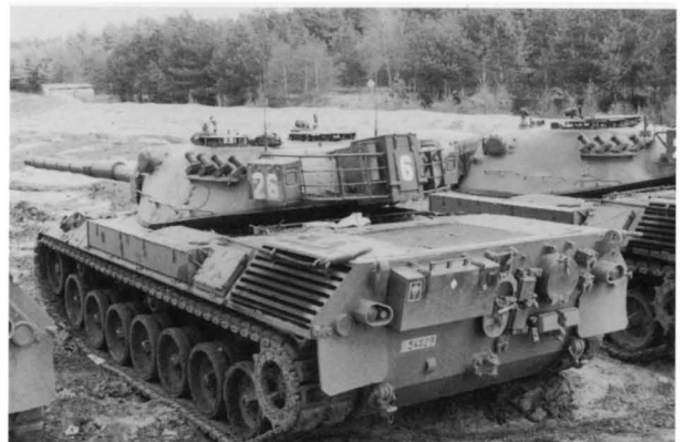
Rear quarter view of a Belgian Leopard 1 BE taken at Bergen in 1989, displaying its external similarity to German 4th batch vehicles. Ammunition boxes have been added to the turret basket for extra storage space. (Michael Jerchel)
