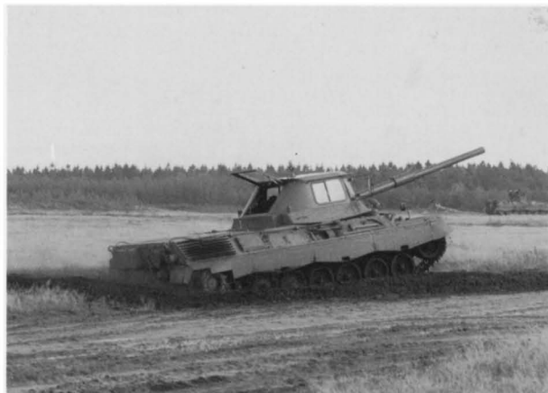
A Leopard 1 driver training tank travelling across country. The turret is replaced by an observation cabin with dual controls, a dummy gun barrel ensuring that the trainee driver is fully aware of the vehicle's overall dimensions. (Sabine Rotter)
