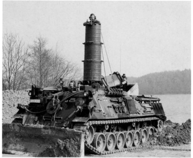
Pionierpanzer 2 Dach ACEV fitted with a deep wading snorkel, allowing it to work in the water to a max. depth of 2.25 m. The remote control set may be seen in front of the commander, standing in the snorkel. (Michael Jerchel)
