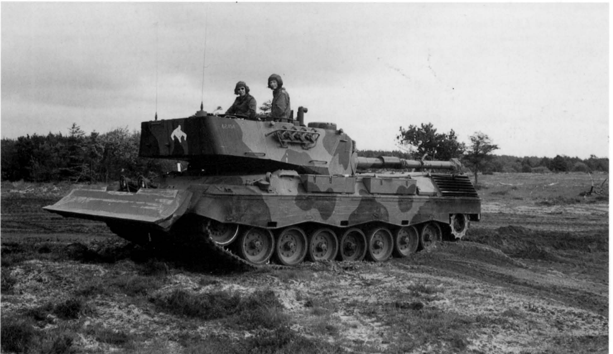
All Danish Leopard 1 MBTs are modified to carry either the dozer blade or Tracked Width Mine Plough (TWMP).
