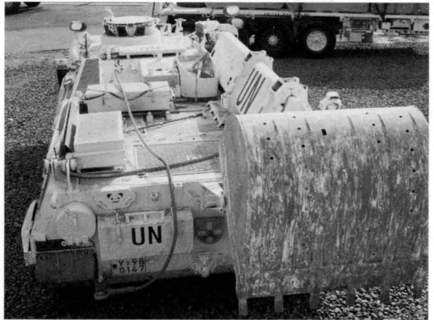
Included in the German UNOSOM in Somalia were two Pionierpanzer 2 Dach ACEVs; this one was photographed on return to Emden. (Michael Jerchel)
