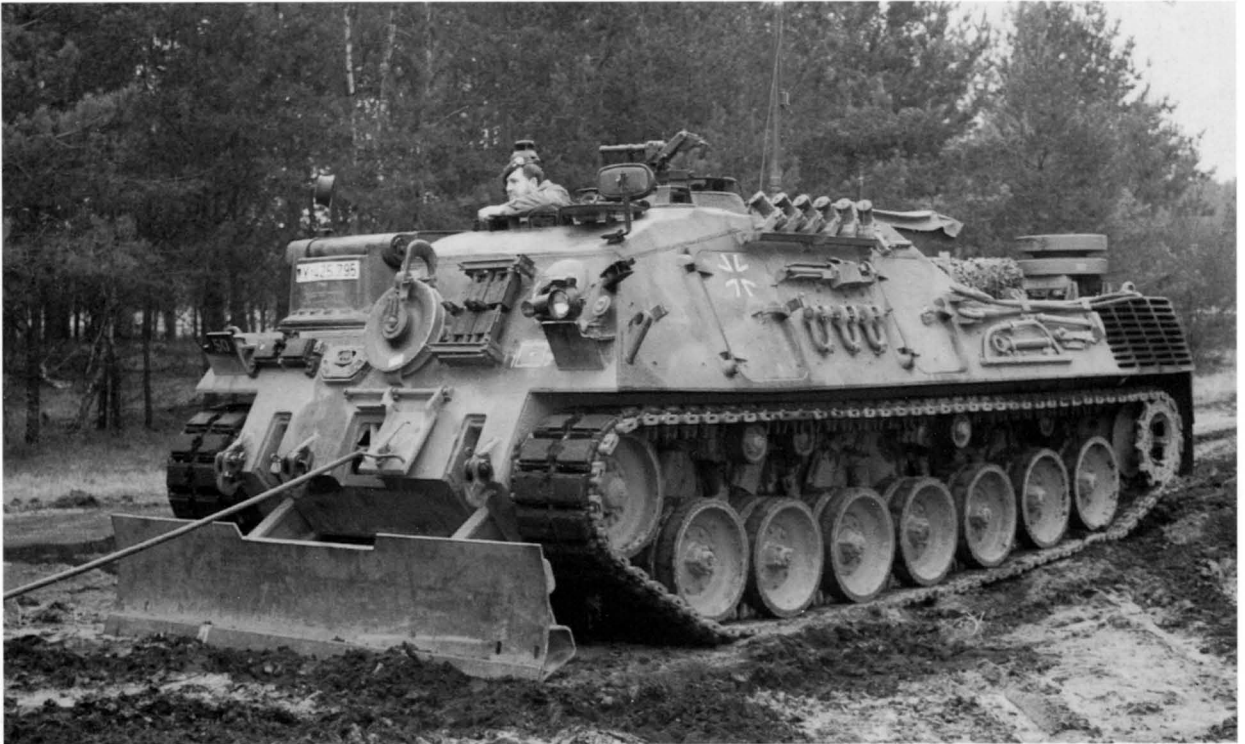
Bergepanzer 2 Standard ARV during winching operations, for which a cable emerges through the aperture provided, covered by a sliding door opening to the left, as seen here.
