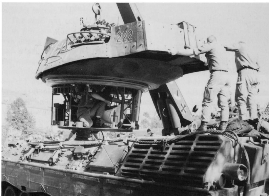
The first two batches of the Leopard 1 were delivered without hookeyes, but as an interim measure they were added to the vehicle's rear, as revealed by this Leopard 1A1A1 having its turret removed by a Bergepanzer 2. (Michael Jerchel)
