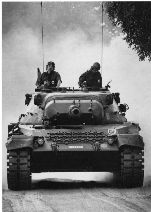
Head-on view of a Belgian Leopard 1 BE going downrange during the CAT 89 NATO tank gunnery competition. The crosswind velocity sensor of the SABCA FCS is clearly visible on the turret roof. (P-Info NORTHAG)
