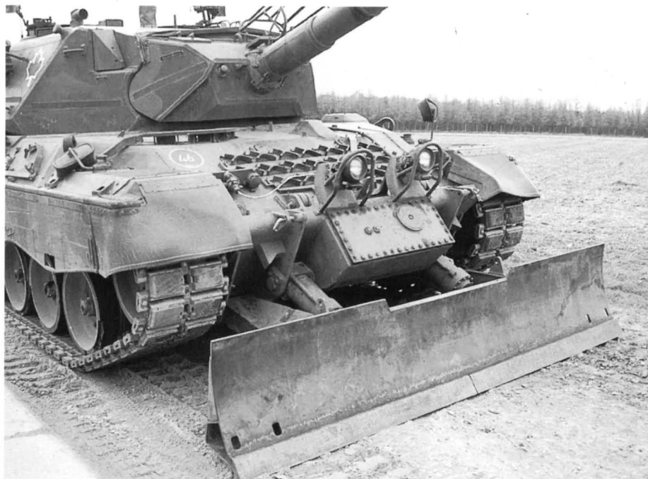
Hydraulic dozer blades were issued to one tank per armoured squadron in the 4th CMBG. When the dozer blade is mounted, the headlights have to be repositioned. (Michael Jerchel)
