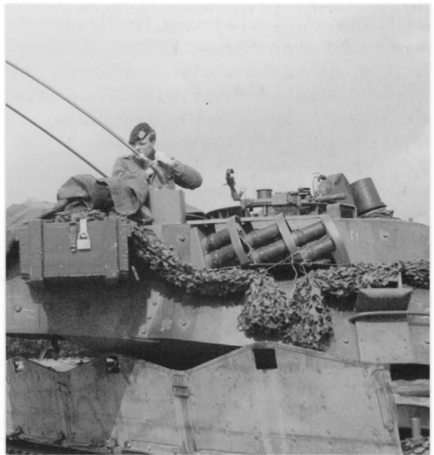
This close up of a Leopard 1 V turret shows the Dutch smoke dispensing system to either side and the US style antenna sockets, the two chocks for which are stowed in the turret guard rails. (Michael Jerchel)
