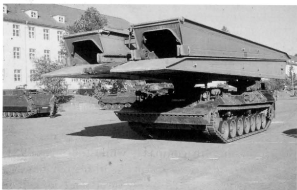
A Brückenpanzer 'Biber' of Pz.Co. 40, showing the two 11m halves of the bridge to good advantage. (M.Jerchel)
