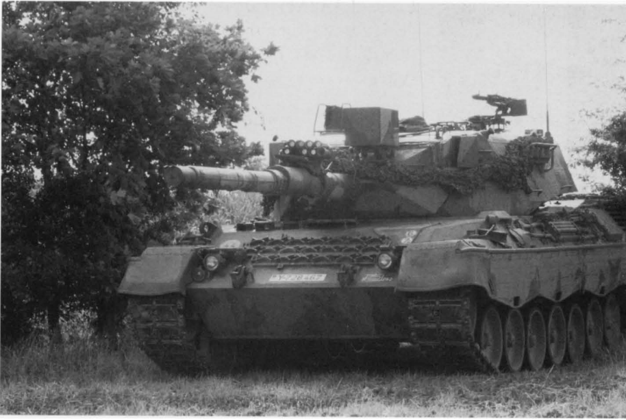
Leopard 1A4 of PzBtl. 282 displaying early style markings on the glacis plate and variations of the mud camouflage. The armoured screens for the EMES 12 A1 stereoscopic rangefinder are in the open position and the optical head of the PERI R 12 may be seen between the gunfire simulator on the barrel and searchlight. (MaK System)
