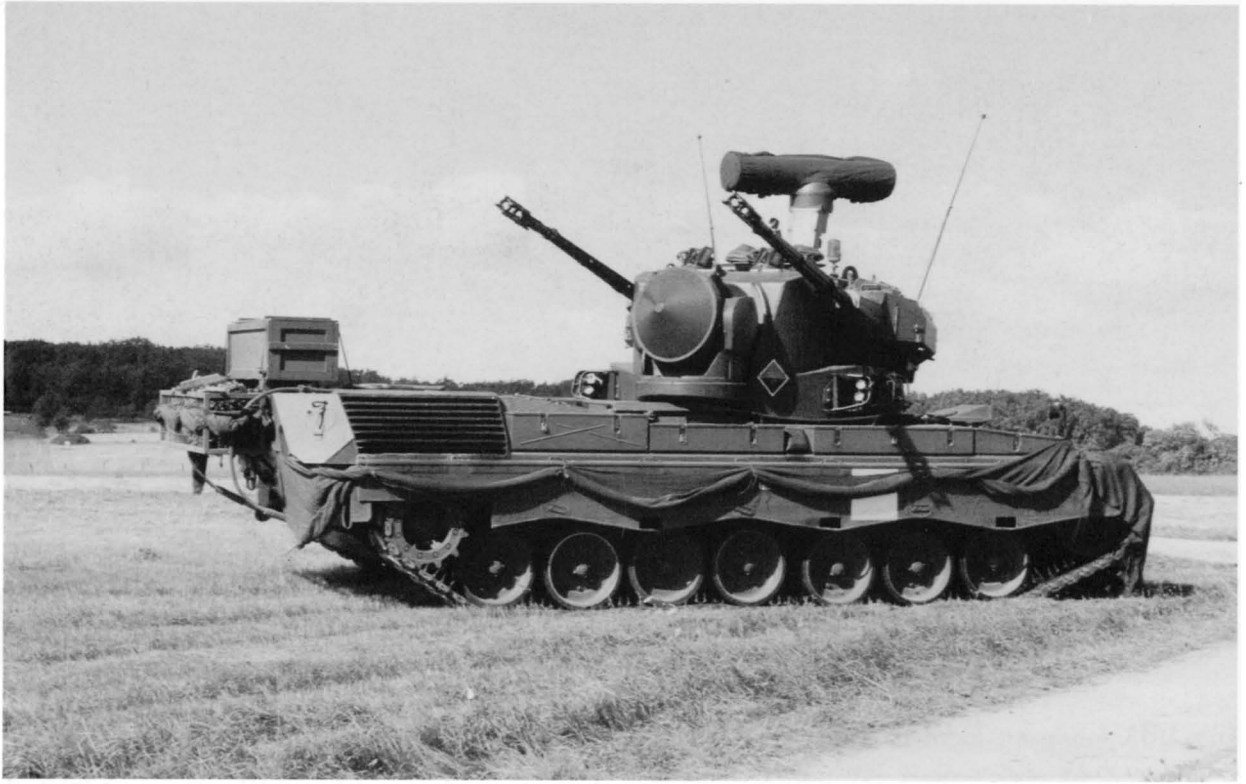
Dutch PRTL SPAAG with tracking radar in operating mode. The PRTL's radar system was produced by Hollandse Signaalapparaten. The PRTL is occasionally referred to as the 'Cheetah', probably due to its company designator, CA1. (Michael Jerchel)
