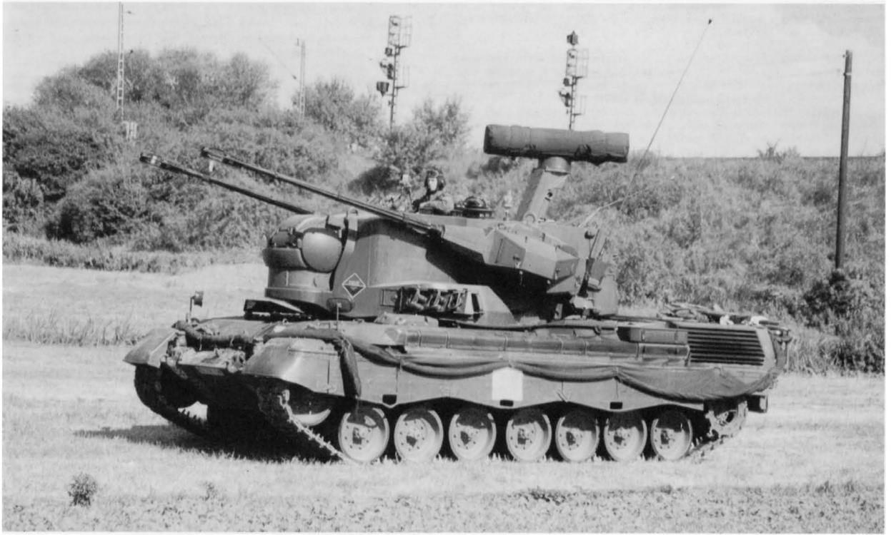
PRTL with tracking radar in stored position, facing the turret front. The HSA surveillance radar is sometimes called the 'dog bone' due to its shape. This PRTL took part in Exercise 'Certain Shield' in September 1991, hence the yellow patch (denoting 'Gold forces') on the side skirts. (Michael Jerchel)
