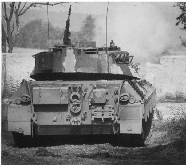
Soon after delivery, the first four batches of the Leopard 1 were modernised to A1 standard. Between 1975-77 these vehicles were further upgraded as Leopard 1A1A1 with add-on turret armour and other changes. This vehicle is from the original 1st batch, recognisable by its square intercom box on the right-hand side of the rear plate. The storage box to the left contains tools. (Michael Jerchel)
