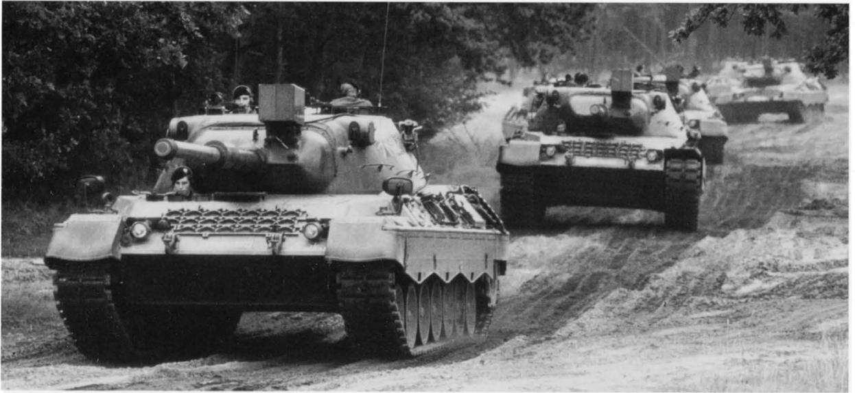
The A1 and A2 are difficult to tell apart, but this is known to be a company of Leopard 1A2 of Panzerlehrbataillon 93 at Munster. As may be seen, these A2s have yet to receive thermal sleeves for their main guns. (MaK System)
