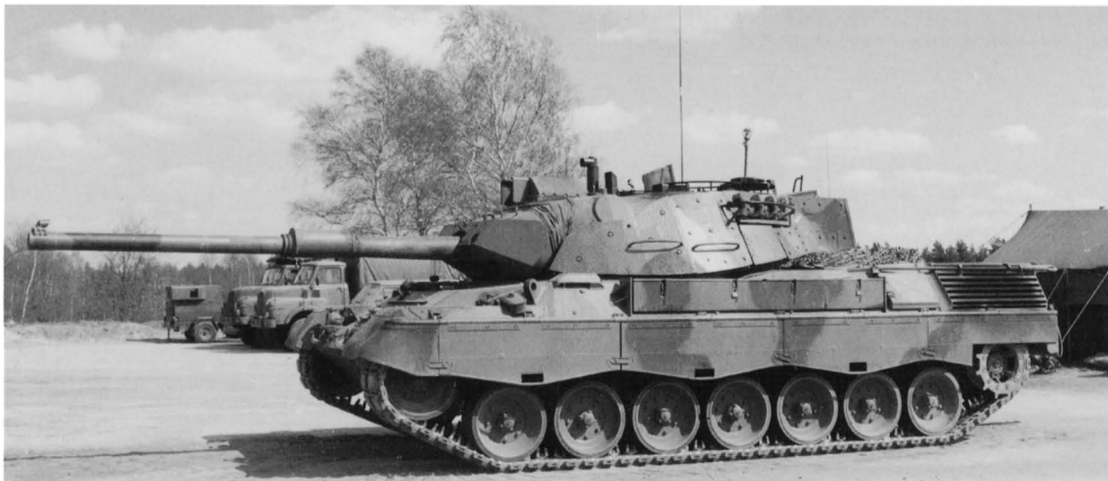
Prototype of the improved Belgian Leopard 1 BE undergoing comparative trials with a German Leopard 1A5 in April 1989. The new FCS includes a thermal day/night
