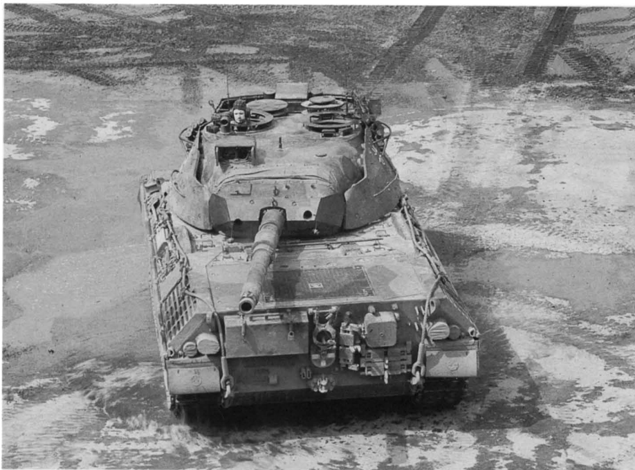
A Leopard 1A5 (former 1st batch) demonstrates its gun stabilisation system, which enables the tank to fire on move with a high degree of first-round hit probability. (Michael Jerchel)
