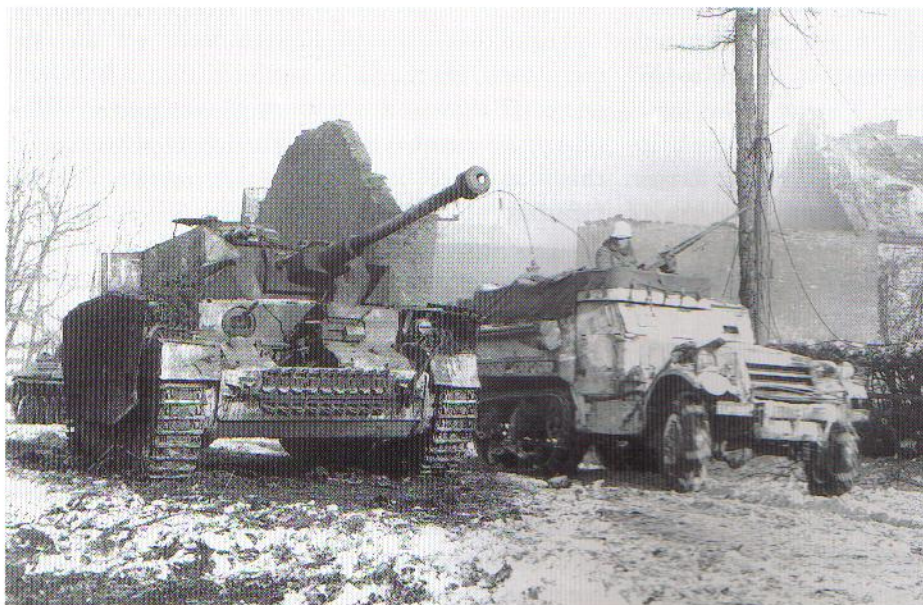
M3A1 carrier of the 6th Armored Division passes by a knocked out German PzKpfw IV in Foy, near Bastogne, in January 1945 during the Battle of the Bulge. This is another rebuilt M3, evident from the use of the old automotive-style headlights. It lacks the usual front bumper, but has been retrofitted with both the M49 ring mount characteristic of the M3A1, and the side mine racks. The front tyres and rubber tracks have been fitted with the usual winter snow chains for better traction. (US Army Signal Corps)
