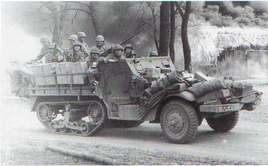
A classic view of the M3 personnel carrier in action with the 46th Armored Infantry, 5th Armored Division near Wittenmoor, Germany, on 12 April 1945. Like most half-tracks in combat for any length of time, it has become encumbered with the crew's equipment. The hull rear is fitted with a luggage rack which was first authorised in September 1943. This particular vehicle is fitted with the winch on front, and a .50cal. machine gun, usually the sign of a platoon leader's vehicle. (US Army Signal Corps)
