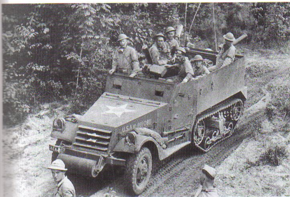
A M2 half-track car of the 14th Field Artillery Regiment during pre-war exercises near Leesville, Louisiana in September 1941. As was often the case with US Army half-tracks, the vehicle is armed far in excess of regulation, with no fewer than three .30cal. Browning water-cooled machine guns. This particular unit used their M2 half-track cars as prime movers for M1897 75mm field guns. Early half-tracks like this one lacked the anti-scuff ring on the front wheels that became standard on later wartime half-tracks. (US Army Signal Corps)
