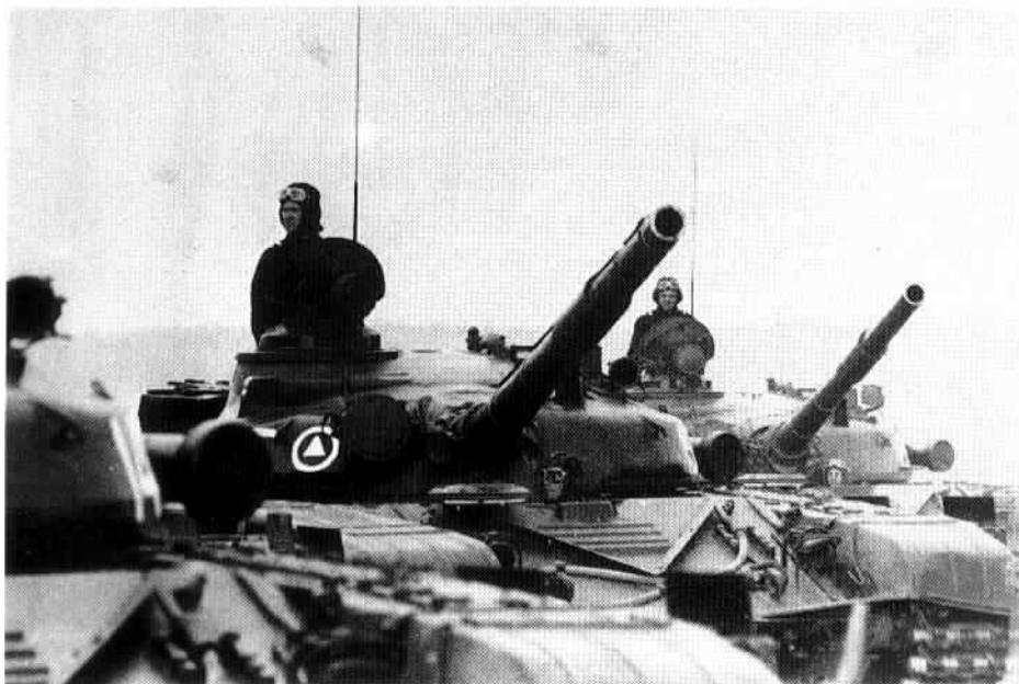
The final production batches of T-72 (Obiekt 172M) Ural tanks had a thickened panel of frontal turret armour, pre-dating the improvement on the T-72A (Obiekt 174). The right coincidence rangefinder port was blocked off, and the improved TPD-K1 laser rangefinder was added. This particular version is very rarely seen and may have served as the pre-series production test-beds for the improved T-72A. (Sovfoto)
