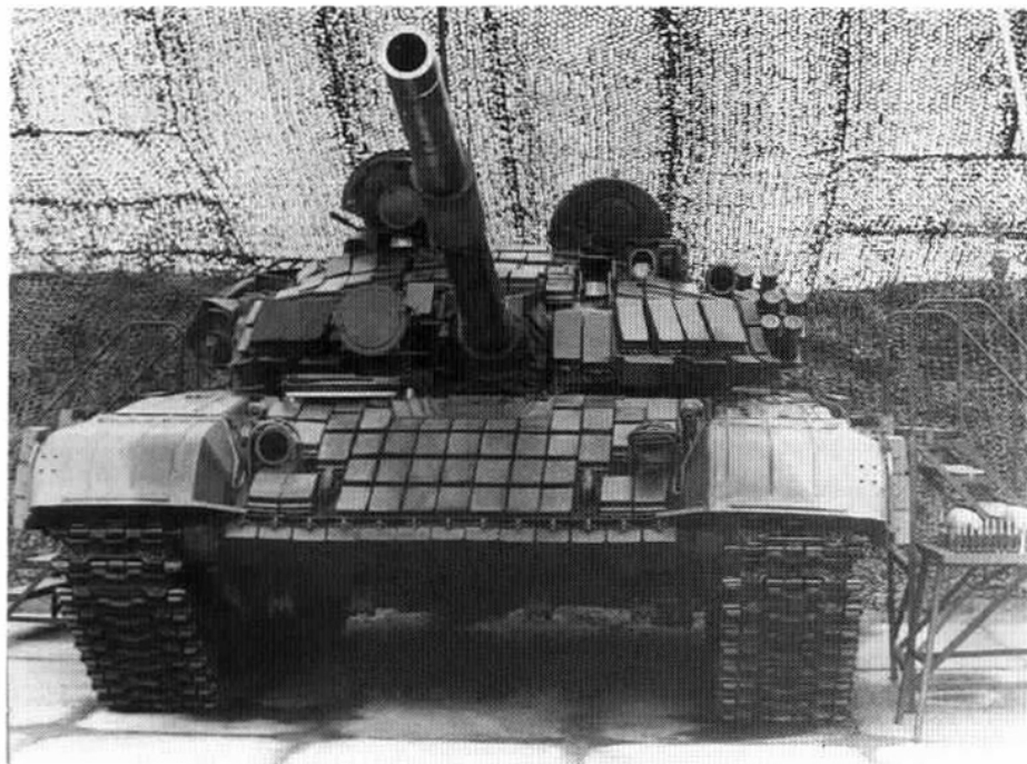
Many T-72B and T-72B1s were eventually retrofitted with EDZ reactive armour. Unlike the T-72As with EDZ, the T-72B uses only a single layer of bricks on the turret front. This is a T-72B, fitted with the 1K13 gunner's laser designator sight for use with the Svir guided anti-tank projectile. (US DoD)
