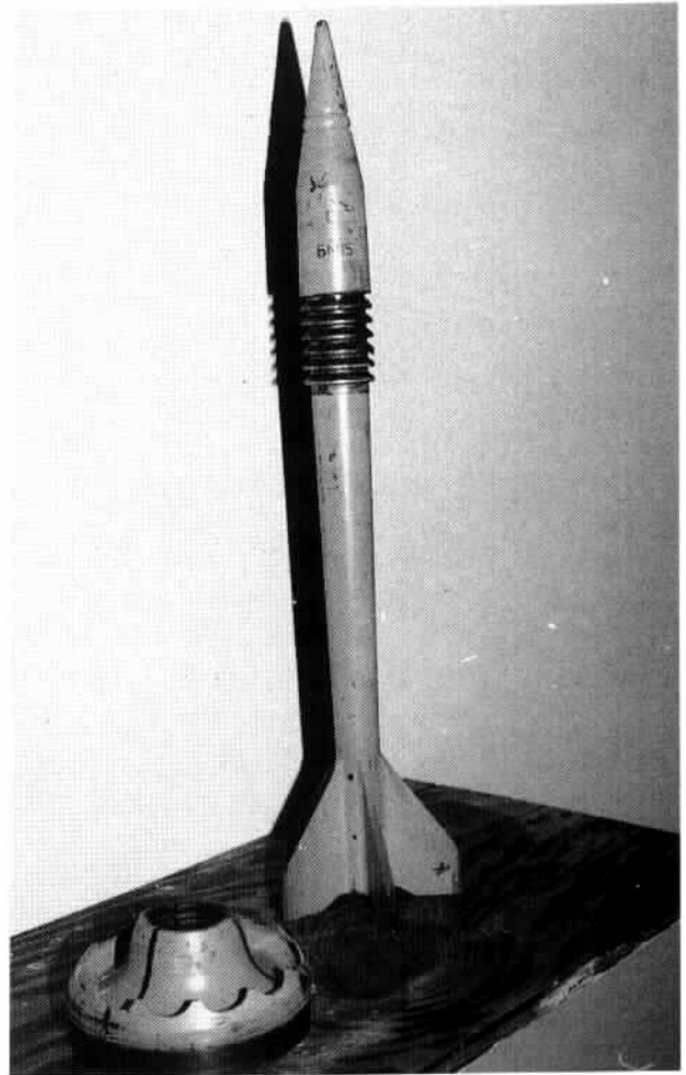
The sharp end of the T-72 is its APFSDS kinetic energy projectile. The example seen here is a BM15 steel projectile, part of the 3UBM7 round, the type used by Iraqi forces
