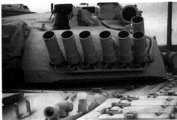
T-72M1s were fitted with the Soviet pattern 81 mm System 902A smoke mortars. The smoke mortars tend to
