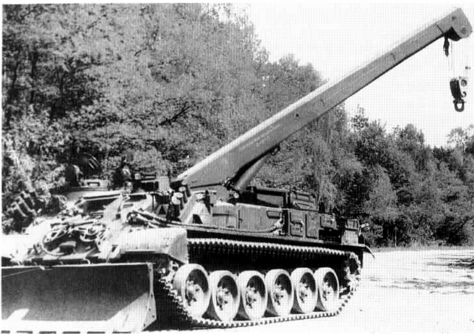
The WZT-3 is the Polish equivalent of the Russian BREM-1 armoured recovery and repair vehicle. It is very similar to the earlier WZT-2 which was based on the T-55 chassis.
