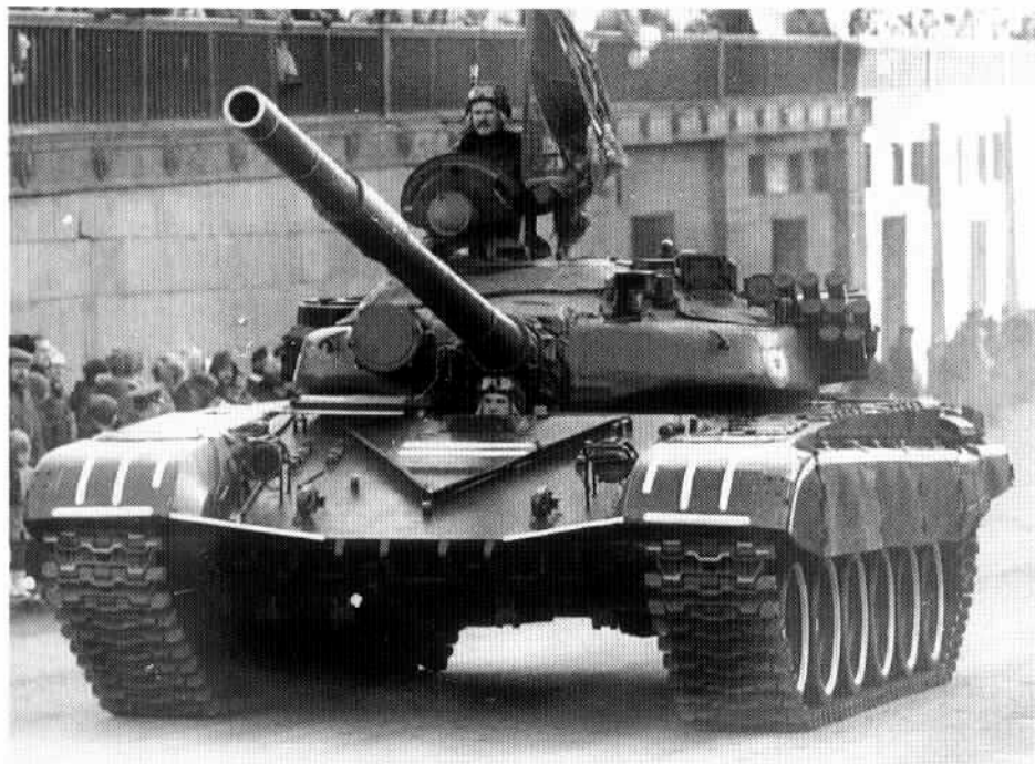
The T-72BI (Obiekt 174M) introduced yet another new turret design, sometimes called 'Super Dolly Parton' in NATO, or 'pot-belly' armour. The first batch of T-72BI had smoke mortars in the usual frontal positions, but the standard production types had them in clusters on the turret side to permit EDZ reactive armour to be fitted later.
