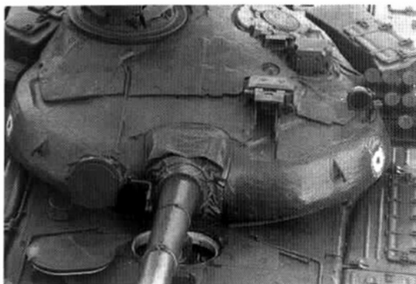
An overhead view of the T-72B1 with its thickened frontal armour. This armour had a distinctive
