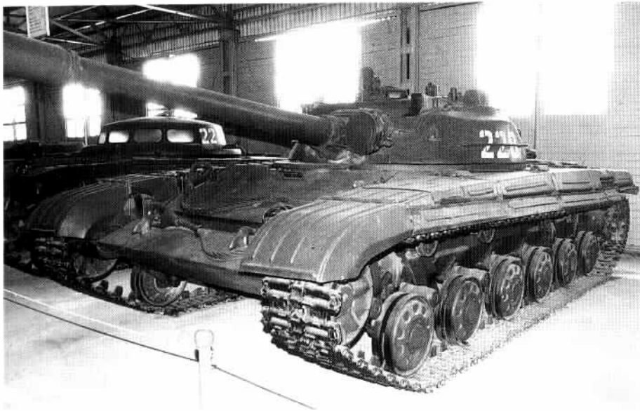
The first prototype of the T-72, the Obiekt 172, bore a close resemblance to the T-64 tank, incorporating many of its features such as its distinctive running gear. This was soon replaced by the running gear from the Obiekt 167 project. (Steven Zaloga)
