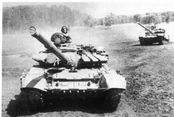
The new T-72 variant, the T-72BM, uses an advanced ERA similar to that first fitted to the T-80U and T-80UD tanks. Otherwise, it is similar to the T-72B tank.
