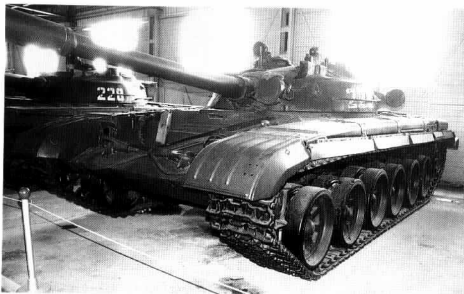
The definitive prototype of the Obiekt 172 shows many changes from the T-64, notably the large diameter roadwheels, new RSh single-pin track, and a new pattern of fuel panniers. A few hundred of these Obiekt 172 were produced for operational trials. (Steven Zaloga)
