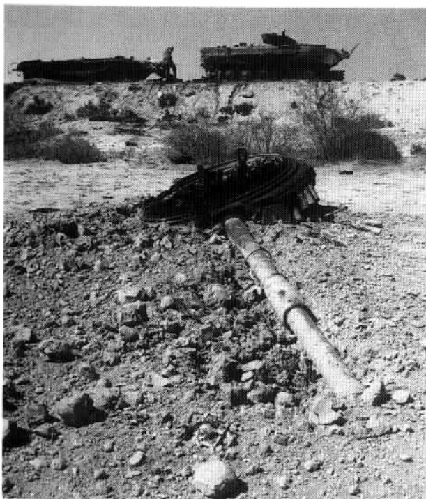
The vulnerability of the T-72 to catastrophic ammunition fire is all too evident in this view of an Iraqi T-72M1 knocked out by the 24th Infantry Division in the battle near
