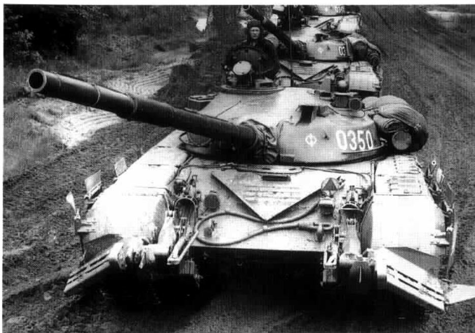
This Polish T-72M is fitted with the KMT-6M2 mine ploughs. Four Polish divisions are equipped with the T-72M and T-72M1: the 2nd, 5th, 11th and 12th Mechanised Divisions. The 1st Mechanised Division has a single regiment.
