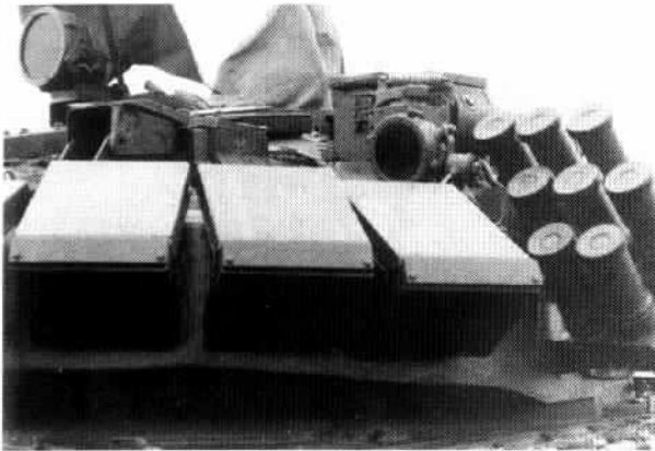
This close-up view of the T-72BM shows the new second-generation reactive armour. Above and behind
