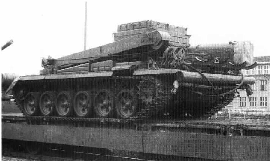
A rear view of a BREM-1 during rail transport near Jena, Germany in 1991. The BREM recovery vehicle has a large crane on the right side as seen here, with tool stowage contained in a platform on the vehicle roof. (Michael Jerchel)
