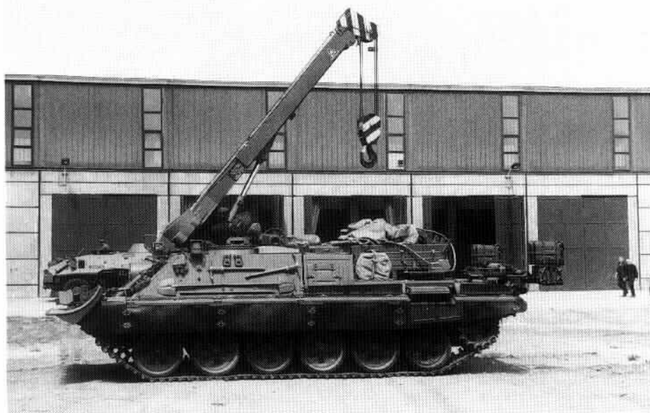
The VT-72, known in Germany as the T-72TK, was a joint German-Czechoslovak effort to develop a recovery vehicle on the T-72M1 chassis, similar in capabilities to the Soviet BREM-1 and Polish WZT-3. One of the German vehicles is seen here during trials at PW 2 in Grossenhain. (Michael Jerchel)
