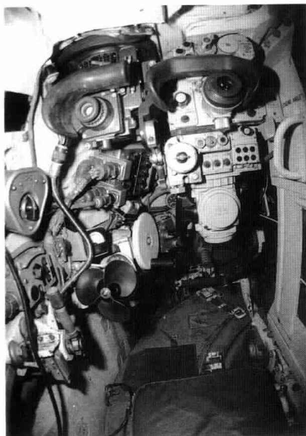
The gunner's station in the T-72M1 is cramped and very busy. The main TPD-K1 sight is on the right with its single monocular eyepiece, while to the left is the TPN-1-49 night sight.
