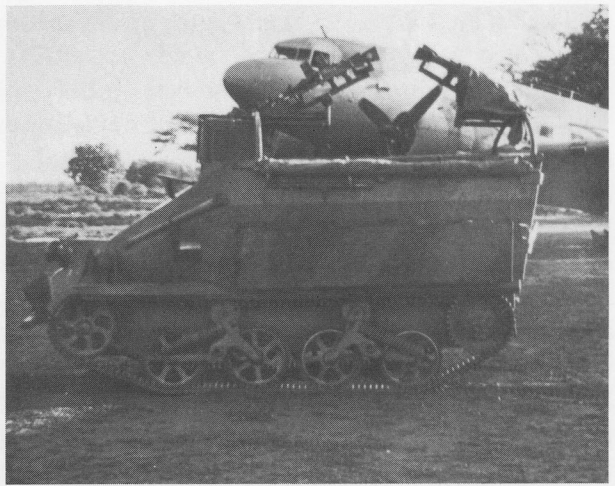
An extraordinary survival, of unknown origin! This Second World War vintage Universal Carrier, fitted locally with a tall armoured superstructure and two twin-MAG mountings, was used for convoy escort in rough terrain.
