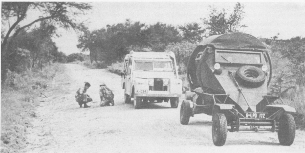
Land mines were a favourite guerrilla weapon, and Rhodesia's roads were highly vulnerable: many had no tarmac surface, and even the metalled stretches had soft shoulders. Note the roll-over bars fitted to the cab of the Police Land-Rover; and the Hippo, one of a number of special mine-protected vehicles devised and produced locally during the war.
