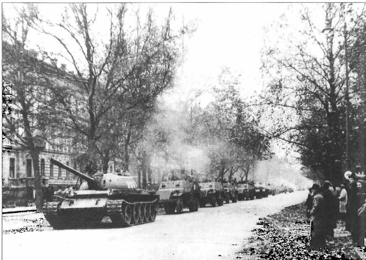
Watched somewhat incredulously by Hungarians, Soviet armour withdraws from Budapest following the ceasefire of 28 November. This shows a T-54 followed by BTR-152 armoured personnel carriers. (Hungarian Military Museum)
