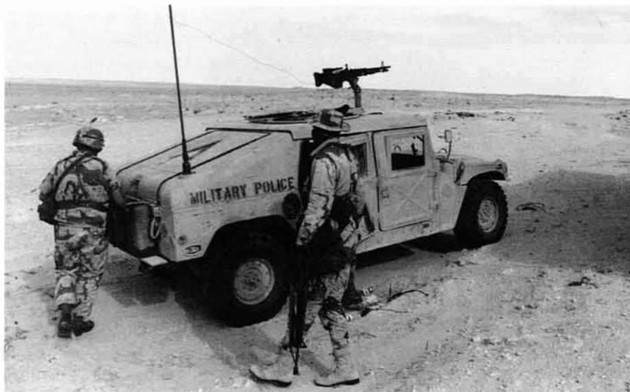
US M1026 HMMWV Military Police team halt to check the fastenings of their spare fuel cans. MP HMMWVs mount an M60 MG. The MP to the right wears the high top, Saudi-made suede boots. The black point-up chevron was painted on all coalition vehicles on the eve of the ground war in an effort to limit friendly fire casualties; it is not to be confused with similar subunit identification markings used by some US units. (Steve Capps)
