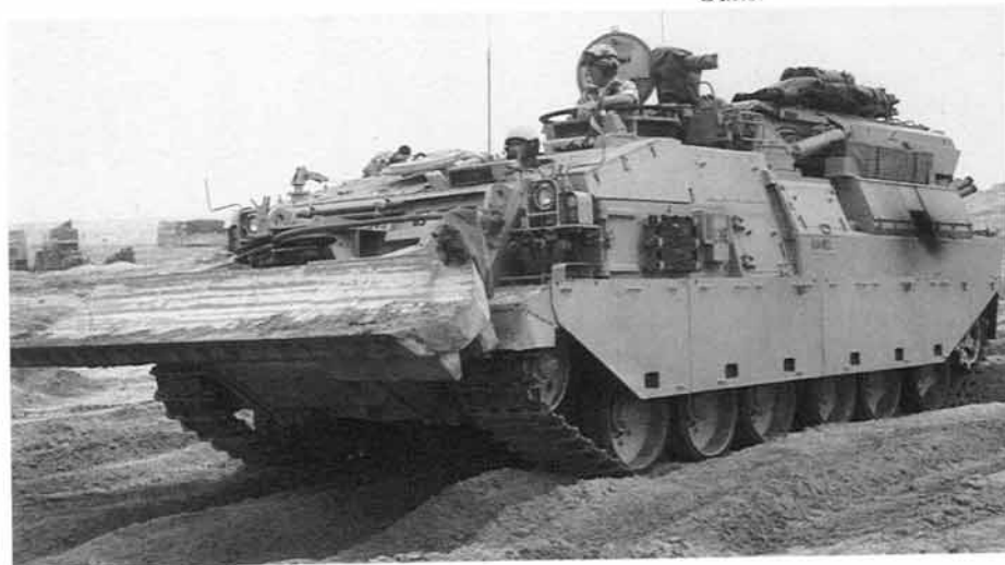
A British FV4204 Mk 1 armoured recovery vehicle. Based on the hull and chassis of the Chieftain Mk 5 tank, the ARV is issued to Royal Electrical and Mechanical Engineer recovery units. It mounts a dozer blade, two winches, and other recovery equipment. (Official)
