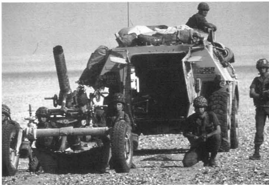
A French Marine Infantry 120mm MO-120-RT-61 rifled mortar crew pose at action stations behind their VTM mortar-towing vehicle, a variant of the VAB APC. (Official)
