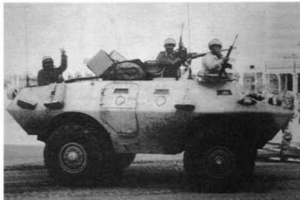
A V-150 Commando APC of the Saudi Arabian National Guard's King Abdul Aziz Bde. after the battle of Al-Khafji. This turrettless version mounts
