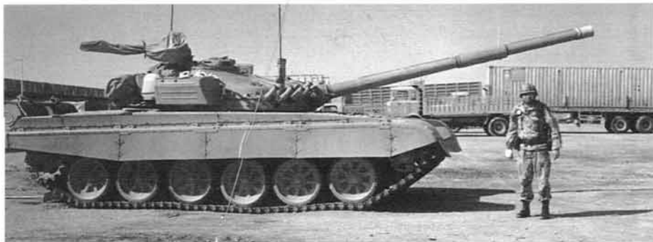
A Yugoslav-built M-84 tank delivered in Saudi Arabia for use by the Kuwaitis. The M-84, ordered prior to the Iraqi invasion, is an up-graded version of the Soviet T-72M. It mounts a 12.7mm DShK MG at the commander's hatch. Auxiliary fuel tanks are fitted on the rear deck. (Naydean Blair)
