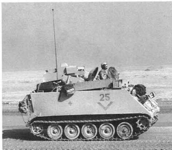
US M901 Improved TOW Vehicle (ITV); the dual-tube TOW turret, with integral sights, is retracted in the travel position. The three-man crew's OG duffle bags are strapped on
