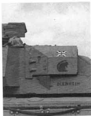
A close-up of a 4th (UK) Armd. Bde. Challenger's Thermal Observation and Gunnery Sight (TOGS) box displaying a full-colour national flag and this brigade's black desert rat (actually a jerboa) above a black vehicle name. The 7th Armd. Bde.'s similar insignia depicts a red jerboa with its tail curved beneath. (Steve Capps)
