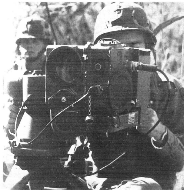
A tripod-mounted AN/TVQ-2 ground-vehicle laser locator-designator is aimed at a target to guide either a Hellfire missile or Copperhead 155mm projectile.
