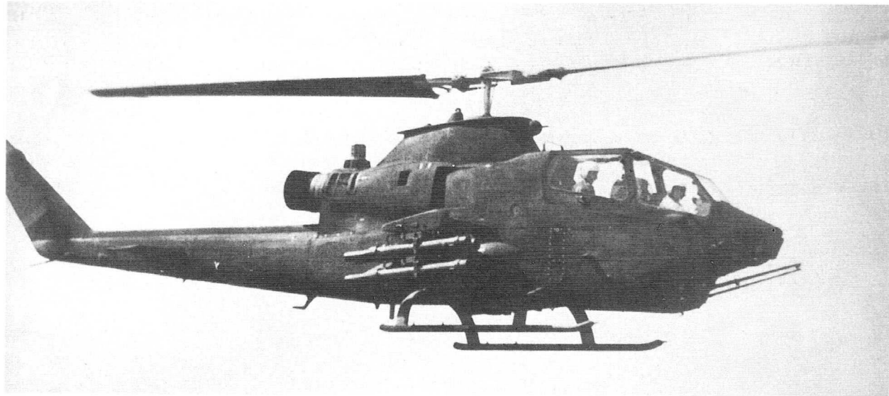
An AH-1S Cobra attack helicopter armed with eight TOW missiles and a 20mm gun.
