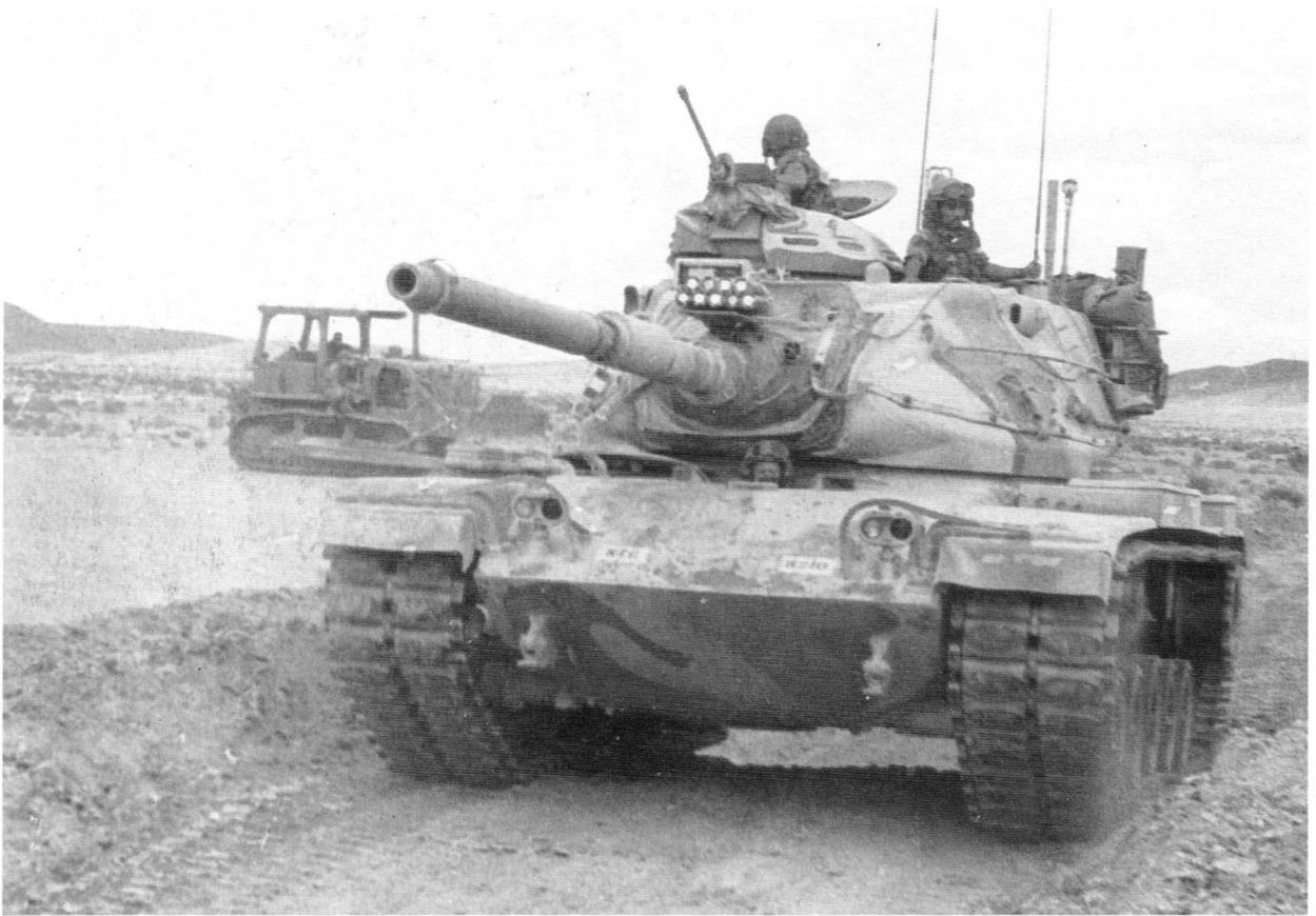
An M60A3TTS main battle tank at the National Training Center. The tubes above the 105mm gun are main gun firing simulators. A D7 dozer is in the background.
