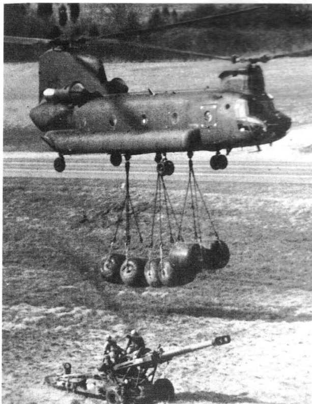
The improved CH-47D Chinook, with greatly increased lift and range, equips Assault Support and Medium Cargo Helicopter Battalions. This one sling-loads six 500 gal. fuel bladders. It can also lift the M198 155mm howitzer.
