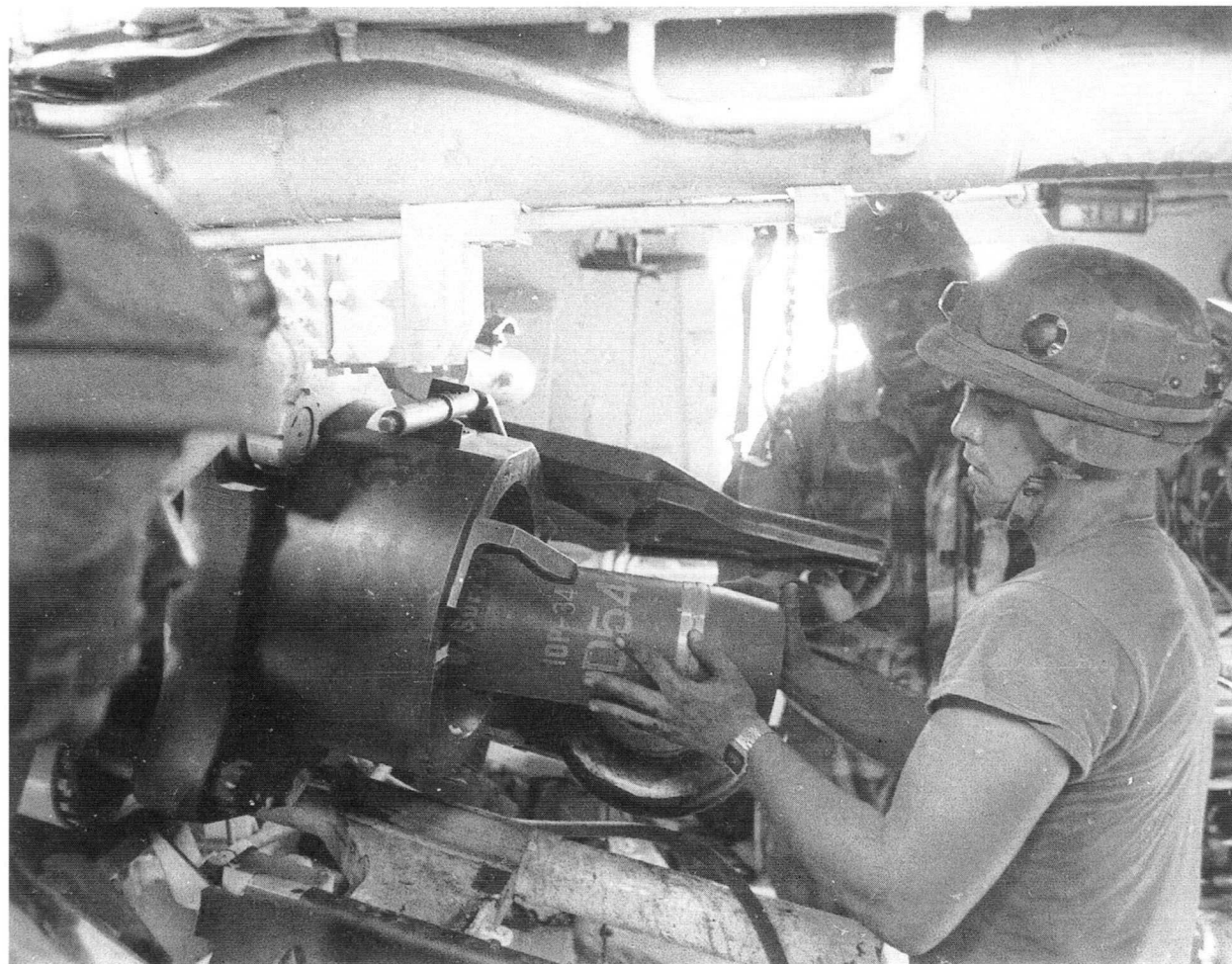
An M109A3 155mm howitzer crew loads an HE round. Note the MILES detector bands on their helmets.
