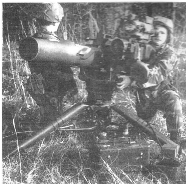
A ground-mounted M220A1 TOW missile system is prepared for firing. Mounted above its main tracker (sight) is an AN/TAS-4A thermal-imaging night sight.
