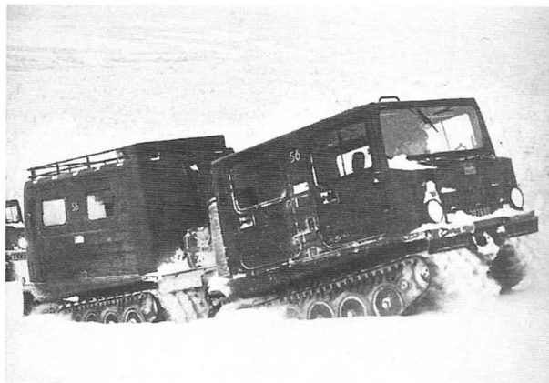
The Swedish-designed M973 small unit support vehicle was adopted by the Army in 1983 for use in far northern and arctic regions. The rear car is not a trailer, but a powered component of the vehicle.
