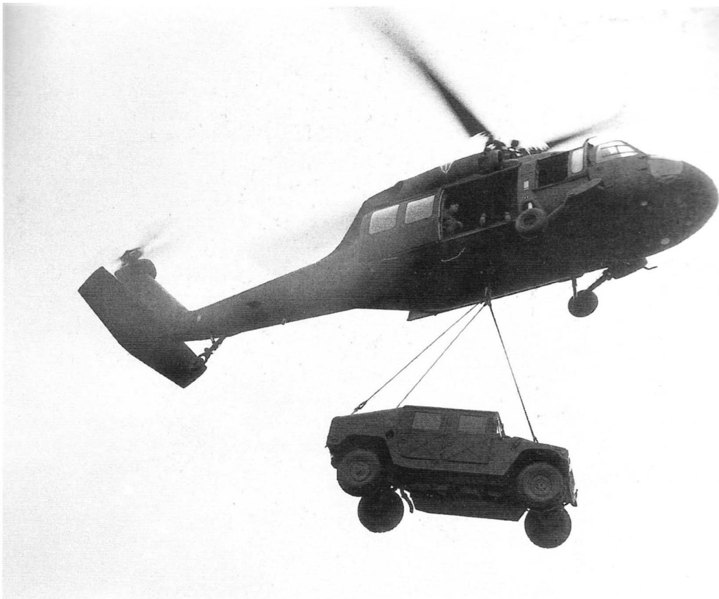
Further capabilities of the UH-60A are demonstrated as it sling-loads an HMMWV.
