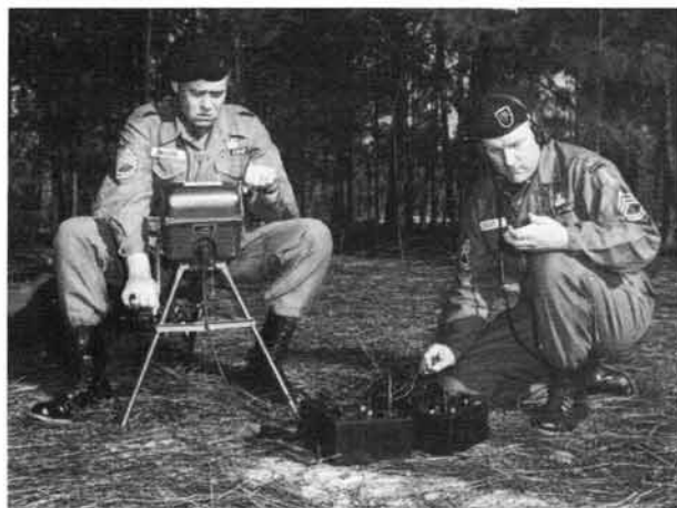
Radio operators of the 5th SFGA operate an AN/GRA-109 radio powered by a G-13 generator, Ft Bragg, 1962. They wear the M1953 field jacket. (US Army)
