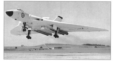
XH533 was the first production Vulcan B 2, and it is seen here undergoing acceptance trials at Boscombe Down
