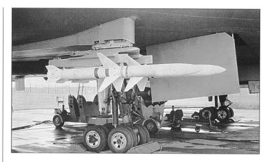
For 'Black Buck 6', XM597 carried four anti-radiation Texas Instruments AGM-45A Shrike missiles split two per underwing pylon. This weapon was considerably lighter than the AS37 Martel that had first been trialled with the B 2, and it also created fewer integration problems (via Phil Jarrett)
