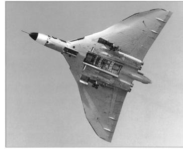
This underside view of a Vulcan B 2 clearly shows the cavernous dimensions of the aircraft's bomb-bay. Also clearly visible is the visual bomb-aiming position forward of the nosewheel leg
