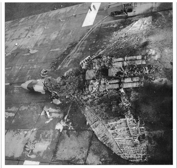
The bitter end. The charred remains of XL385 of No 617 Sqn at Scampton after an explosion in the port engines on start-up on 6 April 1967. The crew got out safely
