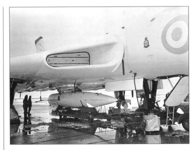
A Blue Steel missile is carefully loaded into the modified bomb-bay of a No 617 Sqn Vulcan B 2
