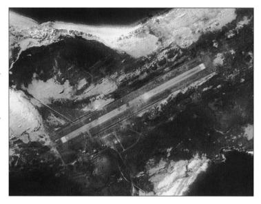
This post-attack photograph taken from a Sea Harrier shows Stanley runway after 'Black Buck 1'. The line of bomb craters is clearly visible, the first bomb from the stick holing the centre of the runway
