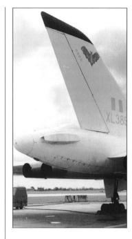
A close-up of the new Vulcan B 2 tail cone as fitted to XL385 (whose tail features a No 9 Sqn bat insignia). The tail cone was full of ECM 'cans', and the scoop was for cooling air to keep all these systems operable
