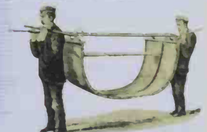
The Lady Alice Stanley had a boat specially made for his expedition to Africa in 1874. It was built in sections so that it could be carried around rapids and other dangerous stretches of the Congo River. He called it the Lady Alice , after his fiancée (who married another man while he was in Africa). The river proved so difficult to follow, and so many of Stanley's men drowned, that he had to complete the journey on foot, leaving the Lady Alice to rot above Livingstone Falls.
