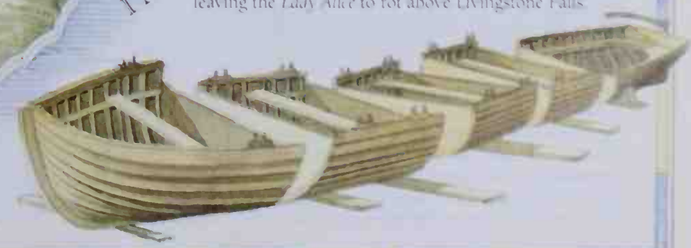
The Lady Alice Stanley had a boat specially made for his expedition to Africa in 1874. It was built in sections so that it could be carried around rapids and other dangerous stretches of the Congo River. He called it the Lady Alice , after his fiancée (who married another man while he was in Africa). The river proved so difficult to follow, and so many of Stanley's men drowned, that he had to complete the journey on foot, leaving the Lady Alice to rot above Livingstone Falls.
