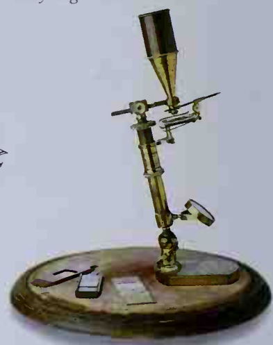
Darwin's microscope This neat little microscope was used by Darwin during his voyage on the Beagle . It was designed to be folded away when not in use.
