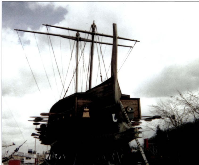
Olympias in dry-dock, showing the three banks of oars from which the name trireme is derived. The trireme was the standard warship of the ancient Mediterranean.
