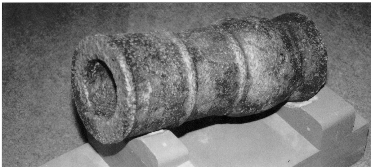
ABOVE Early Chinese cannon were simple cast iron bombards as in this example shown here, which has a calibre of 4.15 inches, and an overall length of 18.7 inches. Note the bulbous shape around the touch-hole to add strength. It was made during the fourteenth century. (Royal Artillery Museum, Woolwich)
