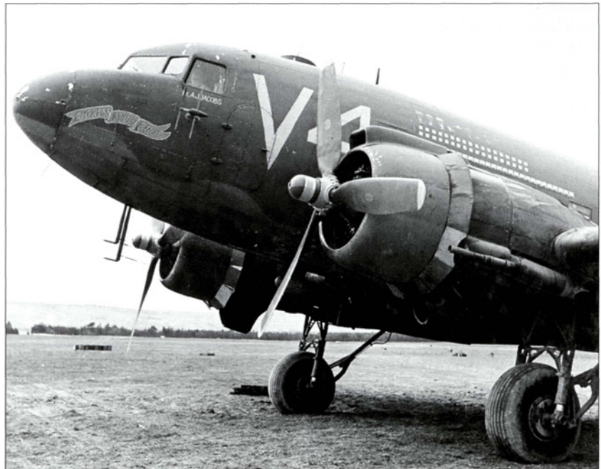
The workhorse of the troop carrier units was the Douglas C-47 Skytrain. The antenna below the cockpit window is for the Rebecca homing system used for navigation to the drop zone. "Empress Mary Ellen" served with the 304th Troop Carrier Squadron, 442nd TCG, 50th TCW, and is seen here at Vertus, France, on February 26, 1945, with an ample array of paratroop, glider and supply missions marked on the side of the fuselage. (MHI)
