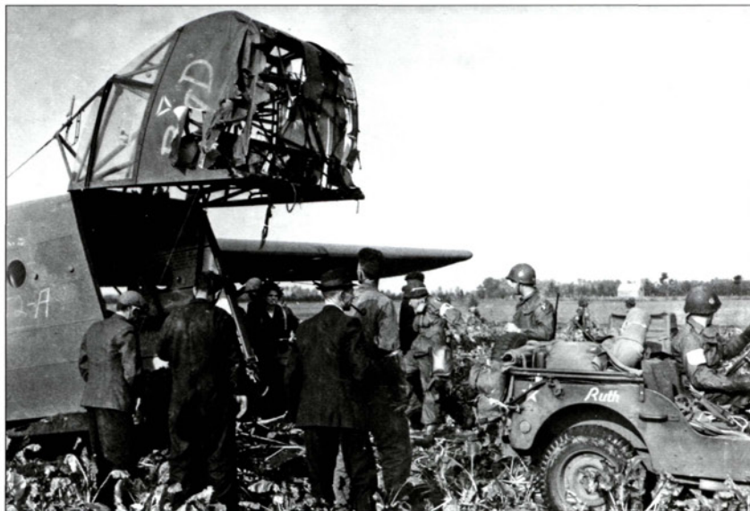
This CG-4A from Serial A-47 of the 434th Troop Carrier Group has lost much of the fabric from its nose after having landed at Landing Zone W during Operation Market. The CG-4A had a special mechanism for quickly opening the nose to disembark its jeep cargo. (NARA)
