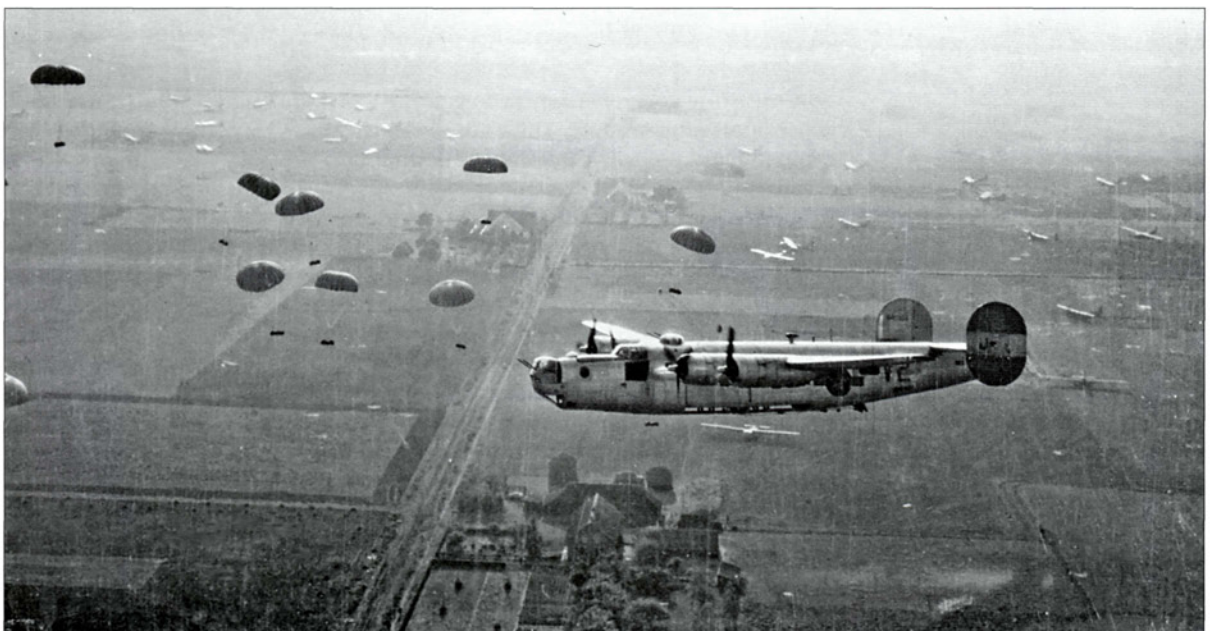
The B-24 Liberator bomber was used on several occasions to supplement transport aircraft for dropping supplies during airborne operations as is seen here in September 1944 during Operation Market. This required the bottom ball-turret to be removed to create a suitable opening for the para-pack drop. (Patton Museum)
