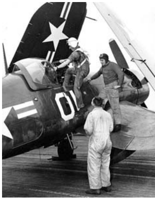
Left: This F4U-5P “Corsair” aerial reconnaissance plane was equipped with radar and aerial surveillance equipment (there is a camera hatch below the cockpit). It was a variant on the F4U-5. The F4U-1P was equipped for photo-reconnaissance. This image was taken around the summer of 1950. The earlier F4U was one of the first aircraft to be equipped with interception radar , in the summer of 1941. Right: The USS Valley Forge transporting aircraft in April 1949. Some of the aft planes are F4Us. [U.S. Navy All Hands and Historical Center Collection historical archives photos, public domain.]
