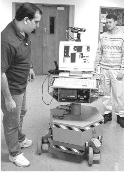
Left: Purdue Doctoral students DeSouza and Jones work with “Peter” a mobile robot equipped with a number of types of sensors. Peter can navigate by converting images to 3D measurement grids and comparing the surroundings with a pre-programmed destination. The robot has cameras and ultrasonic detectors to enable it to carry out its tasks. Right: ROBERT III, evolved from Bart Everett’s original Robart I, was developed in 1992 as part of the U.S. Naval Mobile Detection, Assessment, and Response System (MDARS) program. [Purdue 2000 news photo; U.S. Space and Naval Warfare Systems Center news photo, released.]
