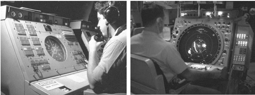
Different types of radar console stations in the combat information center (left) and the combat direction center (right) of the aircraft carrier USS Kitty Hawk (CV-63). [U.S. DoD 1987 and 1991 news photos by James R. Gallagher, released.]
