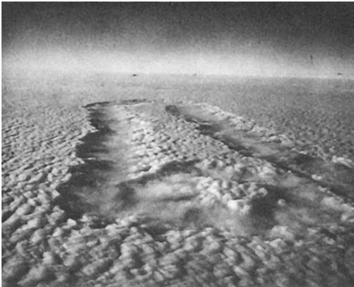
Figure 1.2 Race track pattern approximately 20 miles long produced by dropping crushed dry ice from an airplane. The safety-pin-like loop at the near end of the pattern resulted when the dry ice dispenser was inadvertently left running as the airplane began climbing to attain altitude from which to photograph results. From Havens et al. (1978). Photo courtesy of Dr. Vincent Schaefer.
