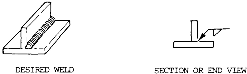
Figure 3-9. Arrow side fillet welding symbol.
