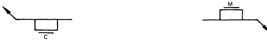
Figure 3-36. Surface contour of plug welds and slot welds with user's standard finish symbol.
