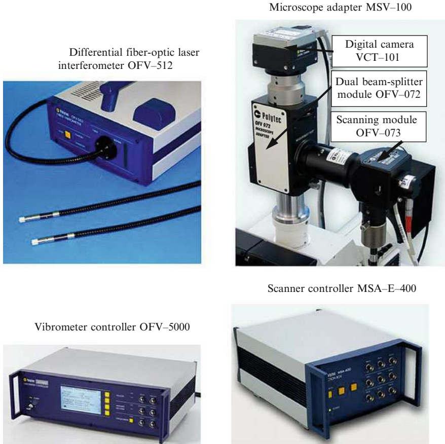
Fig. 5.28 Components of Polytec laser Doppler vibrometry system MSV-400
